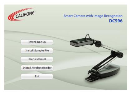
If the computer does not show the above screen, the software can also be installed manually: Insert Installation CD → Install DC596 Program File → Connect DC596 to the Computer → Finish
