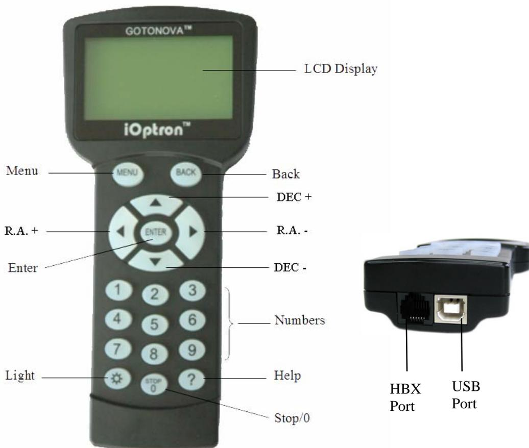
**Figure 19. GoToNova 8406 hand controller**
