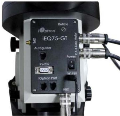
Figure 6. Ports on iEQ75-GT™ control box
