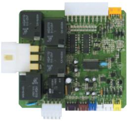
Auto Page remote start circuit boards maintain 30/45-ampere relays for reliable and long-lasting remote start performance.
