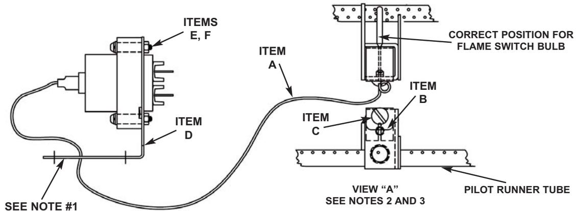
1.) Remove old flame switch and bracket located inside control panel. (Retain hardware). Assemble flame switch item A to bracket item D with items E and F. Slide bulb end of flame switch through center hold in item D flame switch bracket and through hole located in control panel. If needed, use a letter "n" drill to open hole. Reassemble to control panel with retained hardware.
