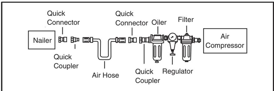
**Figure 2.** Filter/Lubricator/Regulator Unit.
