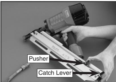
**Figure 3.** Sliding pusher toward the catch lever.
