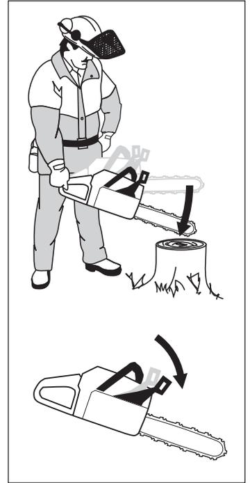
When the bar hits the stump the brake should be applied.
