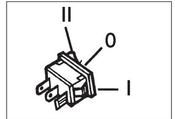
The switch is off in position "0" supplies current to the handle heater in position "I" supplies current to the carburettor in position "II"
