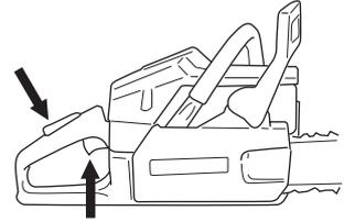
CAUTION! Do not release the starter handle from fully pulled out position as this can cause damage on the saw.
