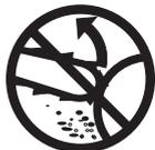
Contact of the guide bar tip with any object should be avoided. Please see pages 12-21 in your "Chain saw operator's safety manual".
