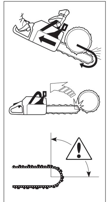
In this case the saw pulls itself towards the tree and the front edge of the saw provides a natural rest when cutting. Cutting on the pull stroke gives you better control over the saw and the position of the kickback zone.
