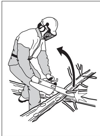
4 Never use the saw above shoulder height and try not to cut with the tip of the bar.
