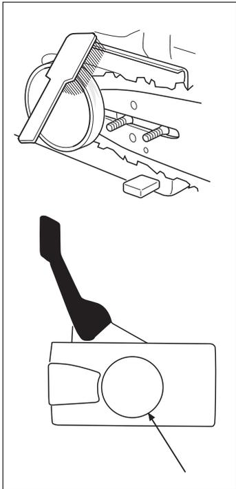
Regularly check that the brake band is at least 0.6 mm thick at its thinnest point.
