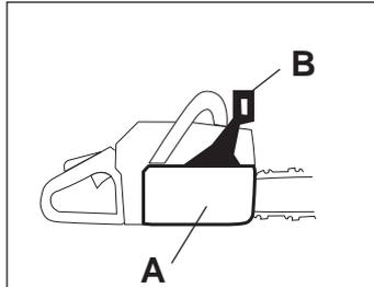
The brake is applied when the front hand guard (B) is pushed forwards.
