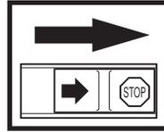
Switch off the engine by moving the stop switch to the STOP position before carrying out any checks or maintenance.
