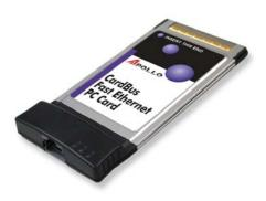
The FE2000SX, 32-bit CardBus 10/100Mbps Fast Ethernet PC Card,
