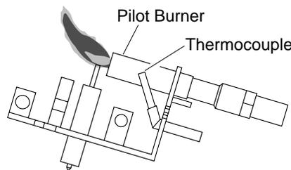
Figure 24 - Incorrect Pilot Flame Pattern
