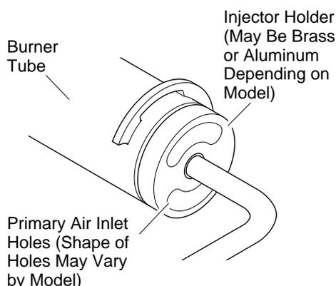
**Figure 25 - Injector Holder On Outlet Burner Tube**
