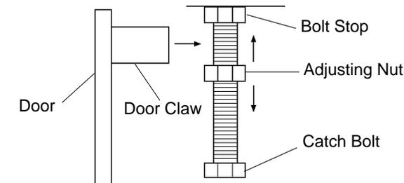
**Figure 12 - Catch Bolt and Door Claw Orientation**
