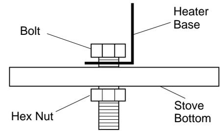
**Figure 14 - Fastening Heater Base to Stove Drop Bottom**
