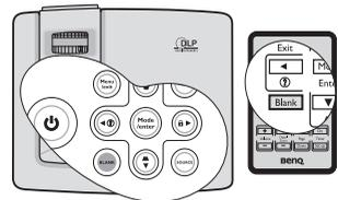
You can set the blank time in the **SYSTEM SETUP: Basic > Blank Timer** menu to let the projector return the image automatically after a period of time when there is no action taken on the blank screen. The length of time can be set from 5 to 30 minutes in 5-minute increments.
