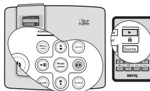
To release panel key lock, press and hold **▶/🔒** on the remote control or projector for 3 seconds.
