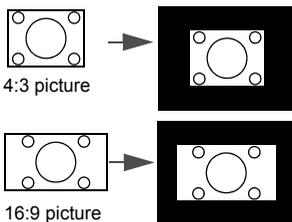
3. **4:3:** Scales an image so that it is displayed in the center of the screen with a 4:3 aspect ratio. This is most suitable for 4:3 images like computer monitors, standard definition TV and 4:3 aspect DVD movies, as it displays them without aspect alteration.
