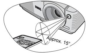
Make sure that there are no obstacles between the remote control and the IR sensor on the projector that might obstruct the infra-red beam.
