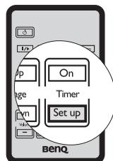
1. Press **Timer Set up** on the remote control or go to the **SYSTEM SETUP: Basic > Presentation Timer** menu and press **Mode/Enter** to display the **Presentation Timer** page.
