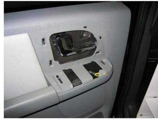
Remove window/lock switch assembly from door
