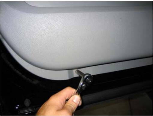
Remove hex head screws holding lower section of door panel
