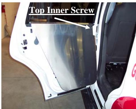
Center door panels so edges do not hang over. Attach to door with #10 x 1/2" stainless sheet metal screws.
