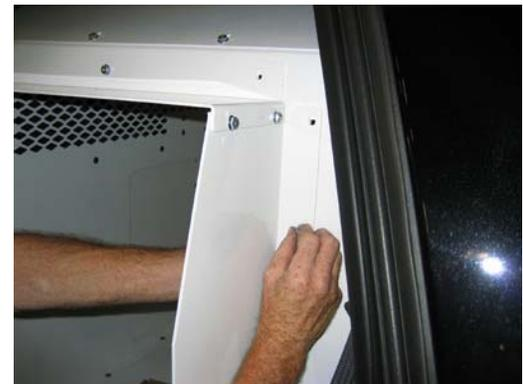
Attach tunnel to K9 assembly using 1/4" x 3/4" and 1/4" x 1/2" carriage bolts and serrated nuts
