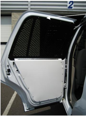
Hinge up window guard and reattach to bracket with 10-32 x 1/2" Stainless machine screws and #10 Flat washers.
