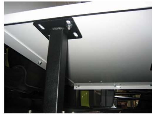
Attach assembly to K9 floor using 1/4" x 3/4" carriage bolts and serrated nuts
