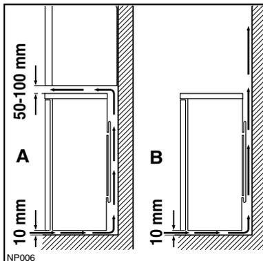
Do not obstruct the space underneath. The back of the cabinet may be placed close to the wall but must not touch it. DO NOT install in places with restricted ventilation.
