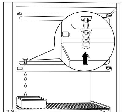
4. when defrosting is completed, dry the interior thoroughly and refit the plug.
