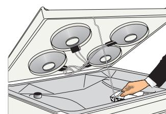
When lowering the lift-up range top, grasp the sides with fingertips only. Be careful not to pinch fingers. **DO NOT** drop or bend the range top when raising or lowering. This could damage the surface.
