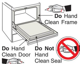
To clean oven door, wash with hot, soapy water and a clean cloth. **DO NOT** immerse the door in water.
