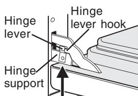
Lock engaged for door removal - Figure 1
