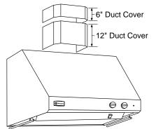
Decorative duct covers are available in 6" and 12" heights. Duct covers may be stacked, in various combinations, to conceal the ductwork running from the top of the hood to the ceiling.
