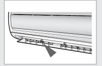
You can adjust the airflow direction horizontally with your hands. The inner blades with small fins moves the air to the required direction.
