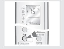
You can adjust the airflow direction vertically. The outer airflow blade moves up and down to increase the efficiency of the cooling or heating operation.
