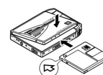
+ Press the center of the MD until the disc is locked into place.
