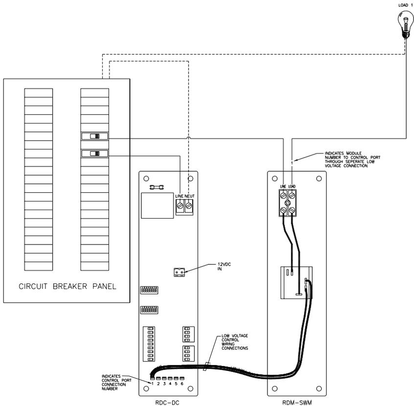
**FIG. 3** RDM-SWM Switch Module 2400 line wiring configuration
