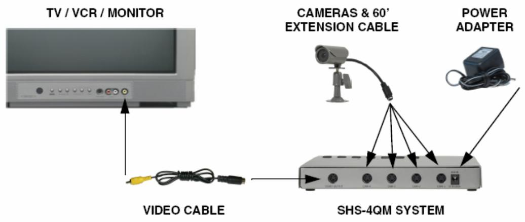
**Scenario #3:** Connect the 4 Cameras to the Switcher, and connect the switcher to the System. Repeat for the second switcher. Purchase additional Cameras for the other open Ports on the System.
