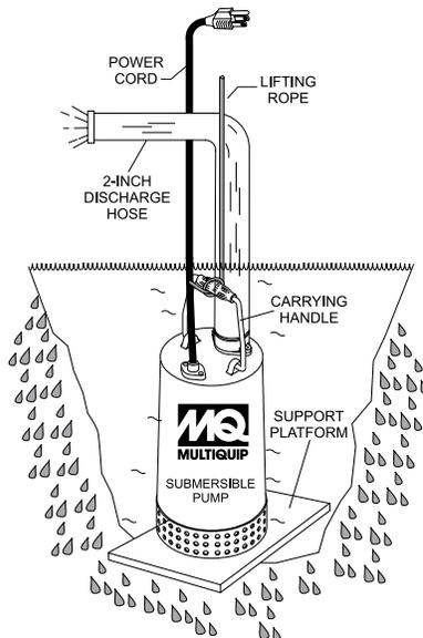
**Figure 9. Submersible Pump Upright
