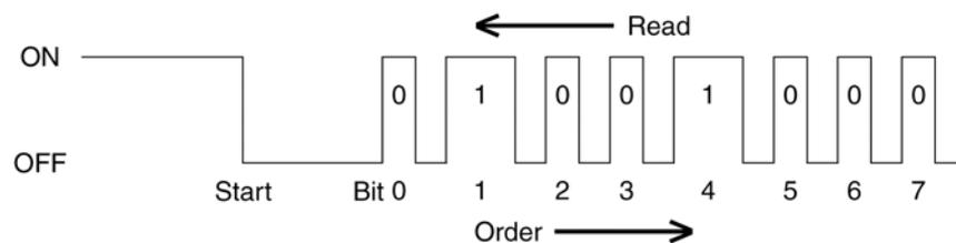
Check 1 Convert the DC IN LED blink pattern into the hexadecimal error code and compare it to the tables below.
