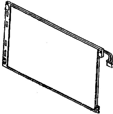
*Figure 1-9 LCD module*
