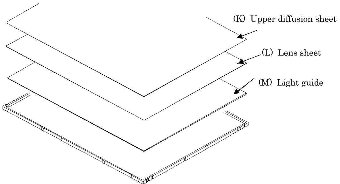
Figure 4-74 Replacing Sharp fluorescent lamp (XGA) (8)
