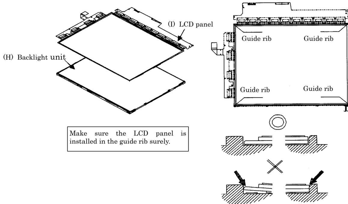
Figure 4-129 Replacing Sharp fluorescent lamp (SXGA+) (17)
