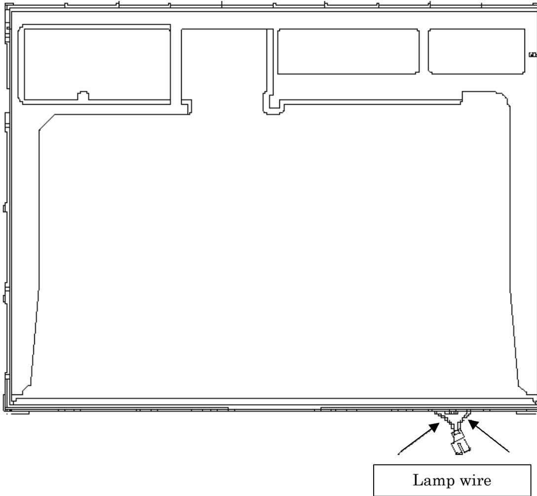
Figure 4-111 Replacing Samsung fluorescent lamp (SXGA+) (8)
