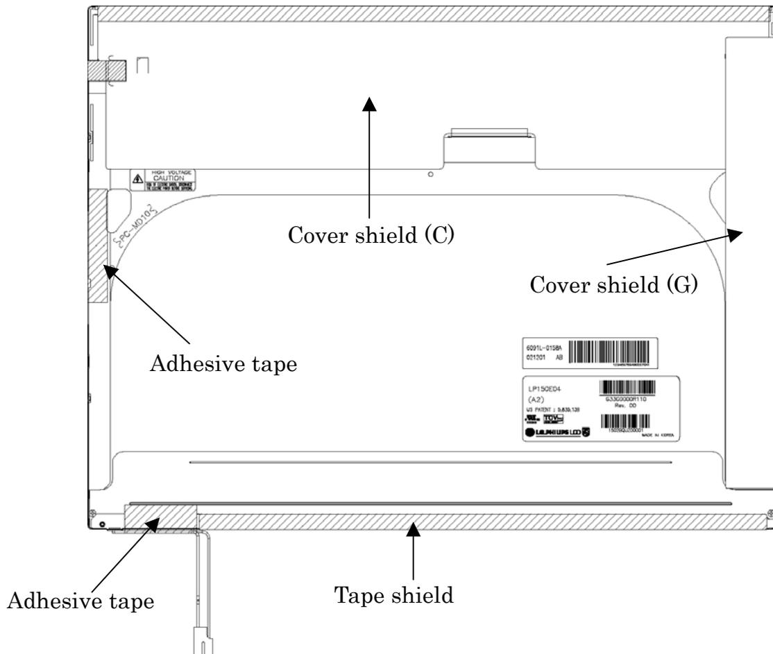
Figure 4-96 Replacing LG.Philips fluorescent lamp (SXGA+) (1)
