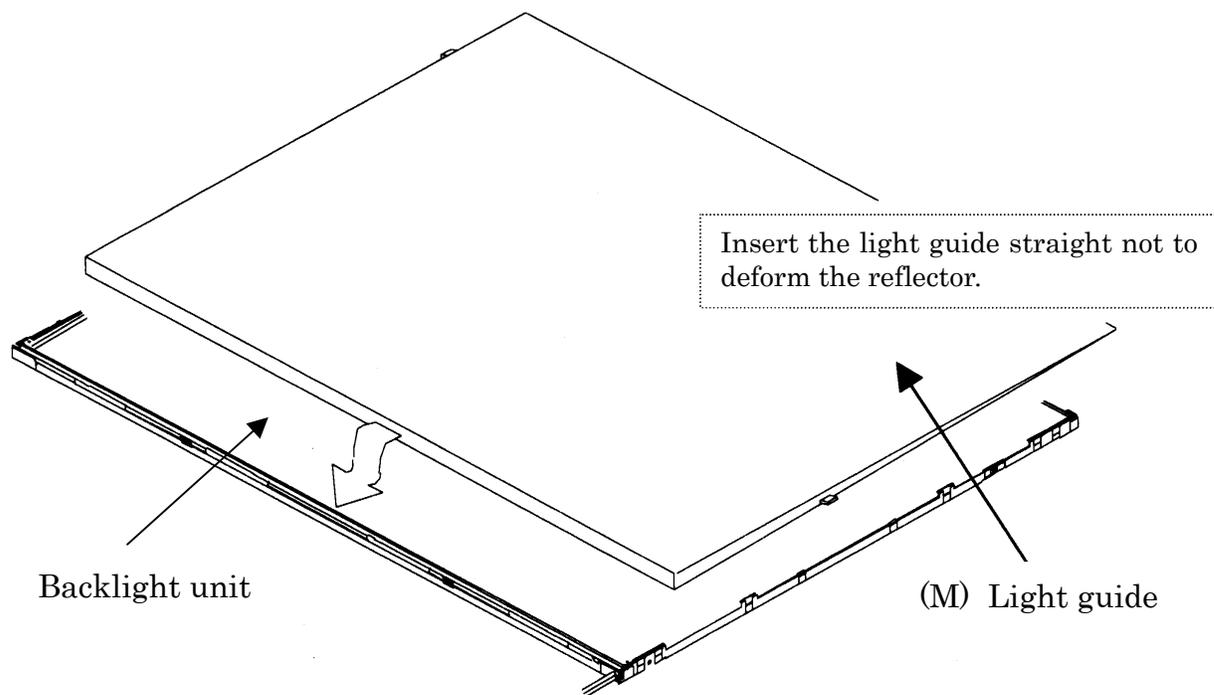
Figure 4-81 Replacing Sharp fluorescent lamp (XGA) (15)
