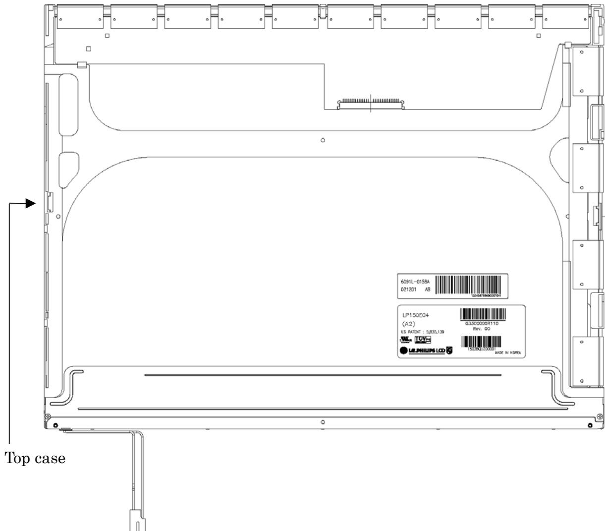
Figure 4-102 Replacing LG.Philips fluorescent lamp (SXGA+) (7)
