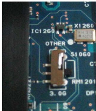
2. When a CPU other than 3.06GHz (2.53, 2.66, 2.80GHz) is used:
