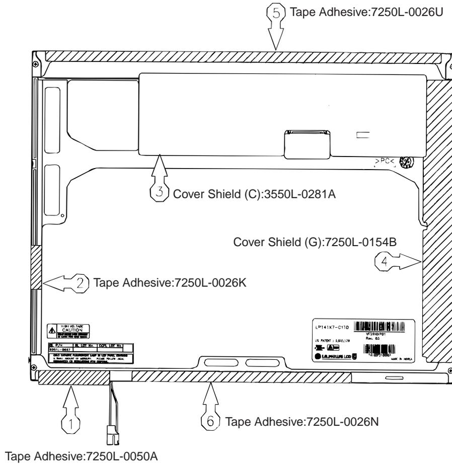
Figure 4-175 Attaching the outside tape and cover shield
