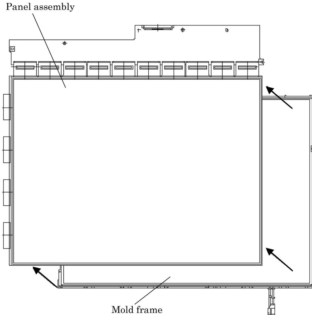
Figure 4-108 Replacing Samsung fluorescent lamp (SXGA+) (5)
