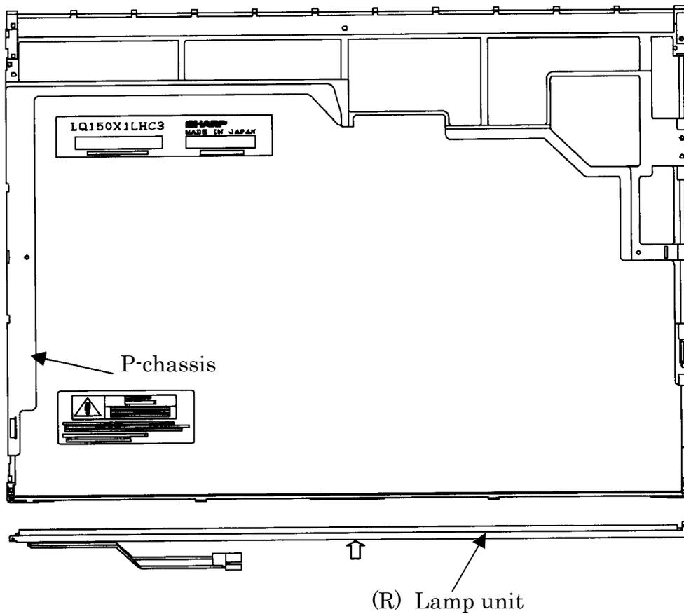
Figure 4-78 Replacing Sharp fluorescent lamp (XGA) (12)
