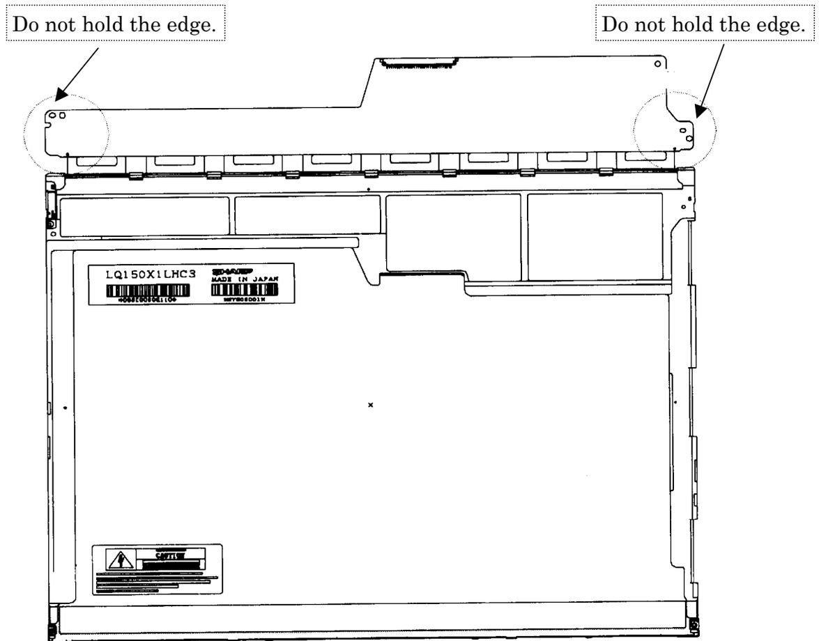
Figure 4-84 Replacing Sharp fluorescent lamp (XGA) (18)
