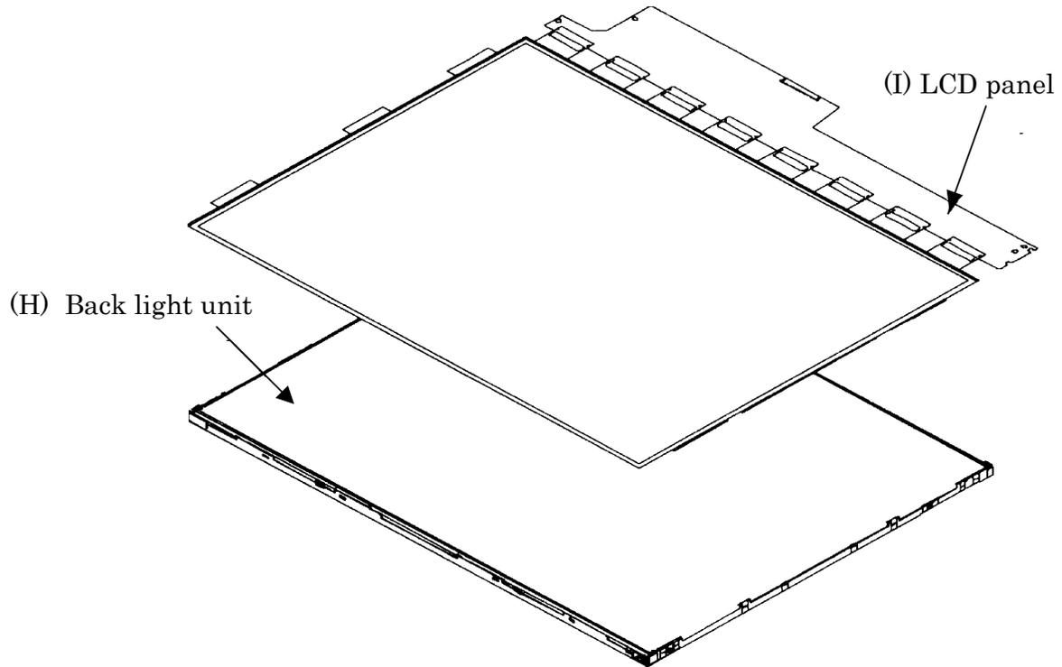
Figure 4-72 Replacing Sharp fluorescent lamp (XGA) (6)
