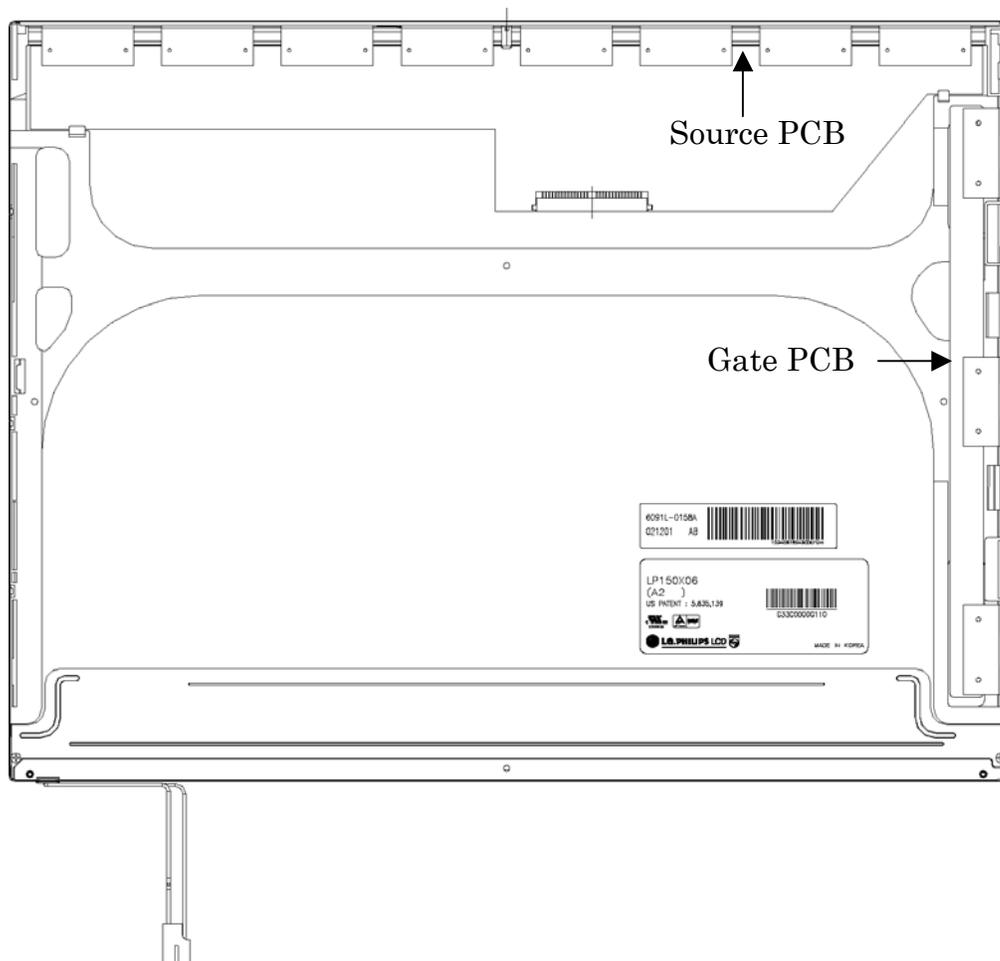
Figure 4-52 Replacing LG.Philips fluorescent lamp (XGA) (3)
