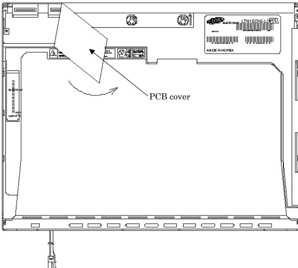
Figure 4-58 Replacing Samsung fluorescent lamp (XGA) (1)
