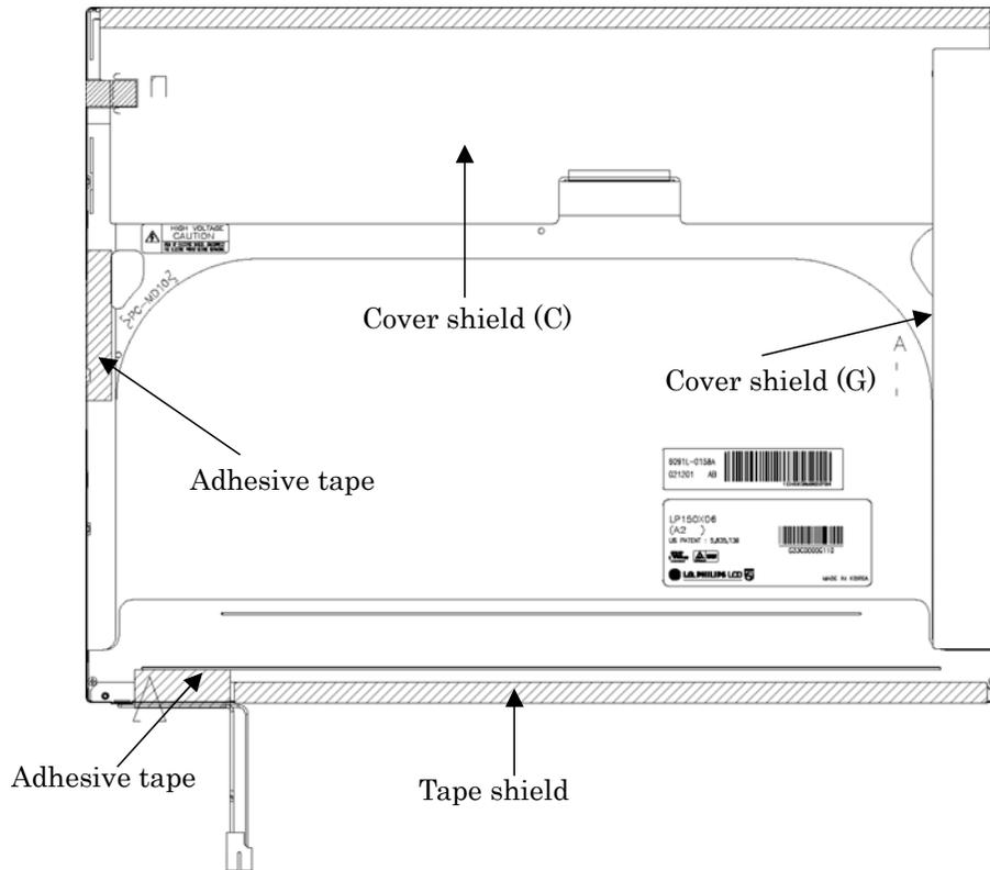
Figure 4-57 Replacing LG.Philips fluorescent lamp (XGA) (8)
