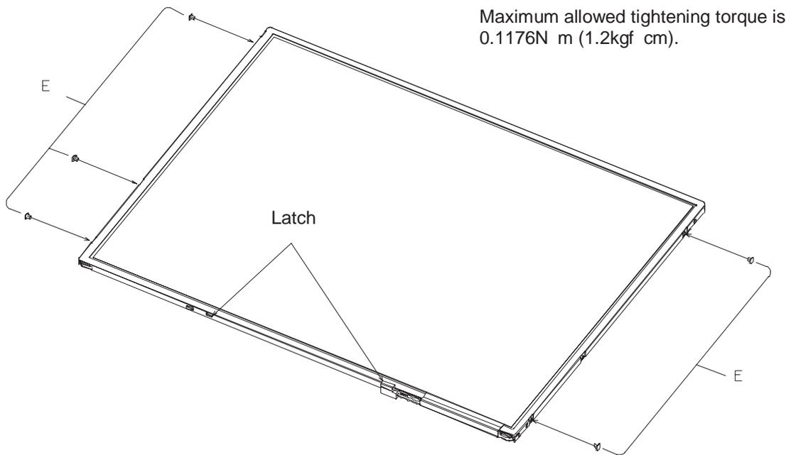
Figure 4-157 Fastening the screws on both sides
