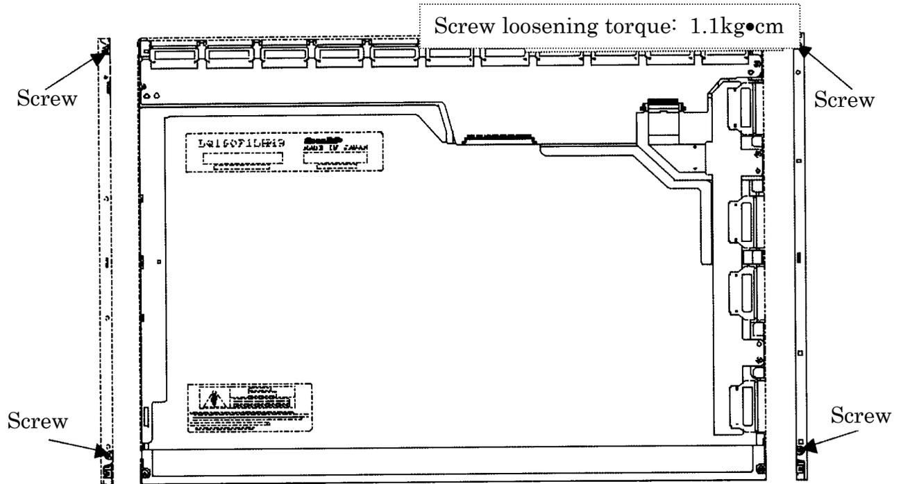
Figure 4-114 Replacing Sharp fluorescent lamp (SXGA+) (2)
