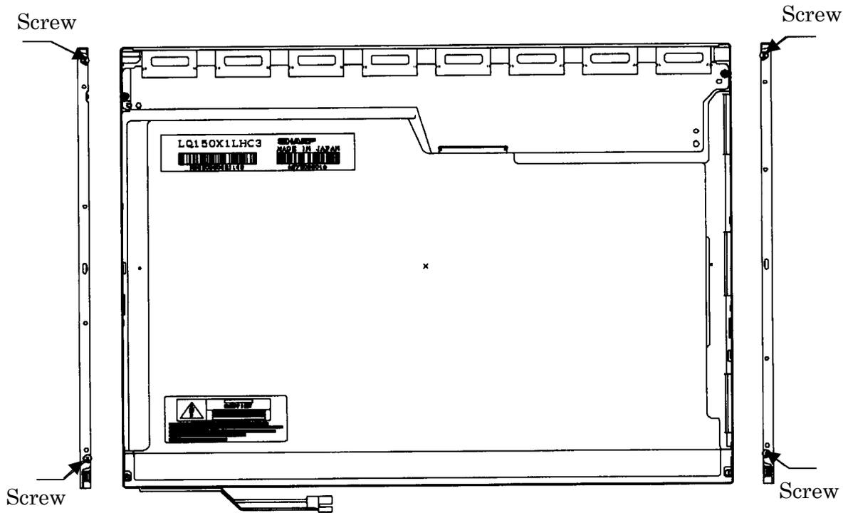
Figure 4-88 Replacing Sharp fluorescent lamp (XGA) (22)
