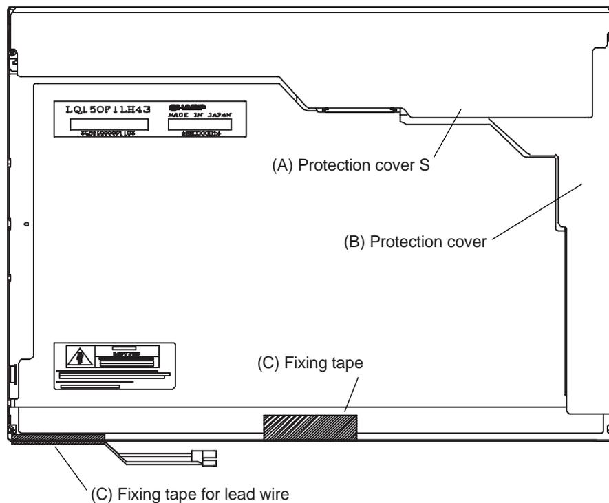
Figure 4-113 Replacing Sharp fluorescent lamp (SXGA+) (1)
