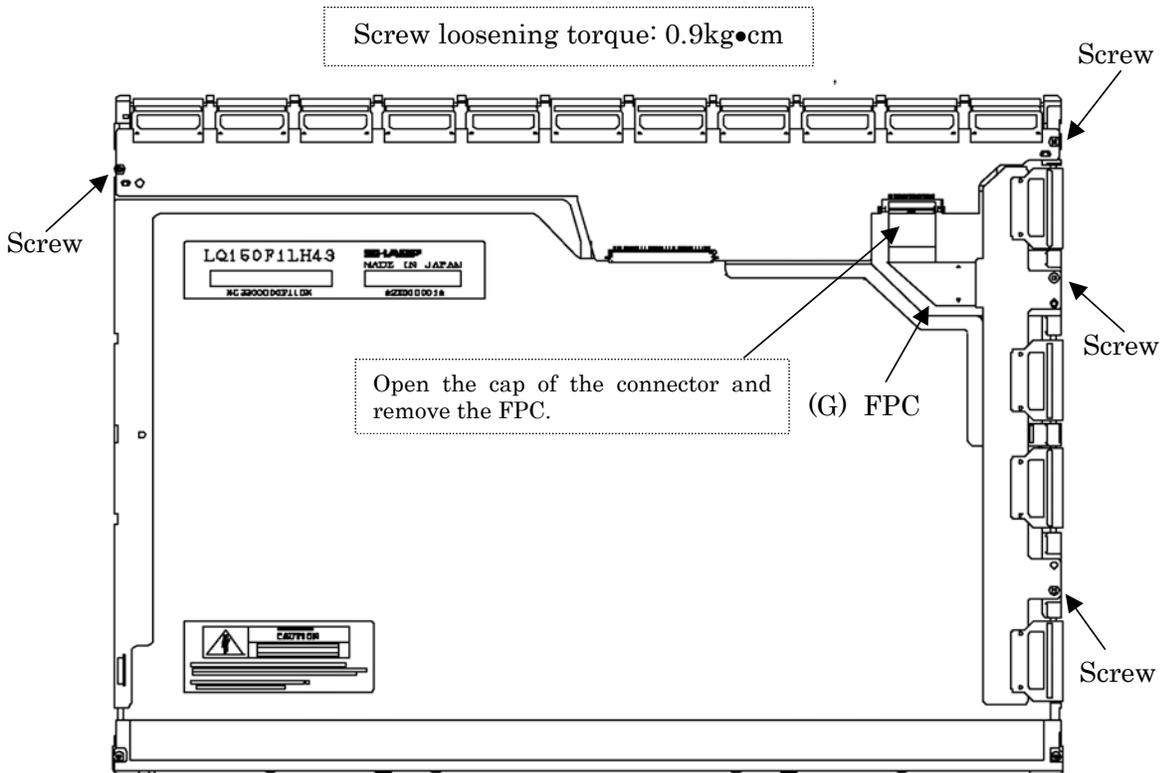
Figure 4-116 Replacing Sharp fluorescent lamp (SXGA+) (4)
