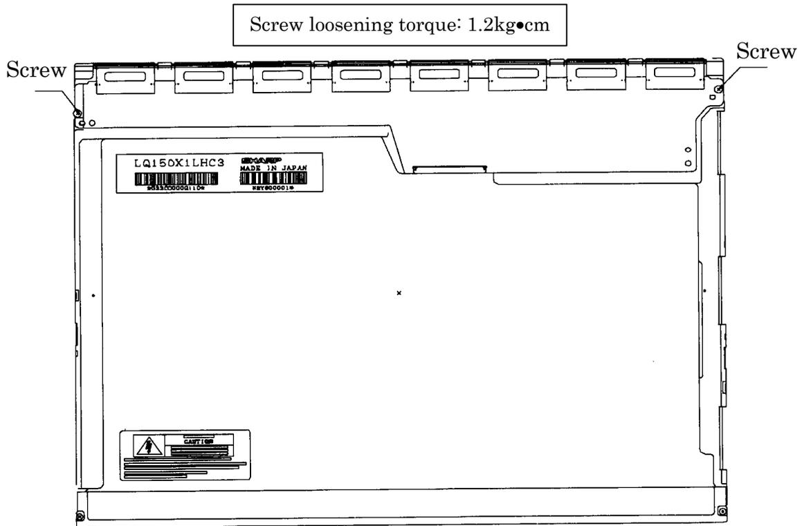
Figure 4-70 Replacing Sharp fluorescent lamp (XGA) (4)
