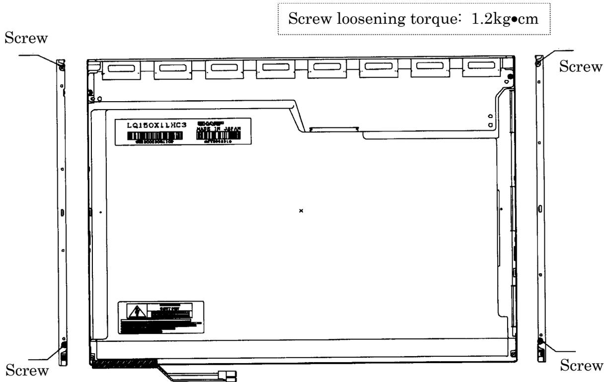
Figure 4-68 Replacing Sharp fluorescent lamp (XGA) (2)
