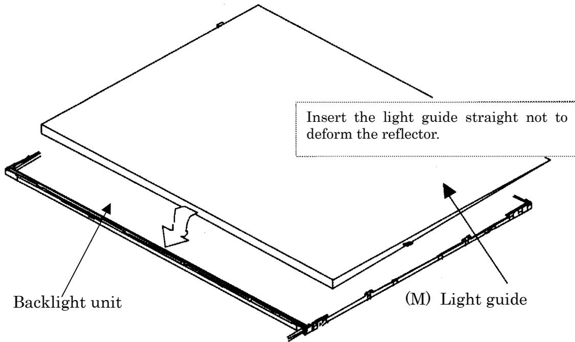
Figure 4-127 Replacing Sharp fluorescent lamp (SXGA+) (15)
