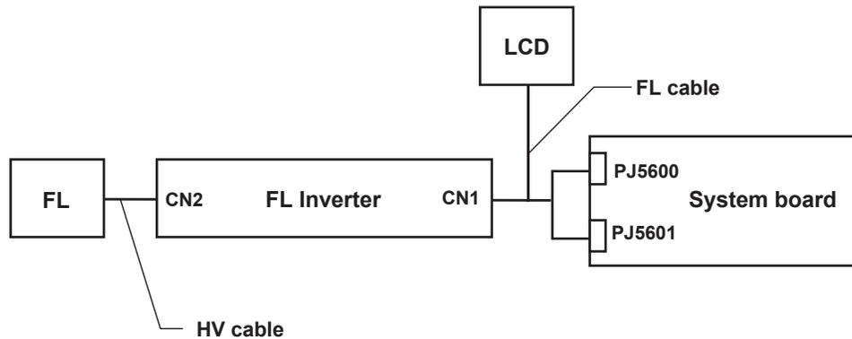
Check 2 The FL cable or HV cable may be defective or damaged. Replace the FL or HV cable with a new one and test the display again. If the problem still exists, perform Check3.
