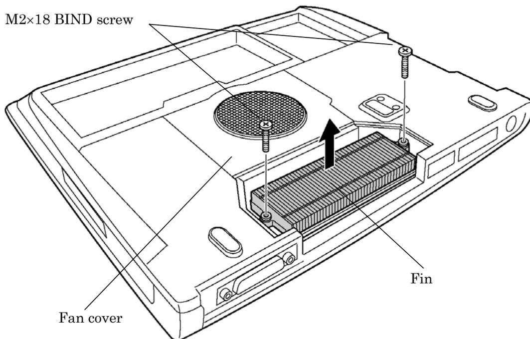
Figure4-12 Removing the Fin
