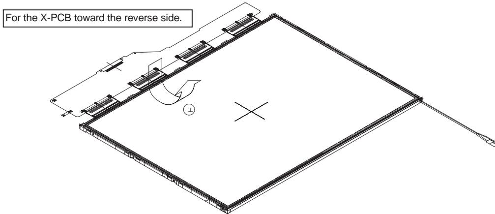
Figure 4-146 Folding down the TAB
