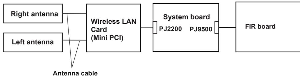
Any of the connections may be disconnected. Disassemble the computer following the steps described in Chapter 4, perform the following checks:
