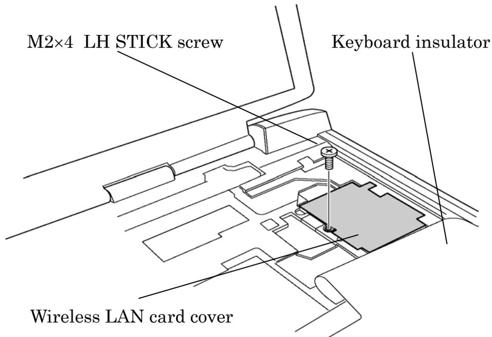
Figure 4-19 Removing the Wireless LAN card cover
