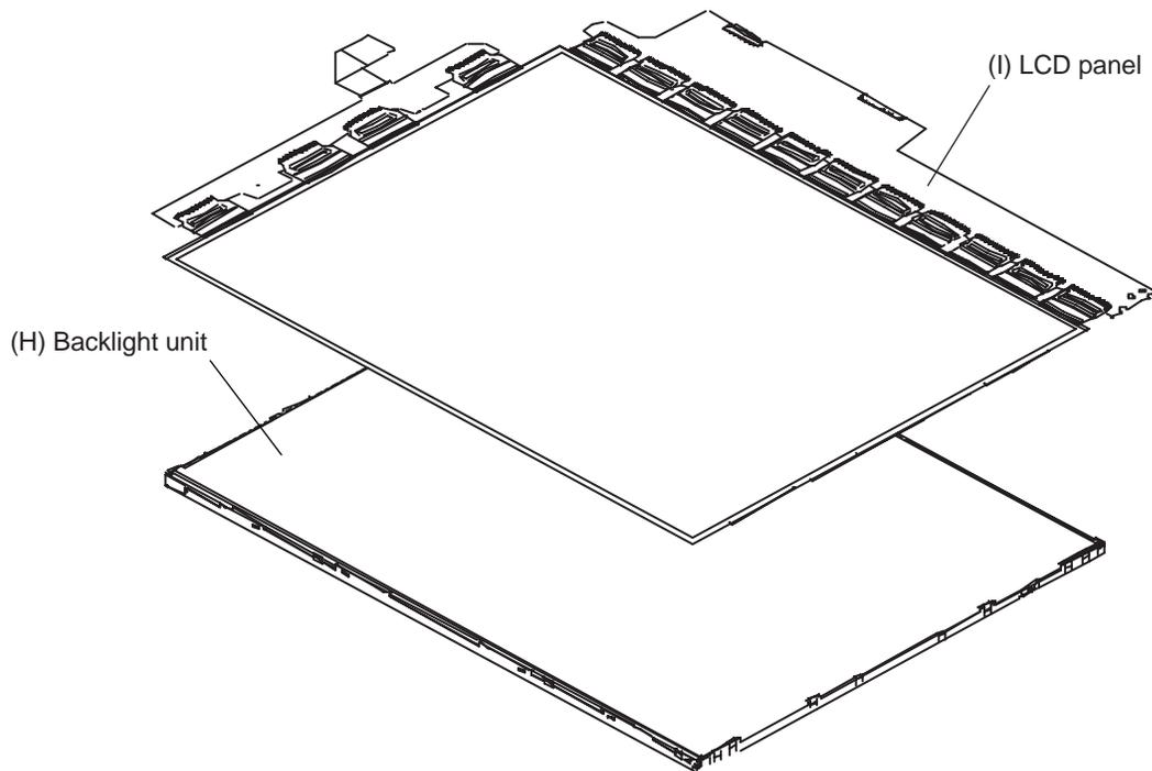
Figure 4-118 Replacing Sharp fluorescent lamp (SXGA+) (6)
