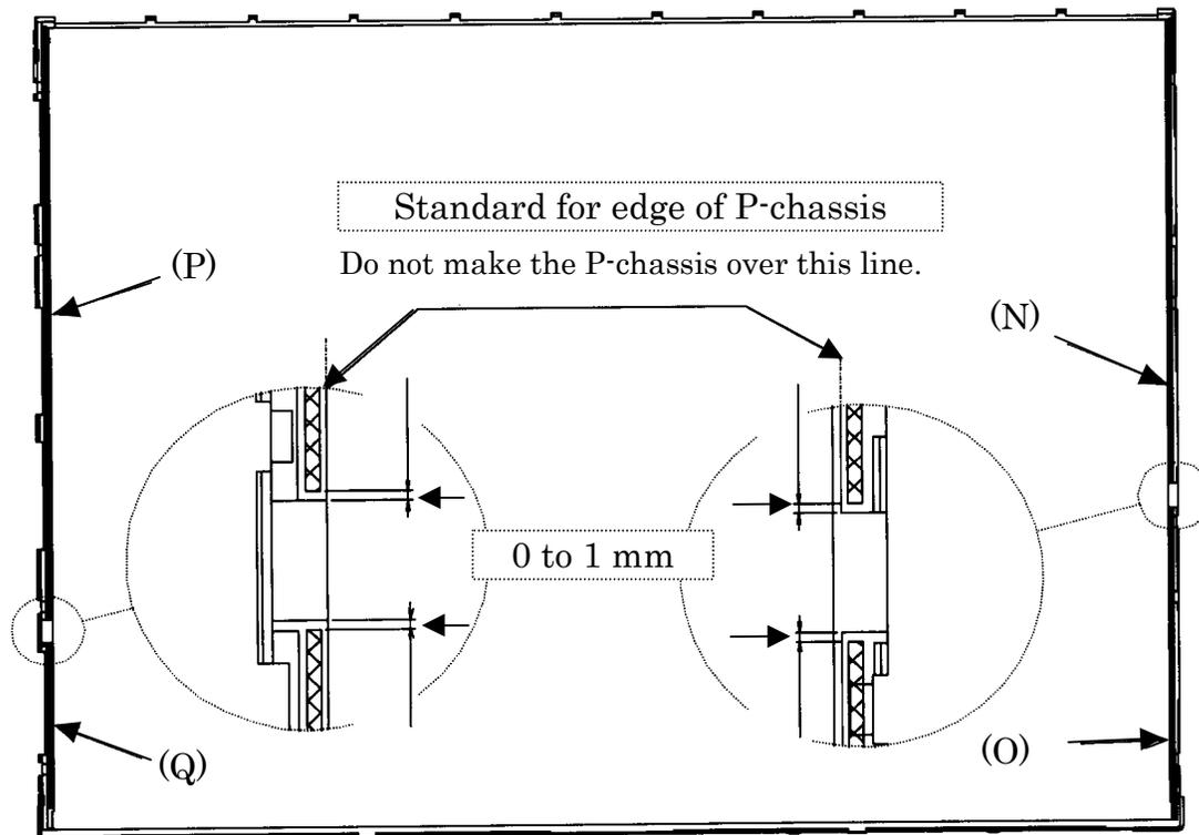
Figure 4-77 Replacing Sharp fluorescent lamp (XGA) (11)
