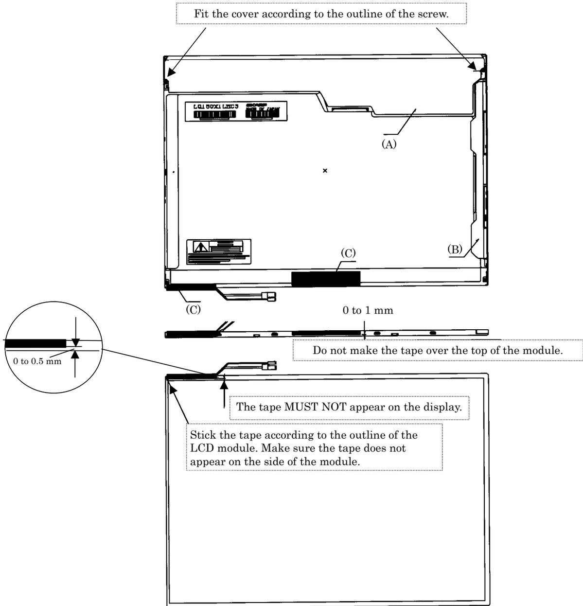
Figure 4-89 Replacing Sharp fluorescent lamp (XGA) (23)
