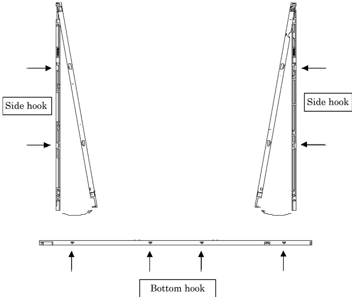
Figure 4-61 Replacing Samsung fluorescent lamp (XGA) (4)
