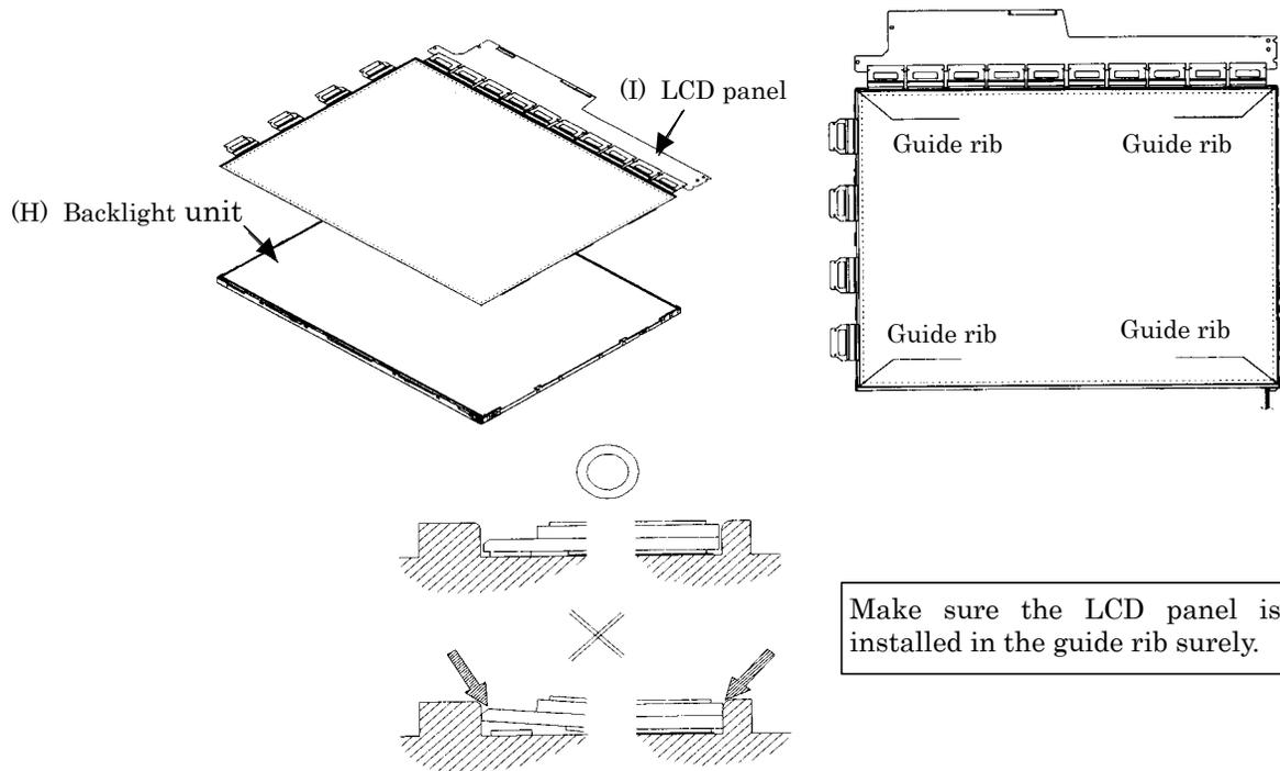
Figure 4-83 Replacing Sharp fluorescent lamp (XGA) (17)
