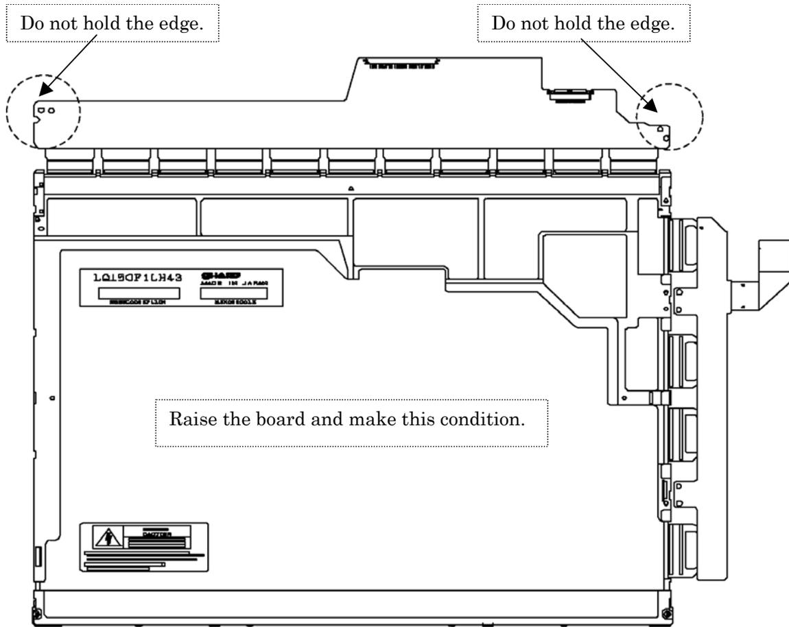
Figure 4-117 Replacing Sharp fluorescent lamp (SXGA+) (5)
