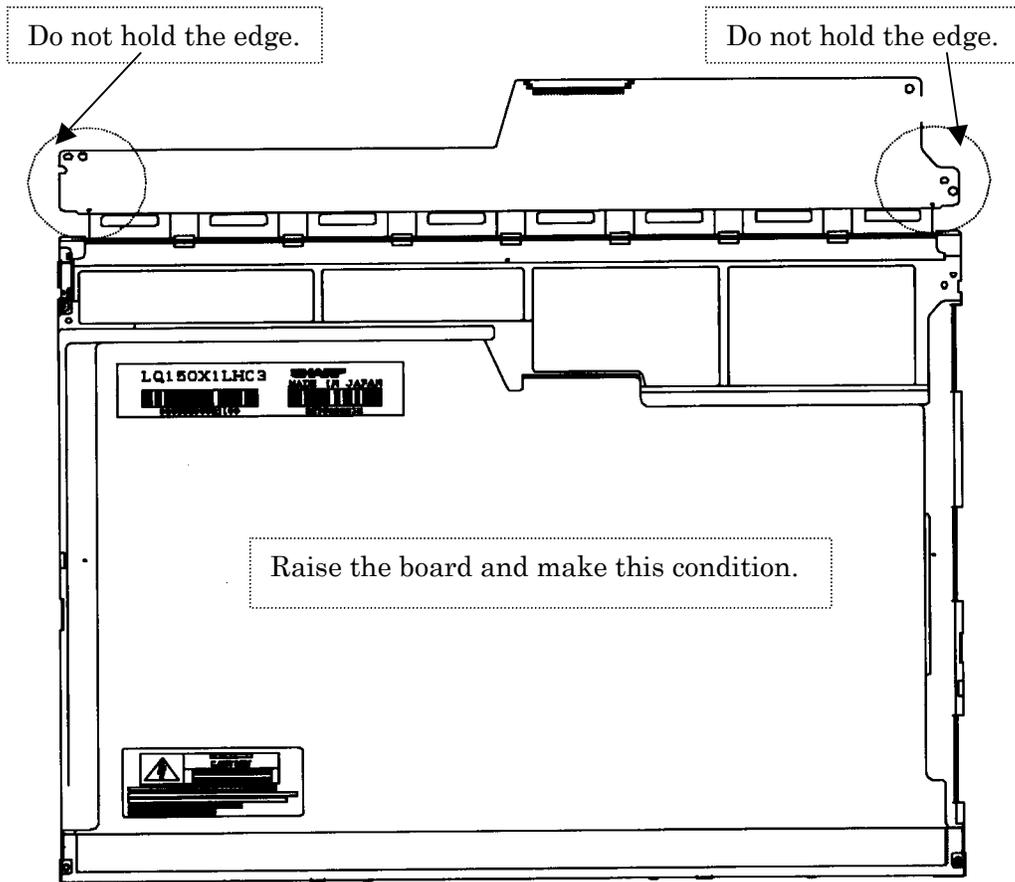
Figure 4-71 Replacing Sharp fluorescent lamp (XGA) (5)
