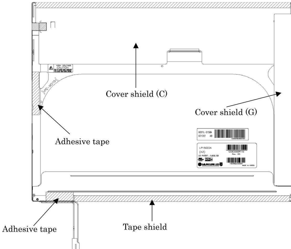
Figure 4-103 Replacing LG.Philips fluorescent lamp (SXGA+) (8)
