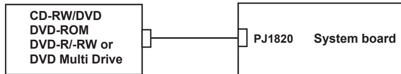
If the connection is loose, reconnect firmly and repeat Procedure 2. If there is still an error, go to Check 2.
