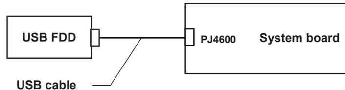
If any of the connections is loose, reconnect firmly and repeat Procedure 2. If any of the connections is damaged, or there is still an error, go to Check 2.
