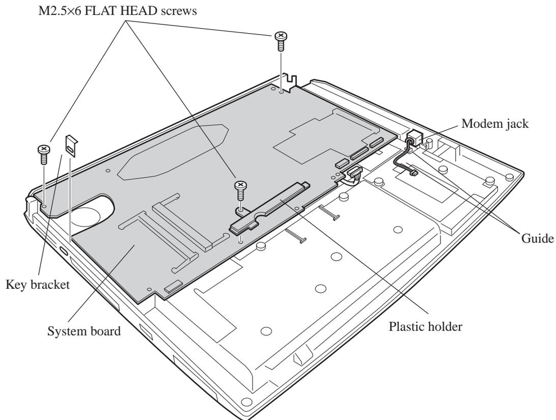
*Figure 4-31 Removing the System board*
