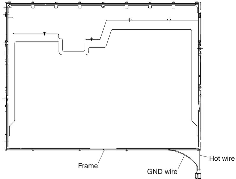
*Figure 4-166 Disconnecting the FL tube ground wire*
