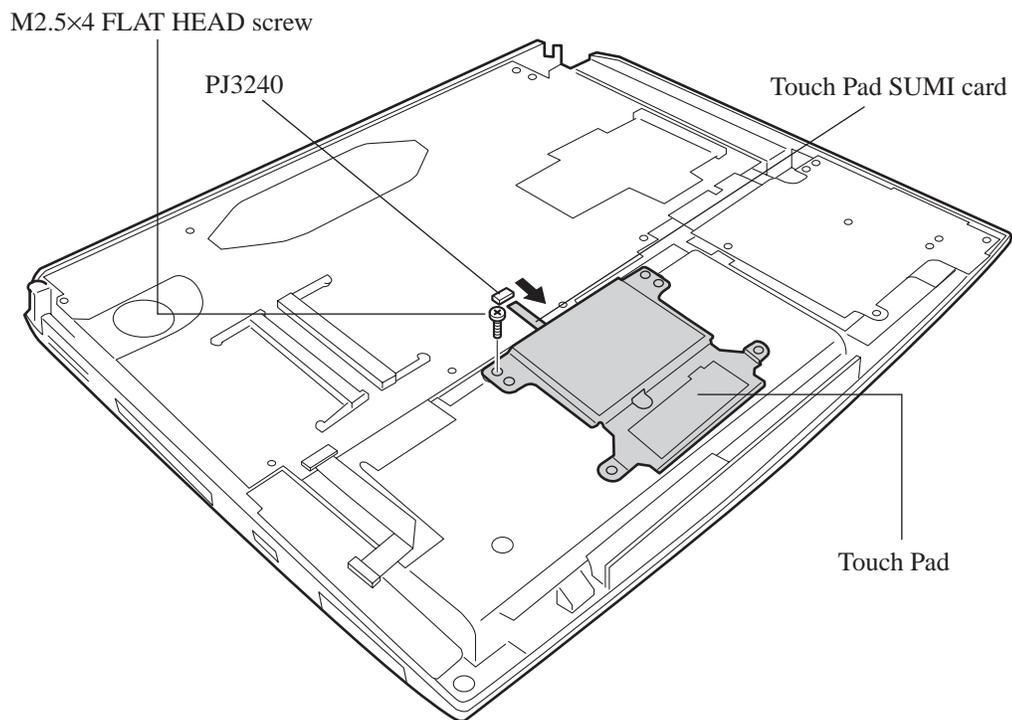
*Figure 4-25 Removing the Touch Pad*
