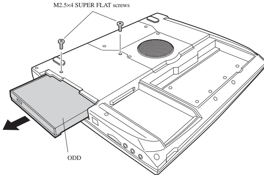
Figure 4-8 Removing the ODD
