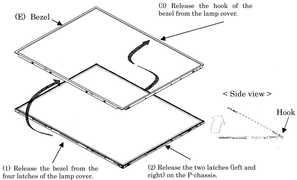
Figure 4-69 Replacing Sharp fluorescent lamp (XGA) (3)
