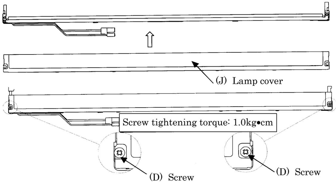
Figure 4-80 Replacing Sharp fluorescent lamp (XGA) (14)
