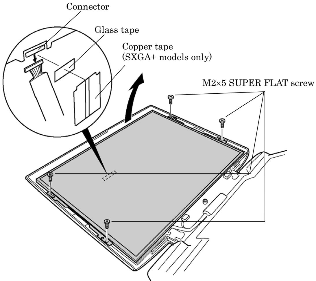
Figure 4-40 Removing the LCD module (1)
