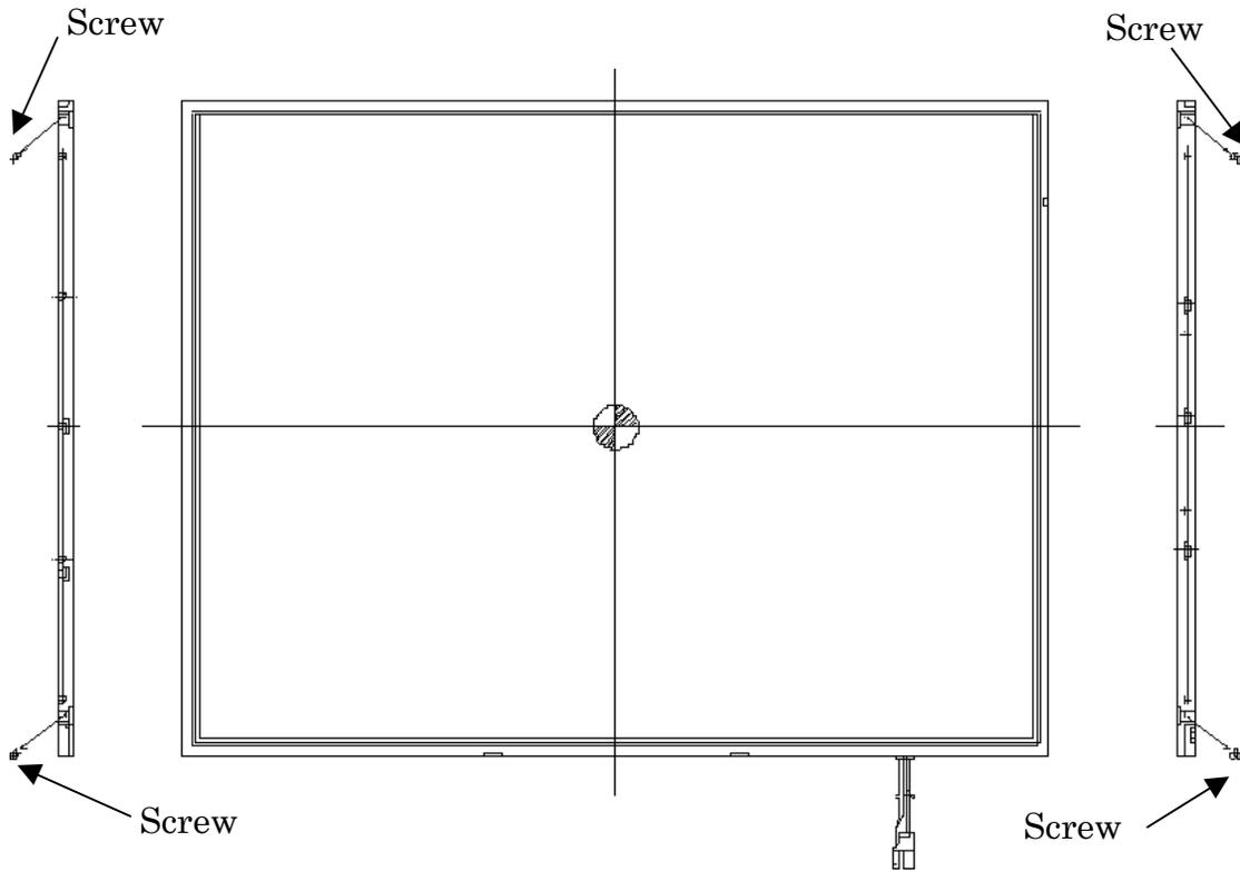
Figure 4-106 Replacing Samsung fluorescent lamp (SXGA+) (3)
