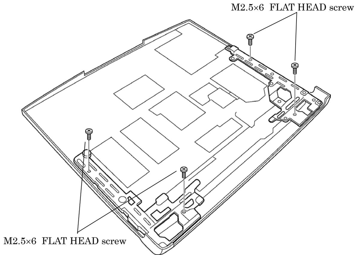
Figure 4-48 Removing the Hinge (2)
