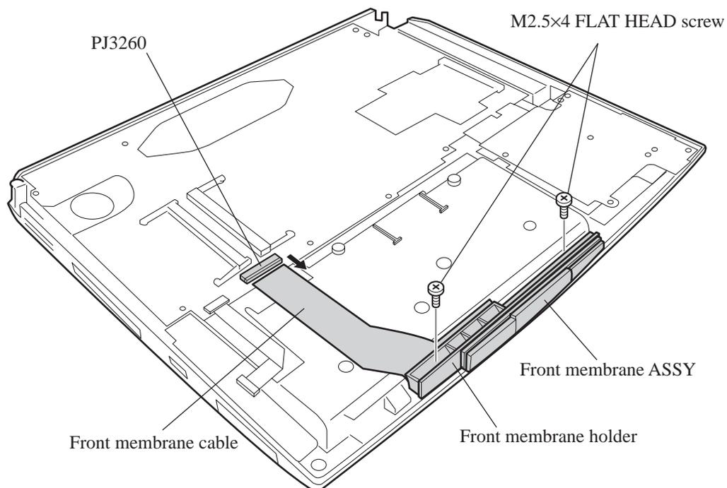
Figure 4-26 Removing the Front membrane ASSY
