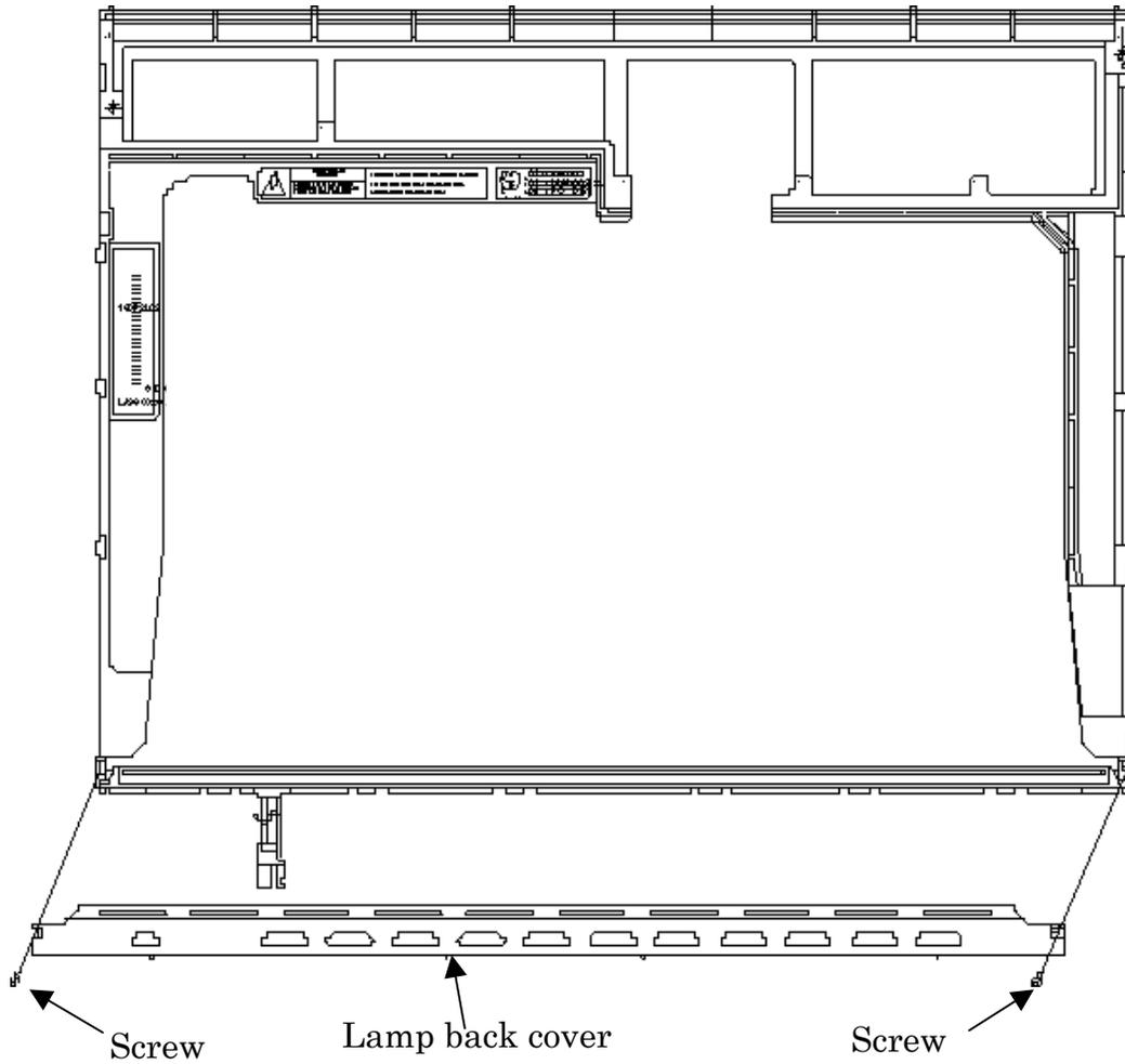
Figure 4-110 Replacing Samsung fluorescent lamp (SXGA+) (7)
