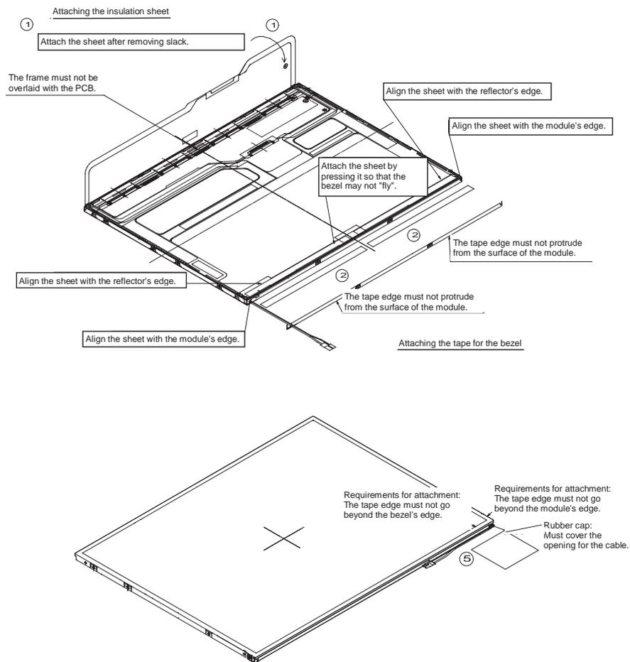
Figure 4-149 Attaching the insulation sheet and tape
