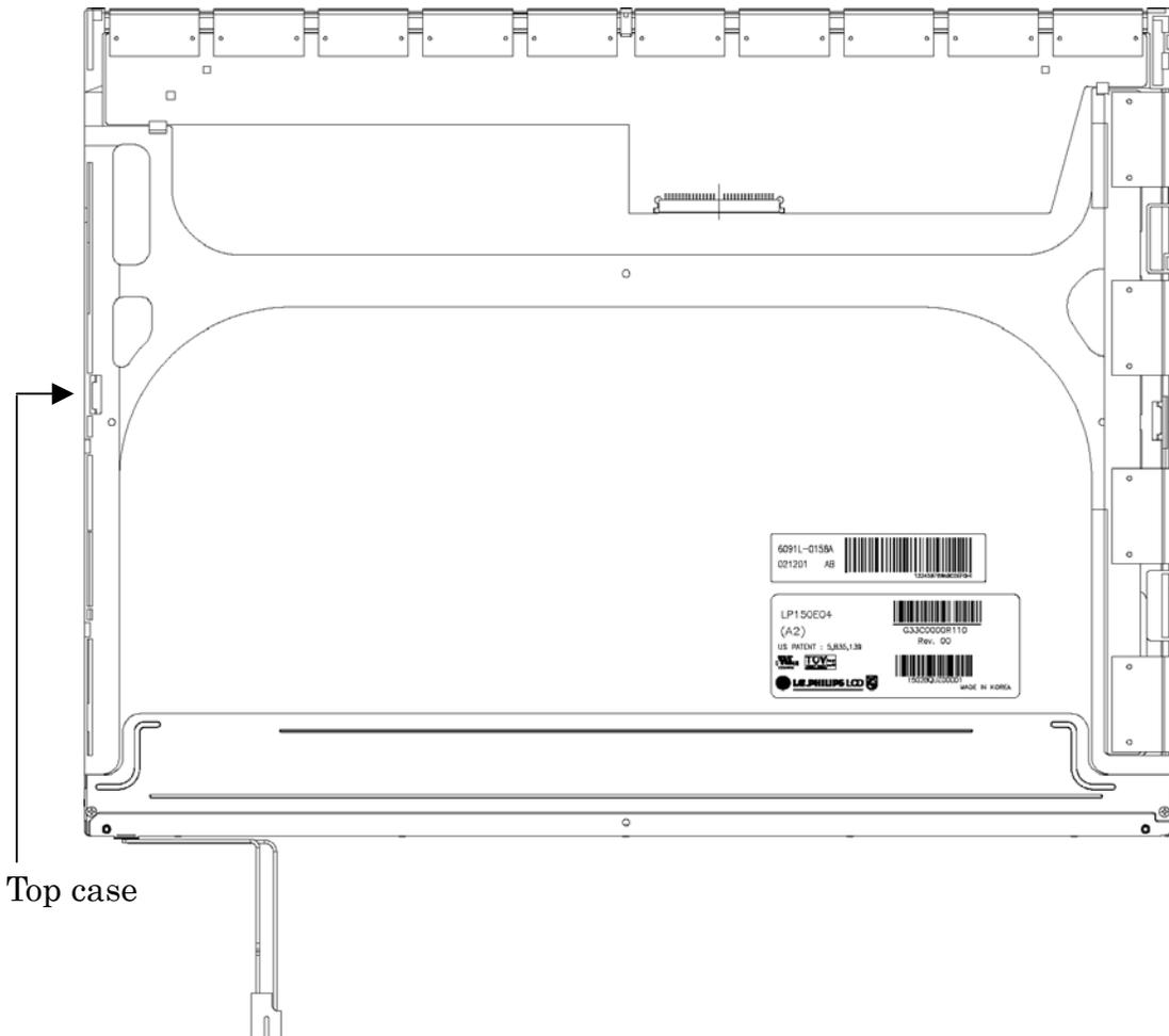
Figure 4-97 Replacing LG.Philips fluorescent lamp (SXGA+) (2)
