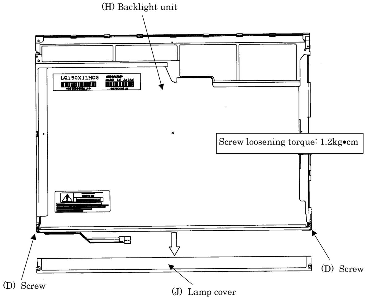
Figure 4-73 Replacing Sharp fluorescent lamp (XGA) (7)
