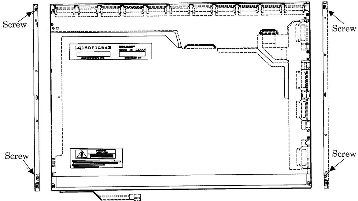
Figure 4-134 Replacing Sharp fluorescent lamp (SXGA+) (22)
