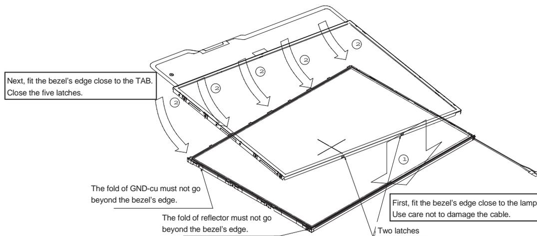
Figure 4-147 Setting the bezel
