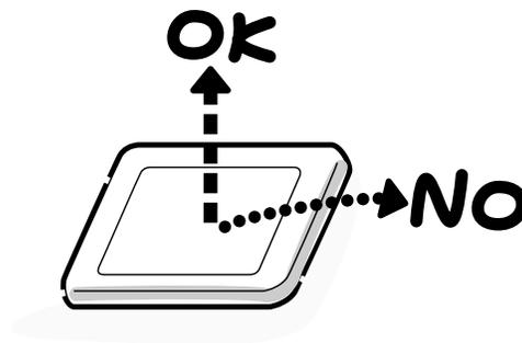
2. For the LCD module, do not force the module into place, because stress can affect its performance.
