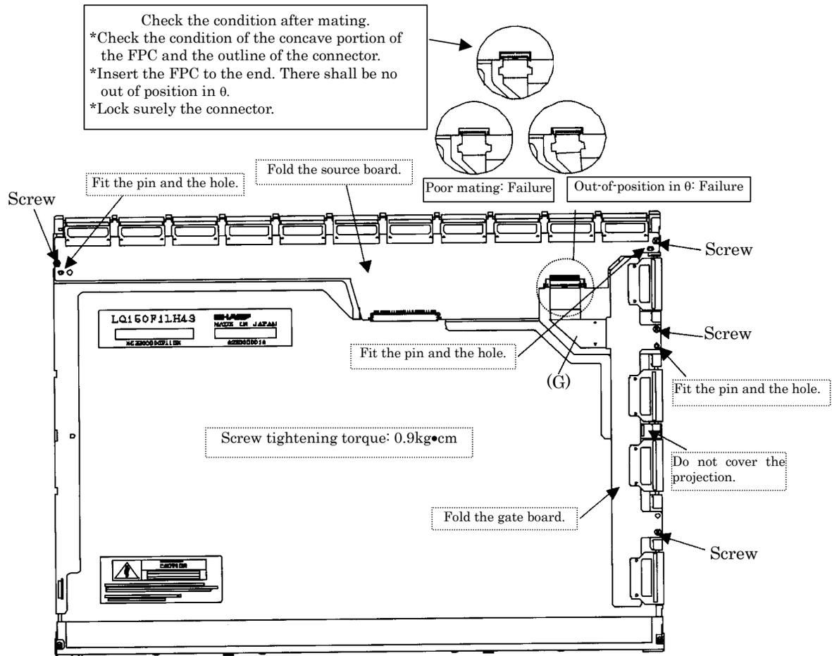
Figure 4-131 Replacing Sharp fluorescent lamp (SXGA+) (19)
