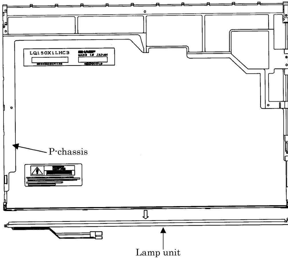
Figure 4-76 Replacing Sharp fluorescent lamp (XGA) (10)
