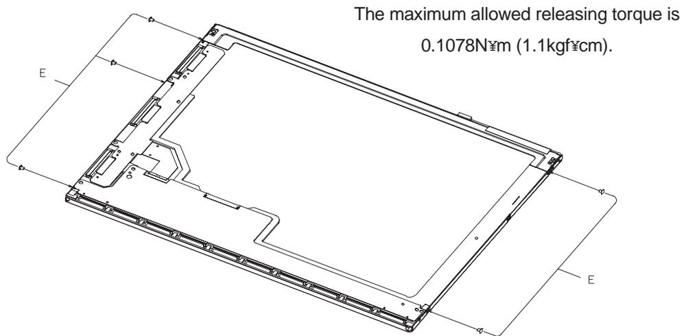
*Figure 4-151 Removing the screws from the sides*
