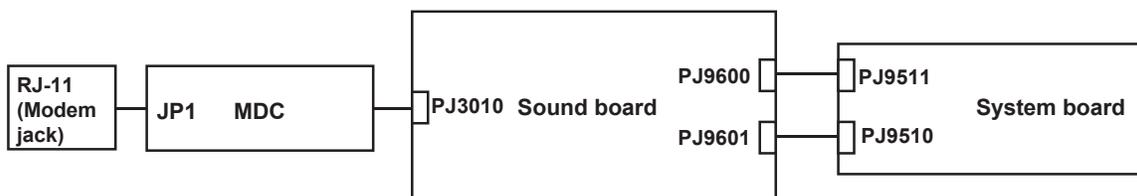
If a connector is disconnected, connect it firmly and repeat Procedure 1. If the Modem is still not functioning properly, perform Check 2.
