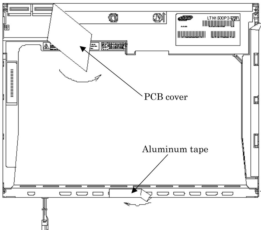
Figure 4-104 Replacing Samsung fluorescent lamp (SXGA+) (1)
