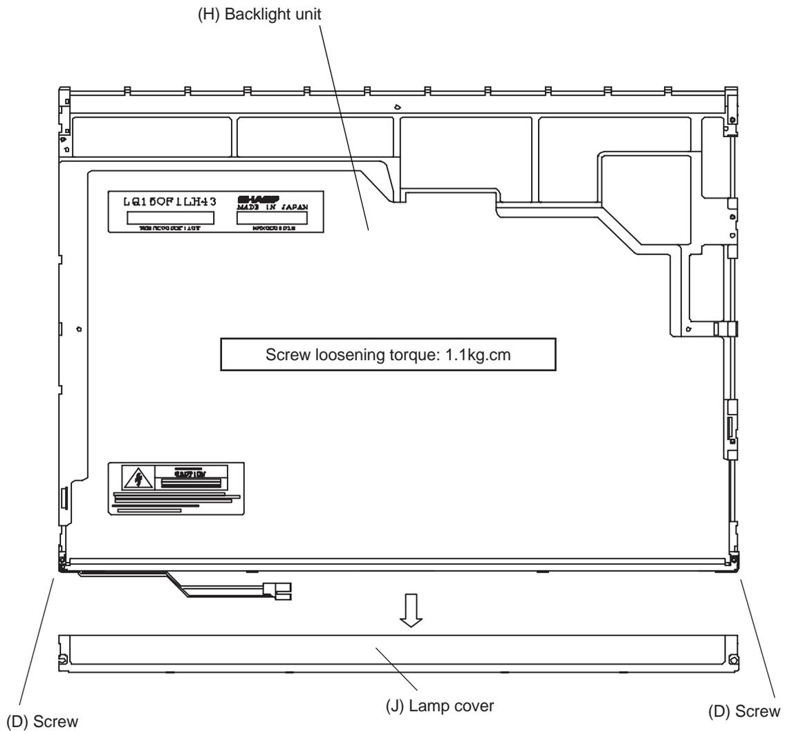
Figure 4-119 Replacing Sharp fluorescent lamp (SXGA+) (7)
