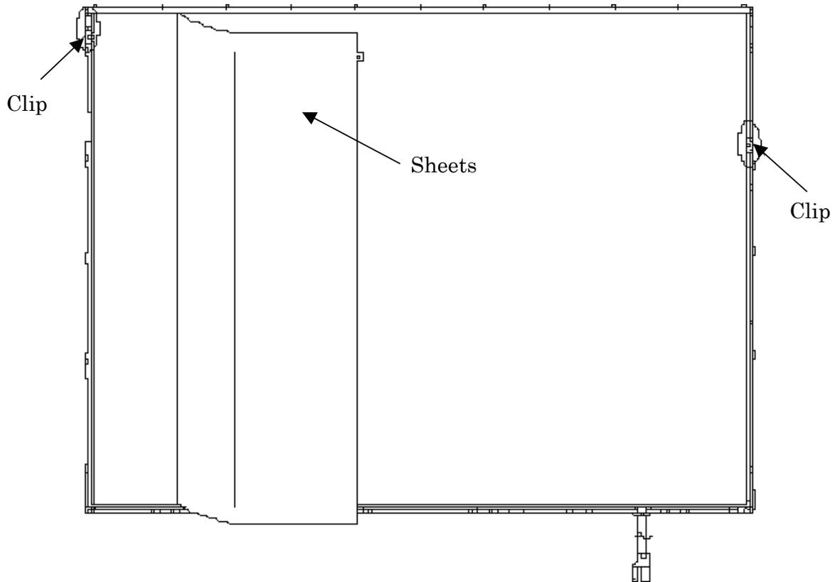
Figure 4-109 Replacing Samsung fluorescent lamp (SXGA+) (6)
