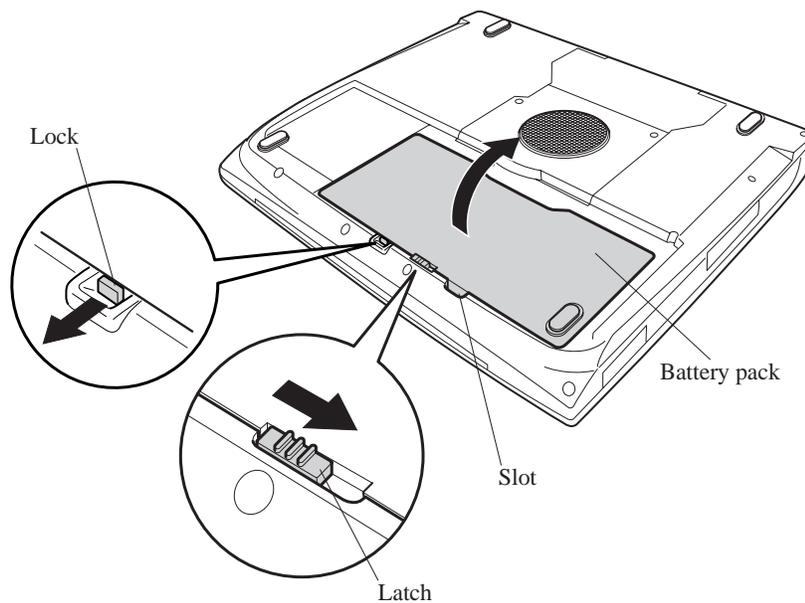
Figure 4-1 Removing the Battery cover
