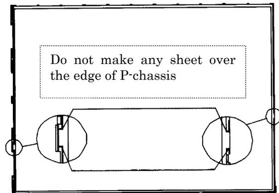
Figure 4-128 Replacing Sharp fluorescent lamp (SXGA+) (16)
