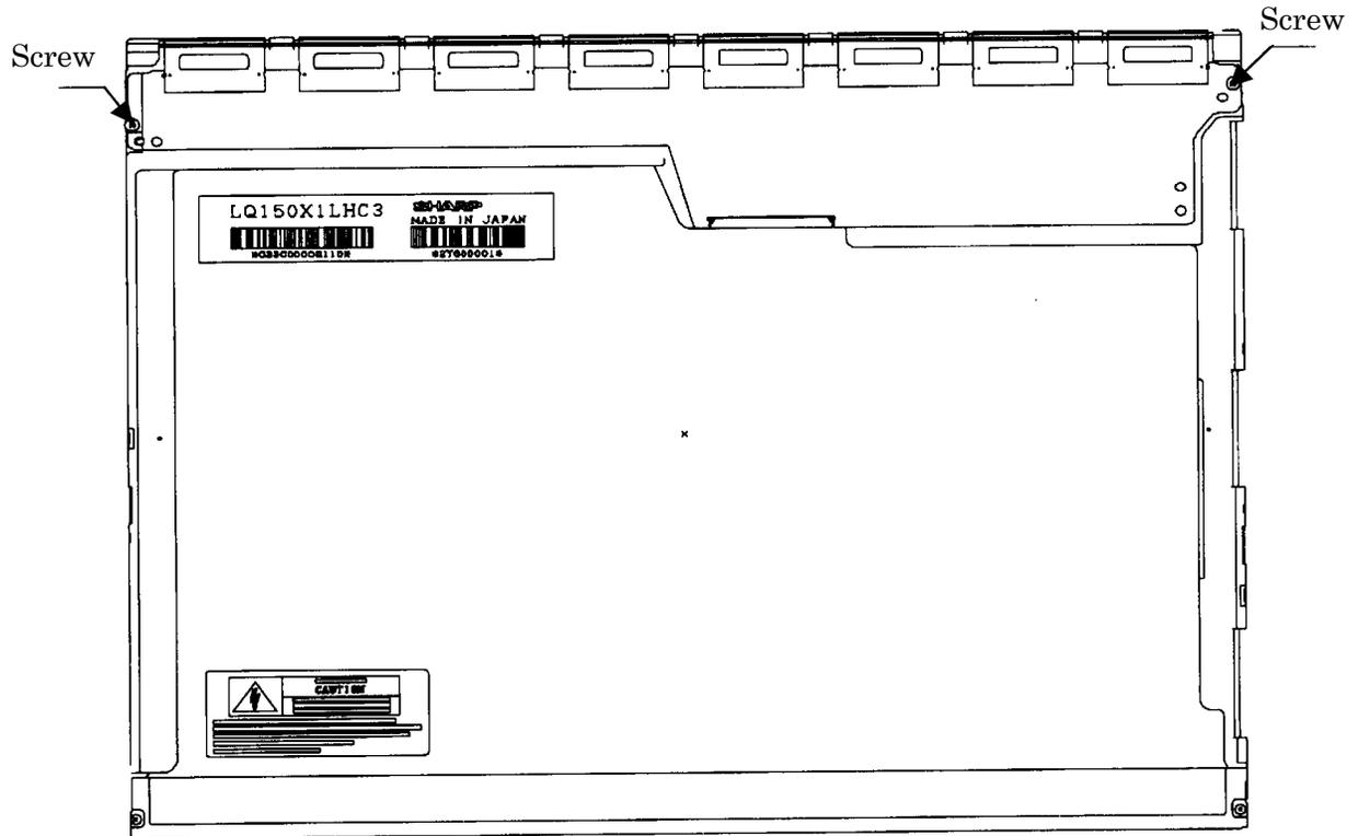
Figure 4-85 Replacing Sharp fluorescent lamp (XGA) (19)
