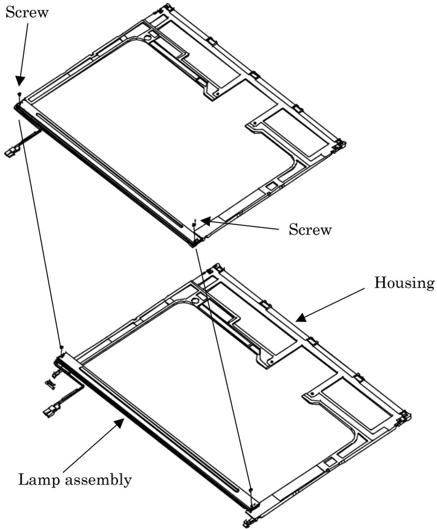
Figure 4-95 Replacing CHIMEI fluorescent lamp (XGA) (6)
