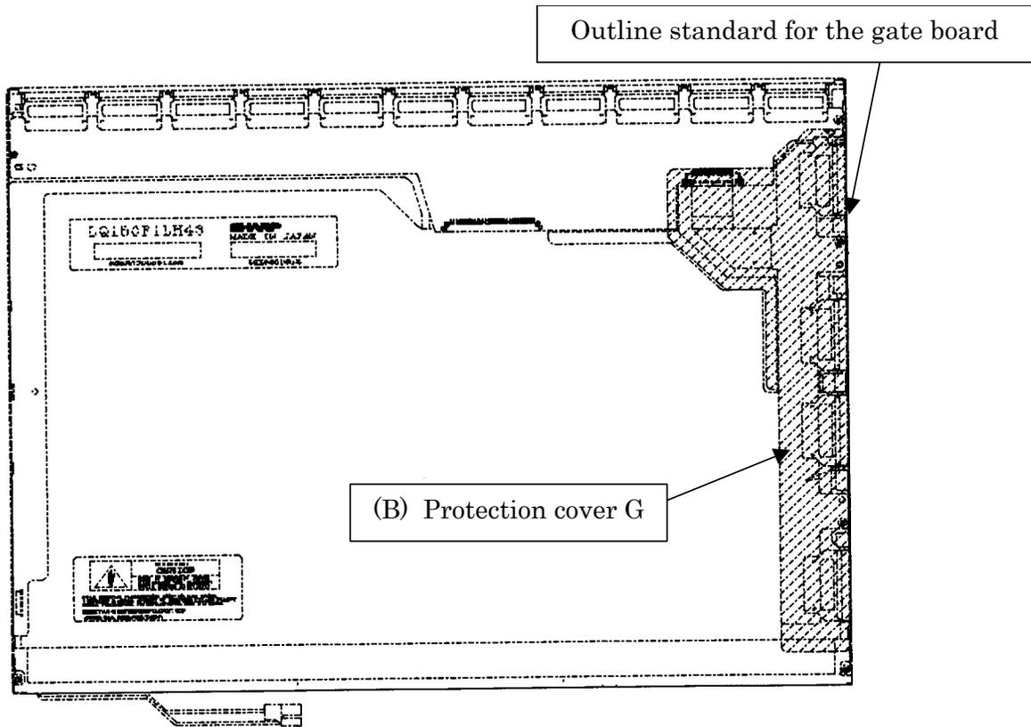
Figure 4-135 Replacing Sharp fluorescent lamp (SXGA+) (23)
