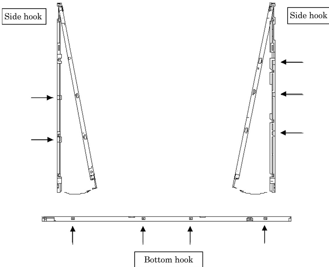
Figure 4-107 Replacing Samsung fluorescent lamp (SXGA+) (4)
