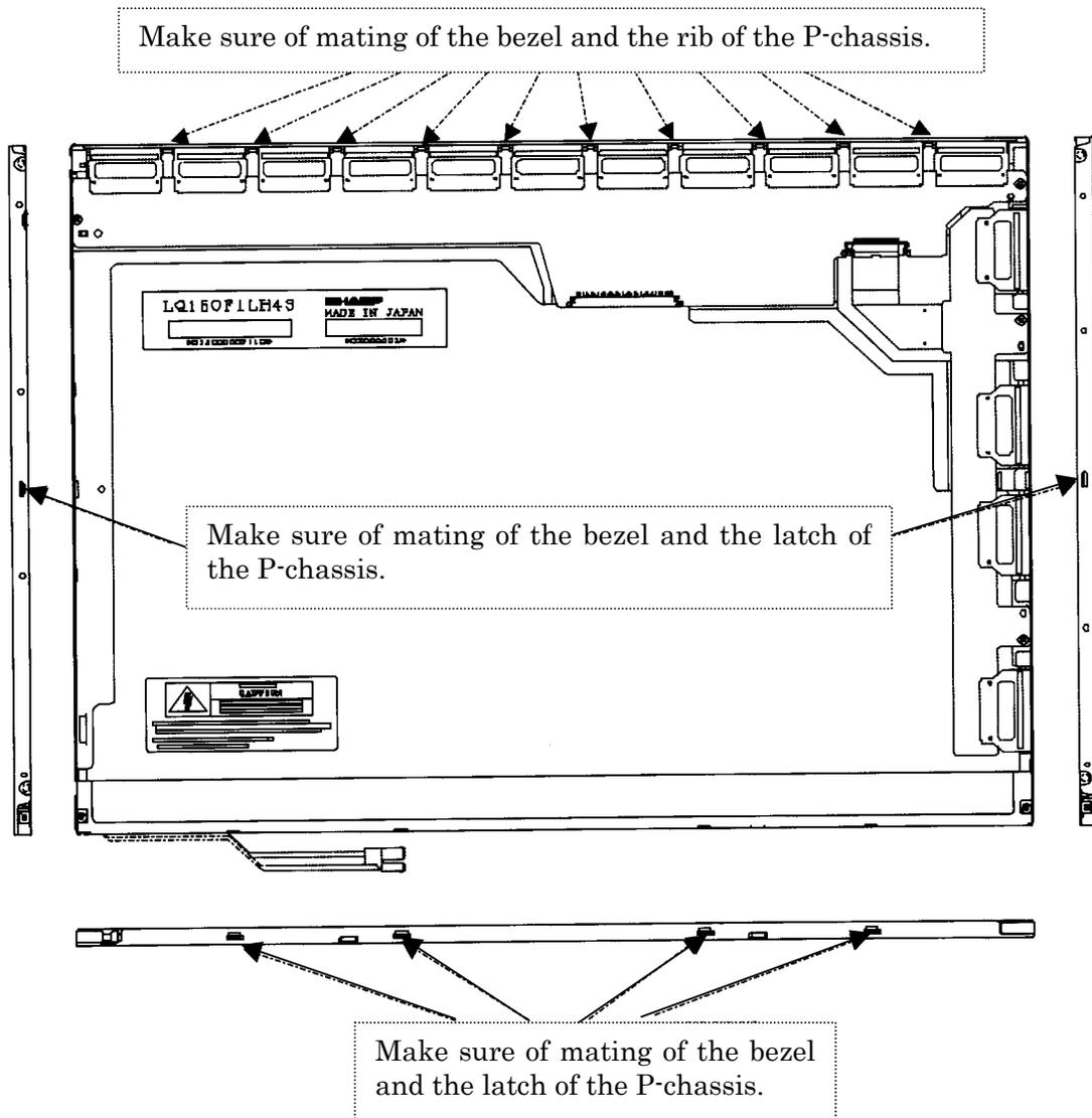
Figure 4-133 Replacing Sharp fluorescent lamp (SXGA+) (21)
