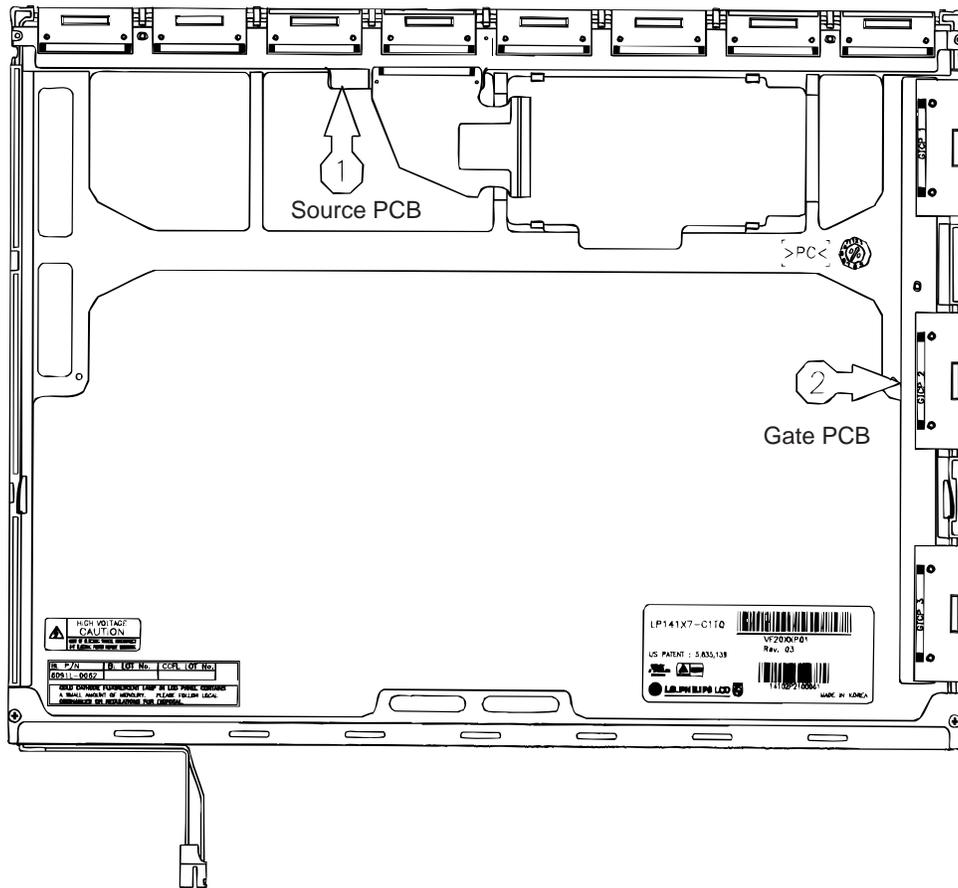
Figure 4-173 Attaching the source PCB and gate PCB
