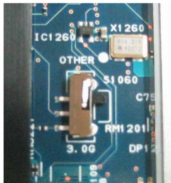
**NOTE:** The position of the SLIDE SWITCH (S1060) can still be changed after completing the assembly by removing the FAN from the bottom of the unit.
