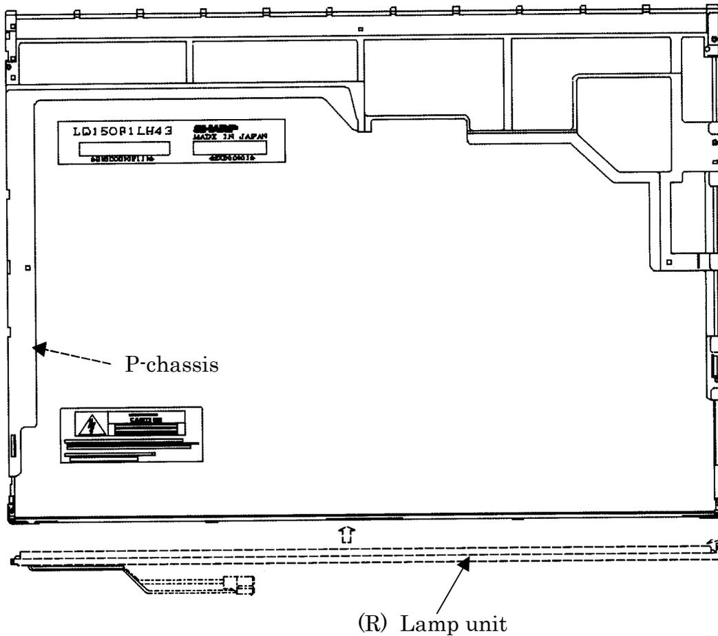
Figure 4-124 Replacing Sharp fluorescent lamp (SXGA+) (12)
