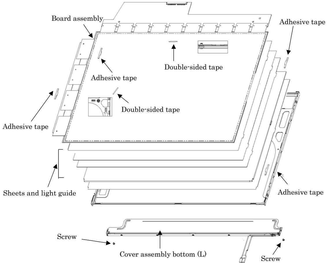
Figure 4-99 Replacing LG.Philips fluorescent lamp (SXGA+) (4)
