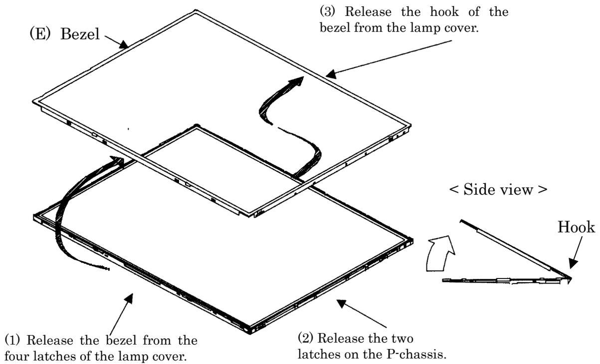
Figure 4-115 Replacing Sharp fluorescent lamp (SXGA+) (3)
