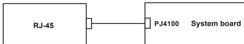
If a connector is disconnected, connect it firmly and repeat Procedure 1. If the LAN port is still not functioning properly, perform Check 2.
