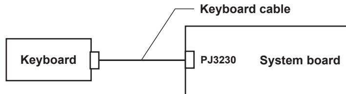
If the connection is loose, reconnect firmly and repeat Procedure 2. If there is still an error, go to Check 2.
