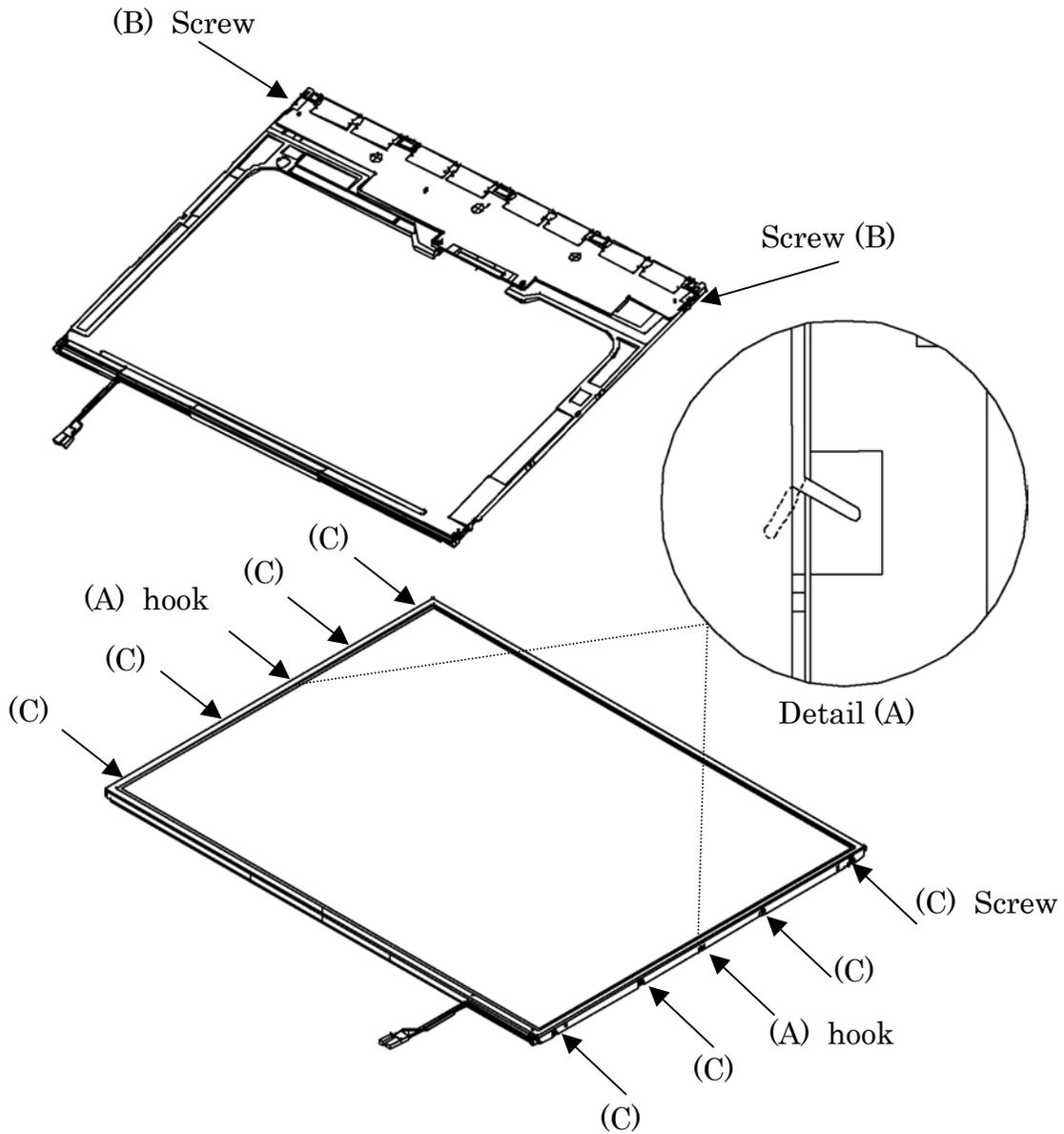
Figure 4-91 Replacing CHIMEI fluorescent lamp (XGA) (2)
