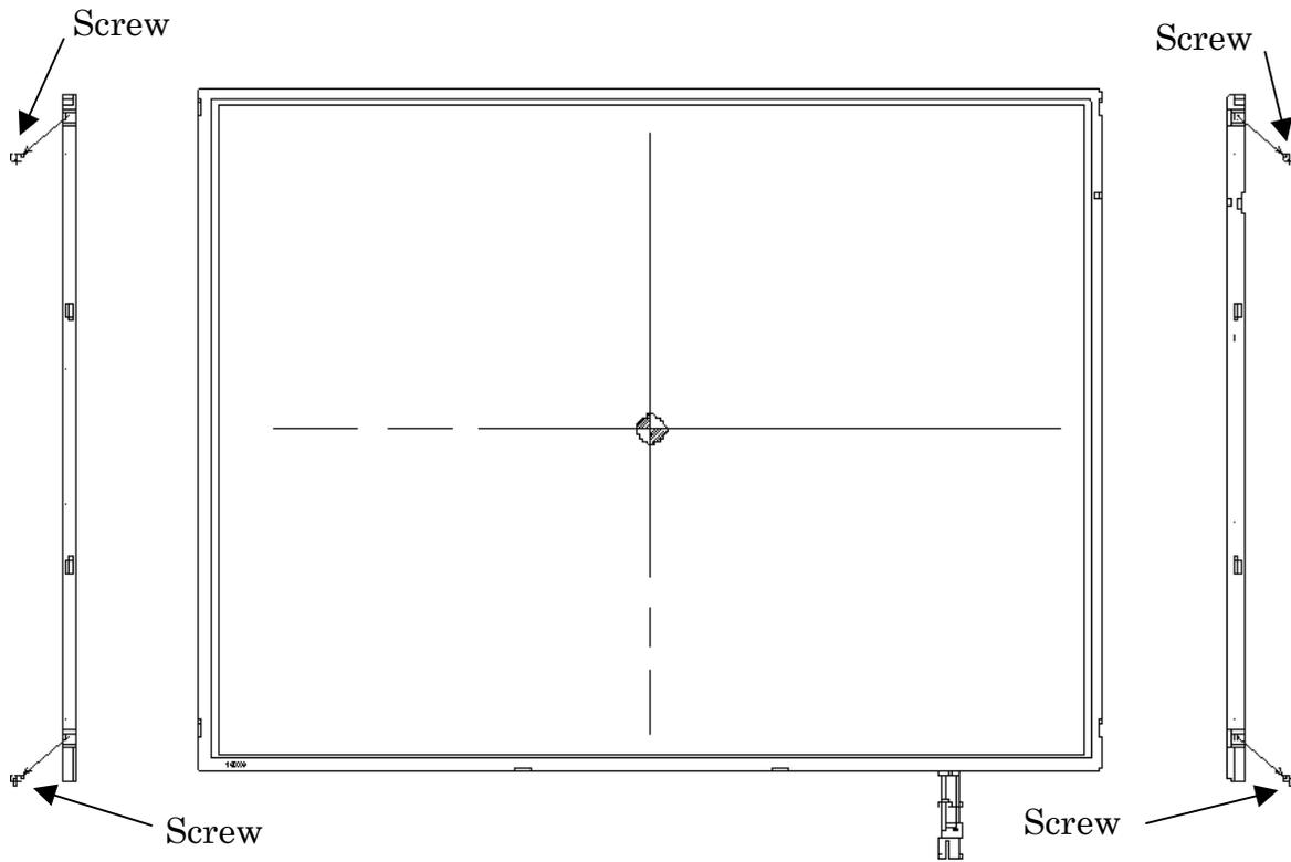
Figure 4-60 Replacing Samsung fluorescent lamp (XGA) (3)
