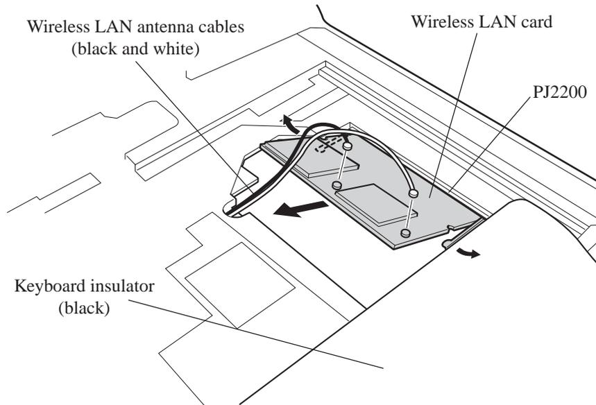
*Figure 4-20 Removing the Wireless LAN card*
