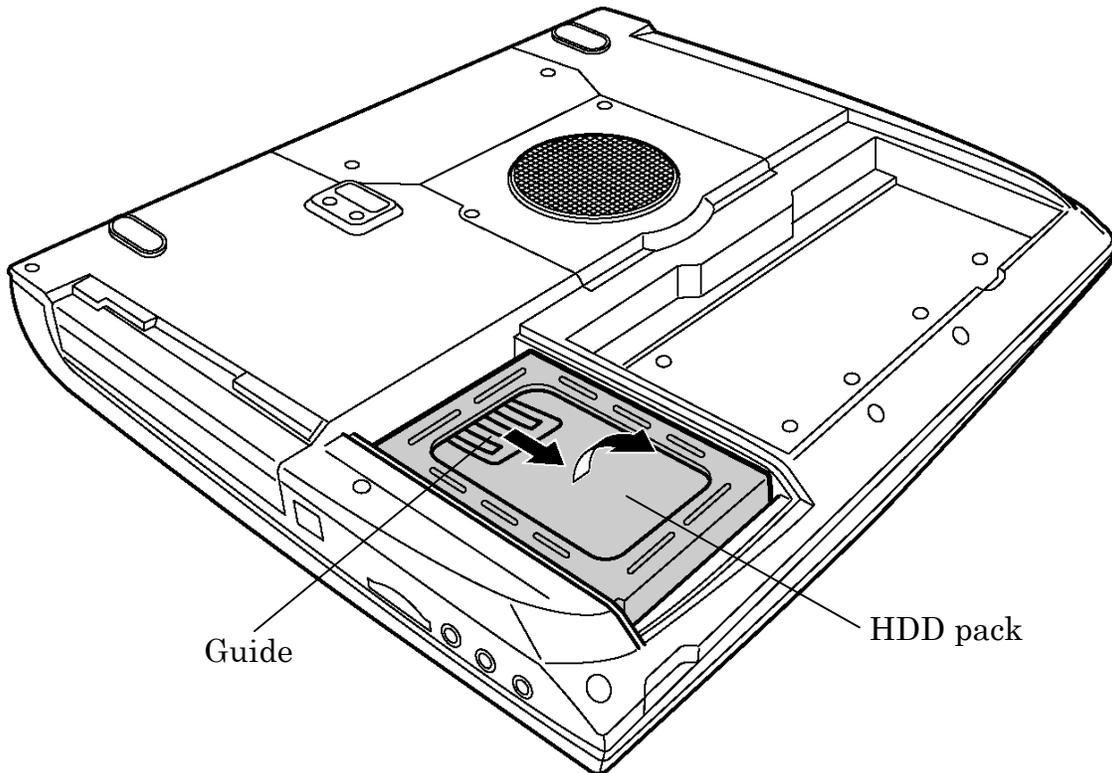
Figure 4-5 Removing the HDD pack
