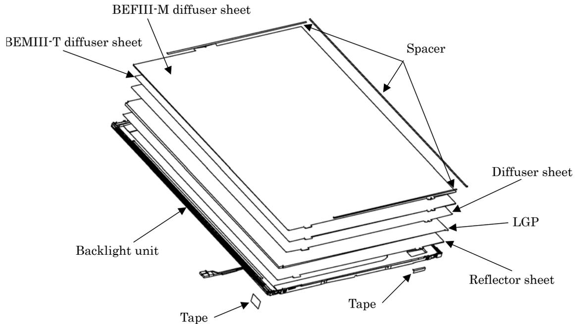
Figure 4-94 Replacing CHIMEI fluorescent lamp (XGA) (5)
