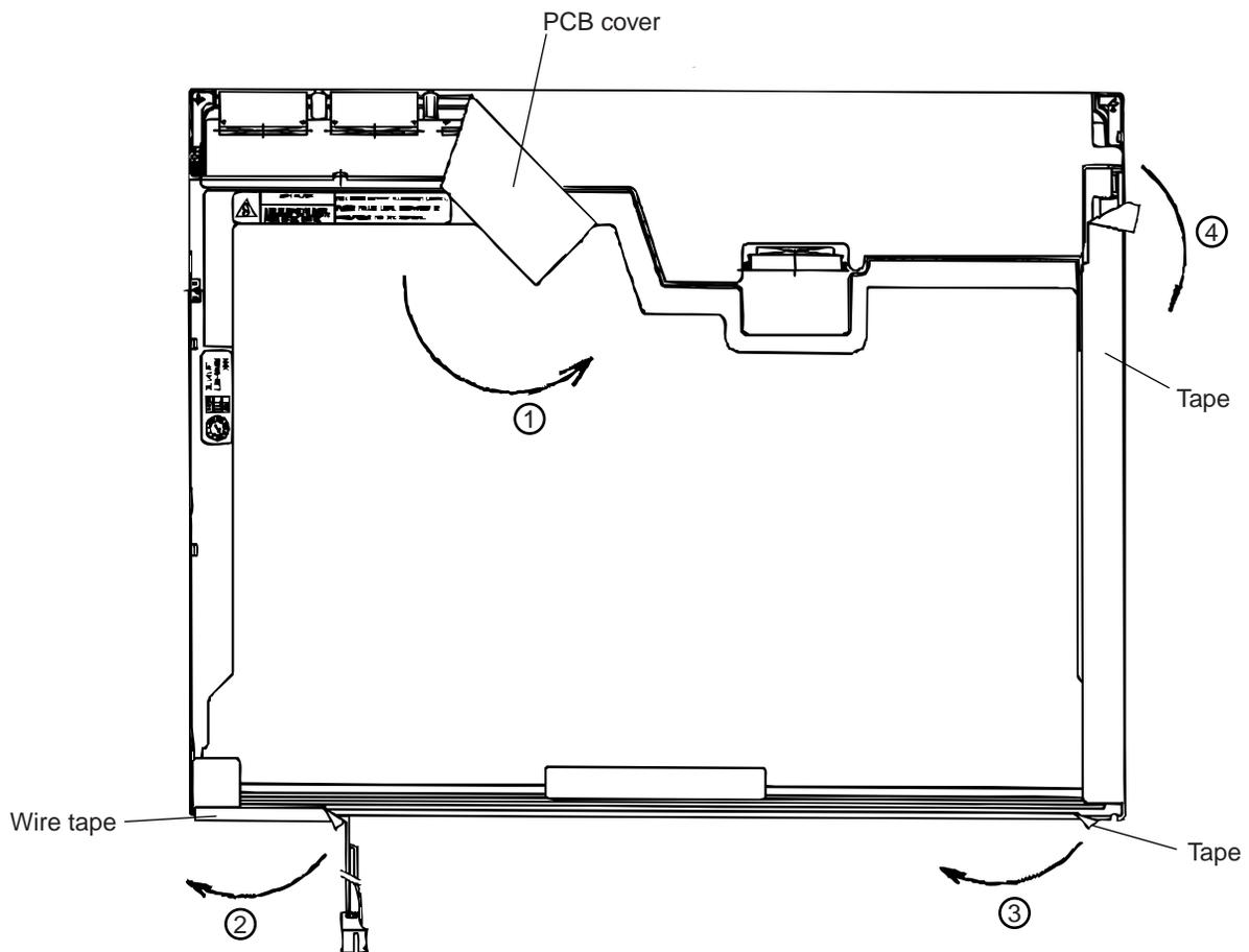
Figure 4-160 Removing the PCB cover and tape
