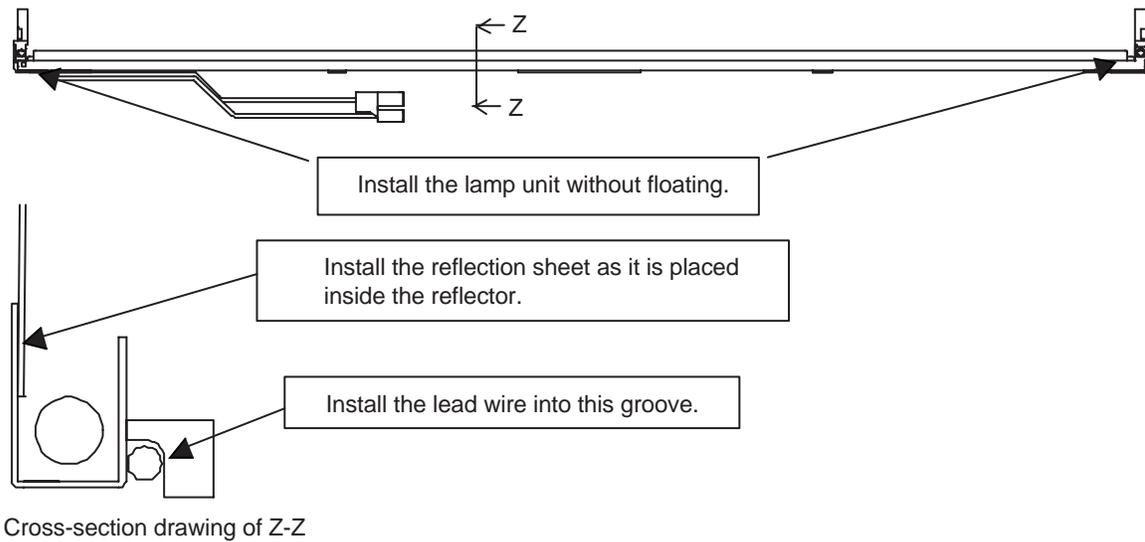
Figure 4-125 Replacing Sharp fluorescent lamp (SXGA+) (13)
