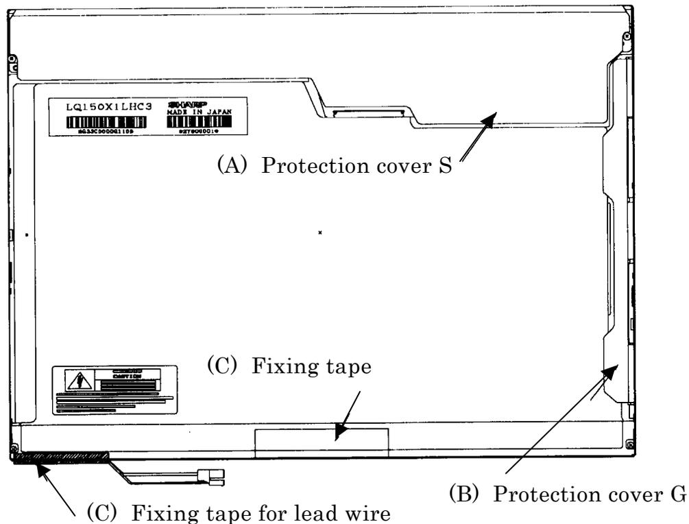
Figure 4-67 Replacing Sharp fluorescent lamp (XGA) (1)
