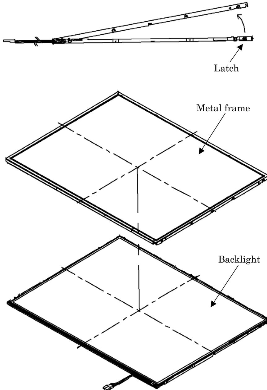
Figure 4-92 Replacing CHIMEI fluorescent lamp (XGA) (3)
