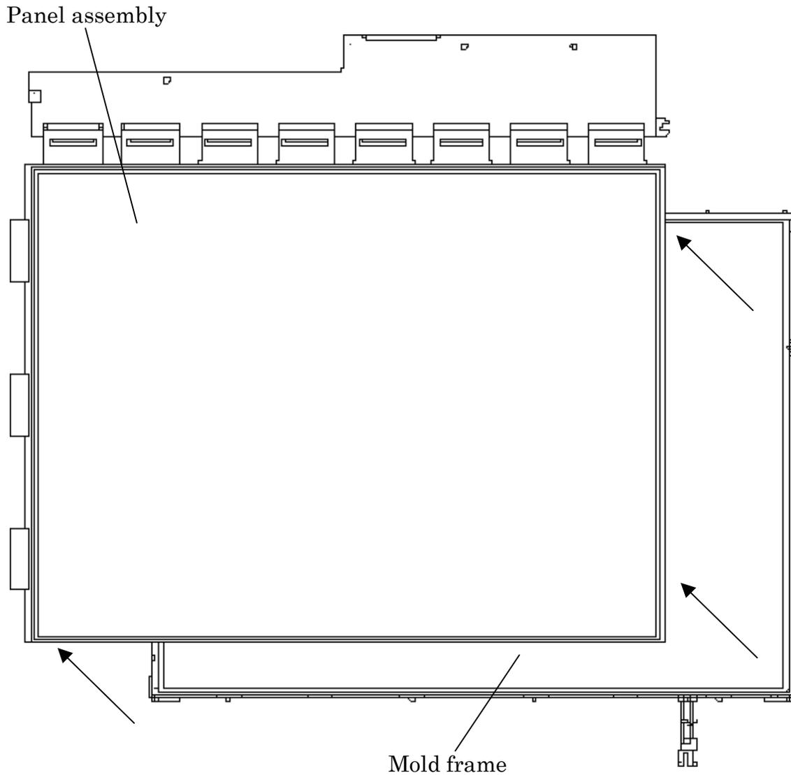
Figure 4-62 Replacing Samsung fluorescent lamp (XGA) (5)
