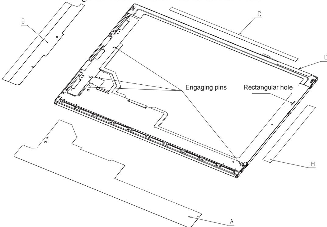
Figure 4-158 Attaching the protection cover and tapes
