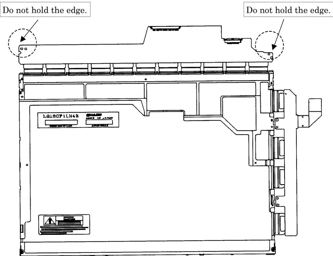
Figure 4-130 Replacing Sharp fluorescent lamp (SXGA+) (18)
