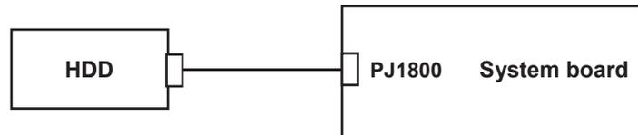
If the connection is loose, reconnect firmly and repeat Procedure 1. If there is still an error, go to Check 2.
