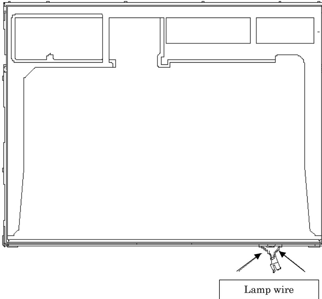
Figure 4-65 Replacing Samsung fluorescent lamp (XGA) (8)
