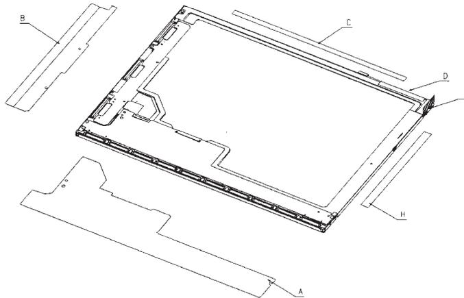
Figure 4-150 Removing the protective cover and tape
