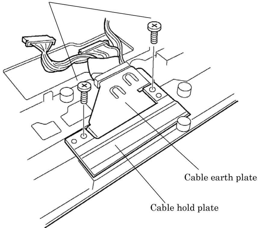
*Figure 4-45 Removing the Cable hold plate/Cable earth plate*
