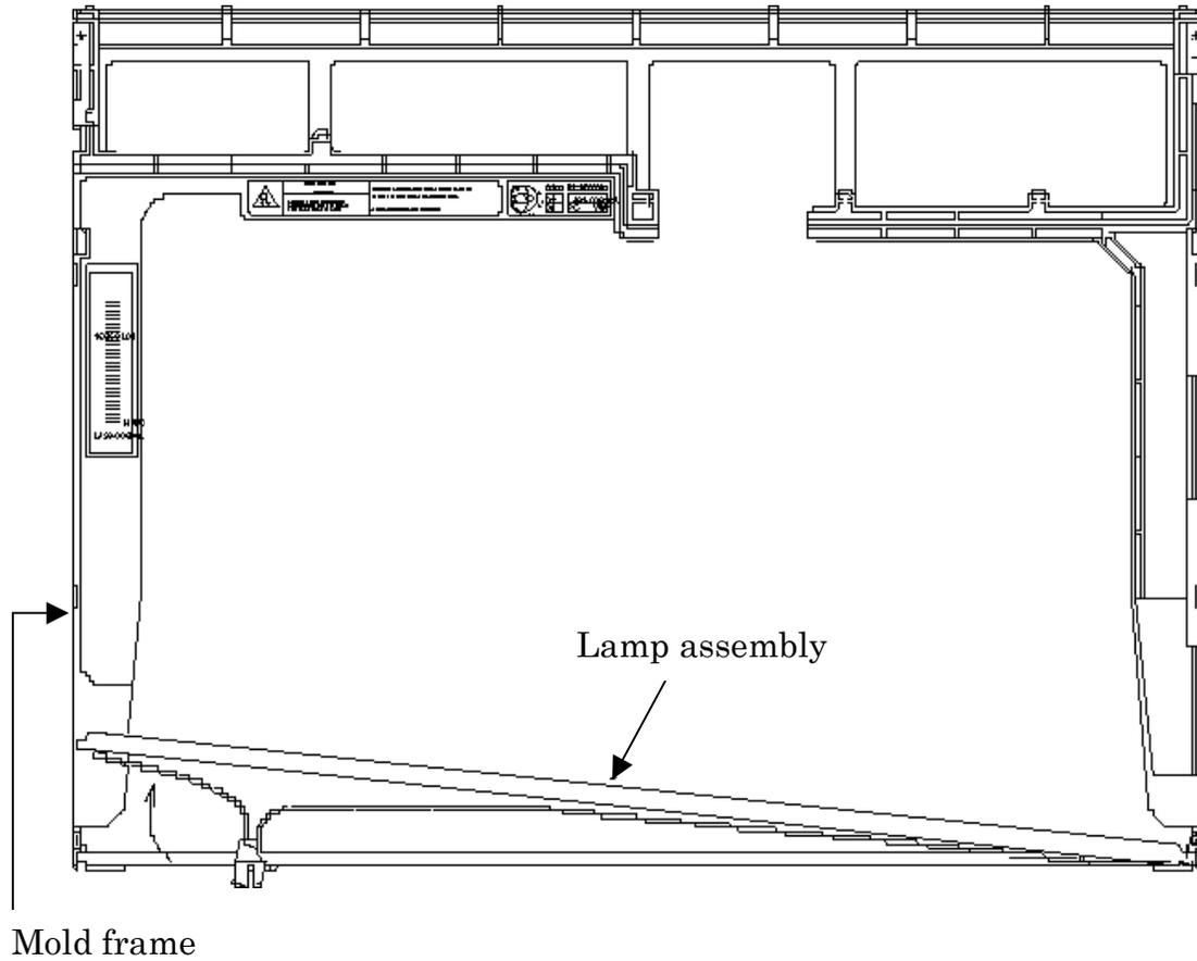
Figure 4-66 Replacing Samsung fluorescent lamp (XGA) (9)
