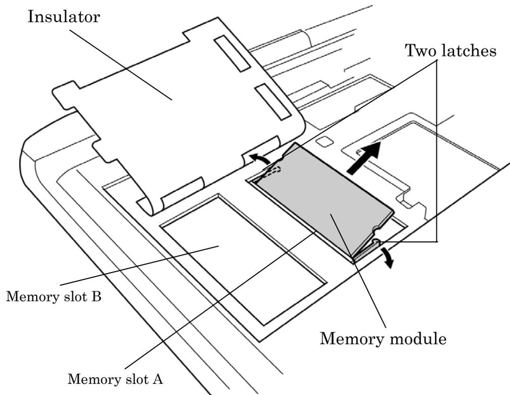
Figure 4-18 Removing the Memory module
