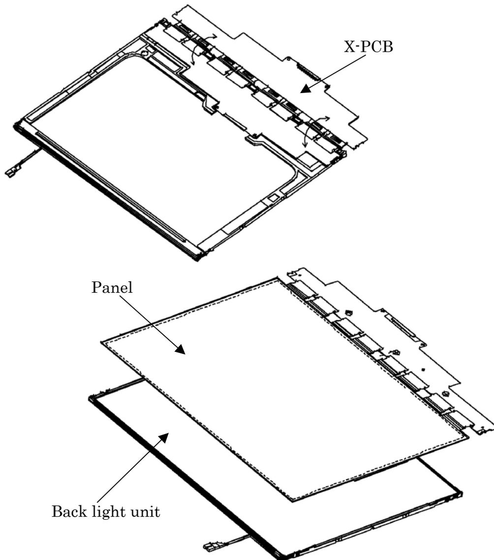
Figure 4-93 Replacing CHIMEI fluorescent lamp (XGA) (4)
