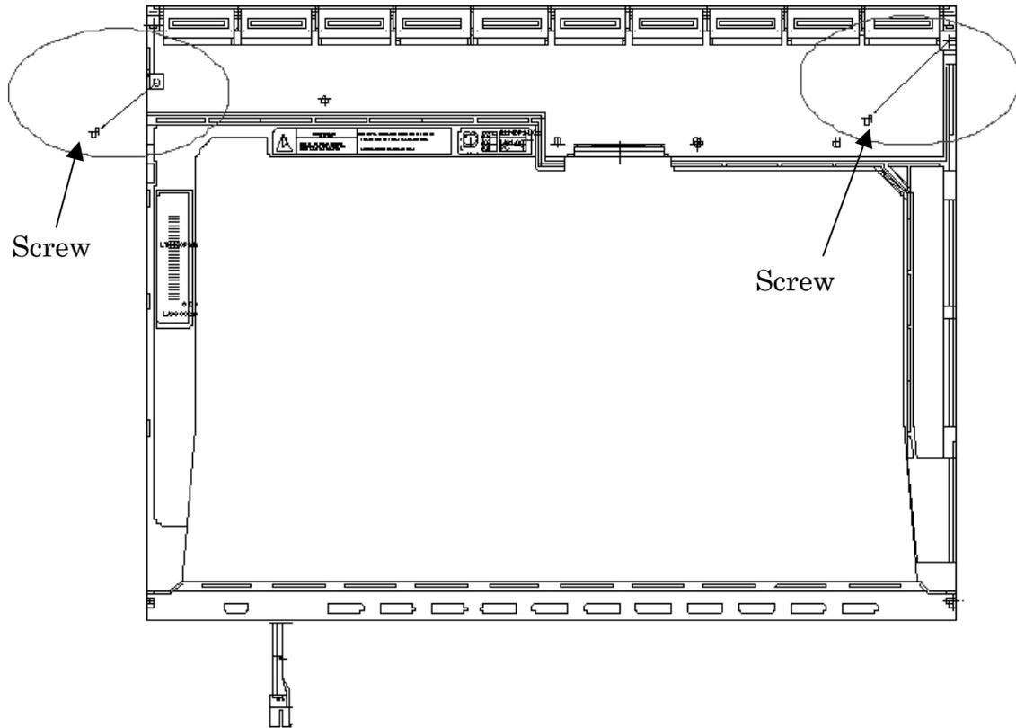
Figure 4-105 Replacing Samsung fluorescent lamp (SXGA+) (2)
