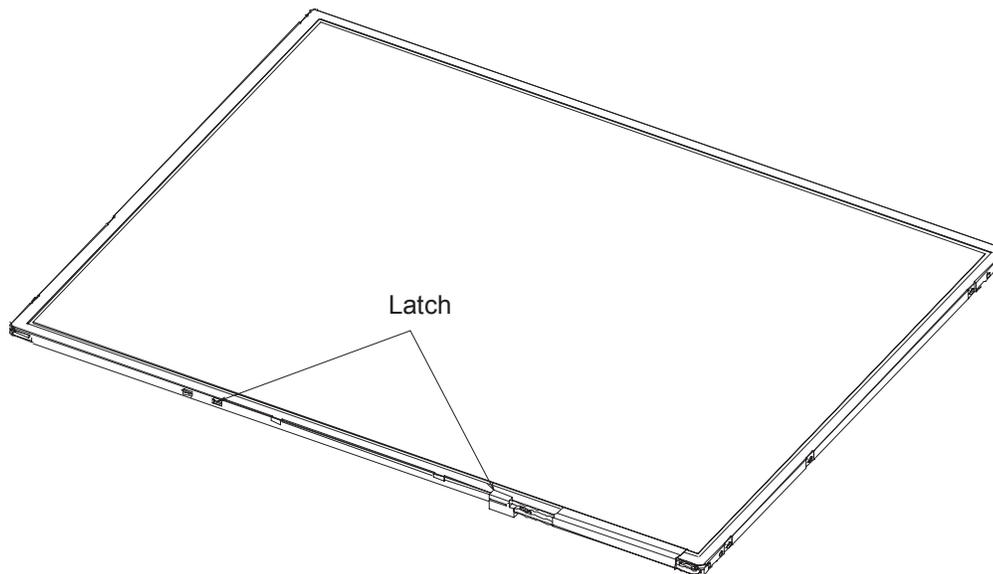
*Figure 4-152 Removing the latches close to the lamp*
