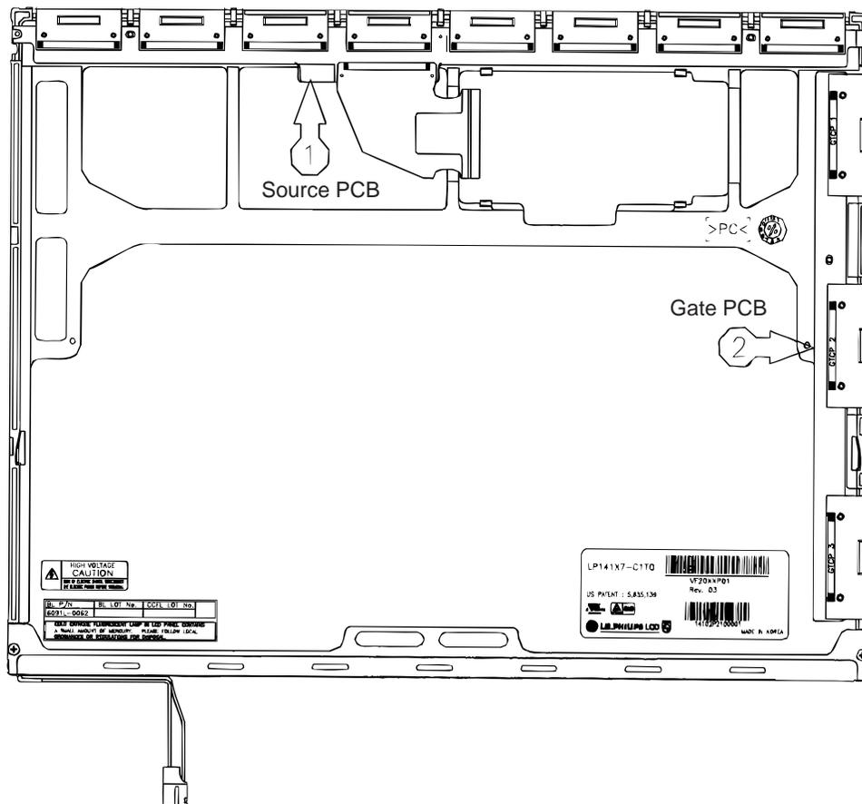
Figure 4-170 Removing the source PCB and gate PCB
