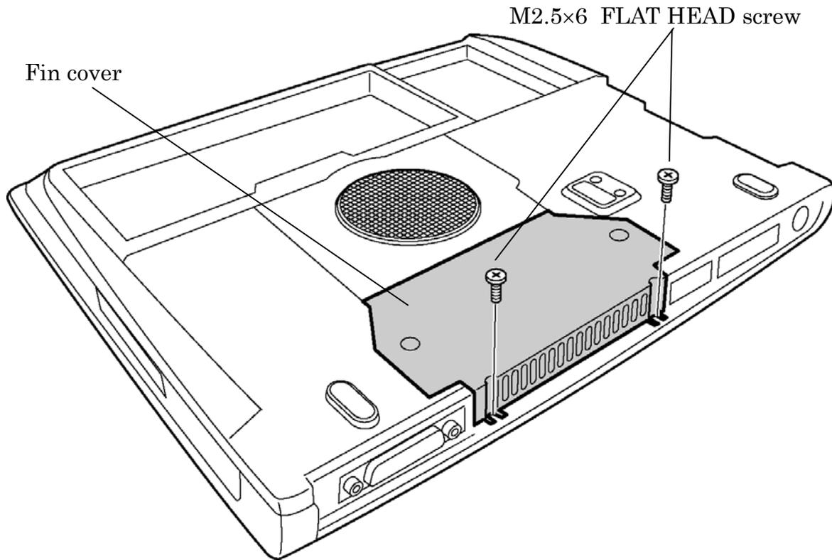
Figure 4-11 Removing the Fin cover
