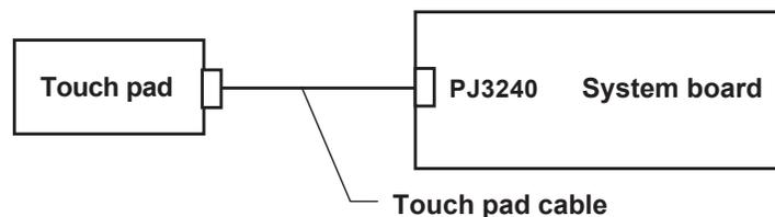
If the connection is loose, reconnect firmly and repeat Procedure 1. If there is still an error, go to Check 4.
