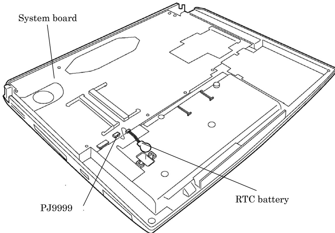
*Figure 4-29 Removing the RTC battery*
