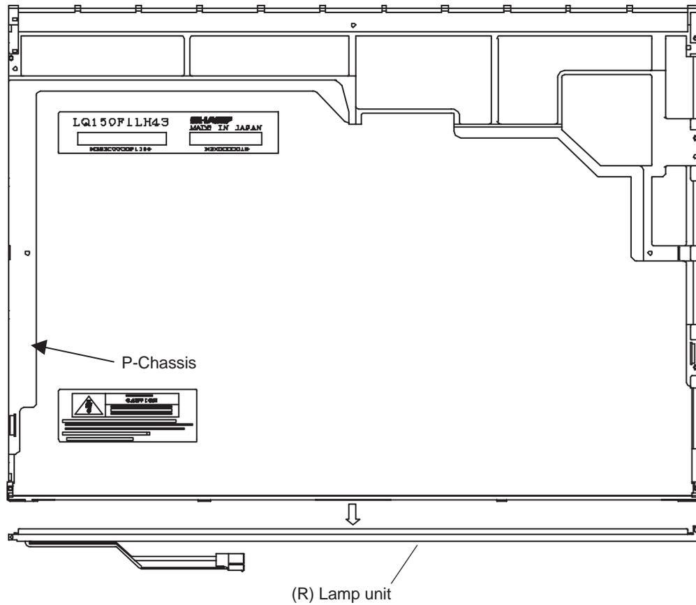
Figure 4-122 Replacing Sharp fluorescent lamp (SXGA+) (10)
