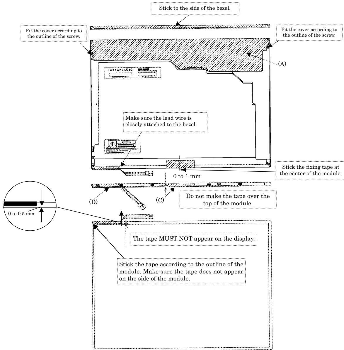
Figure 4-136 Replacing Sharp fluorescent lamp (SXGA+) (24)
