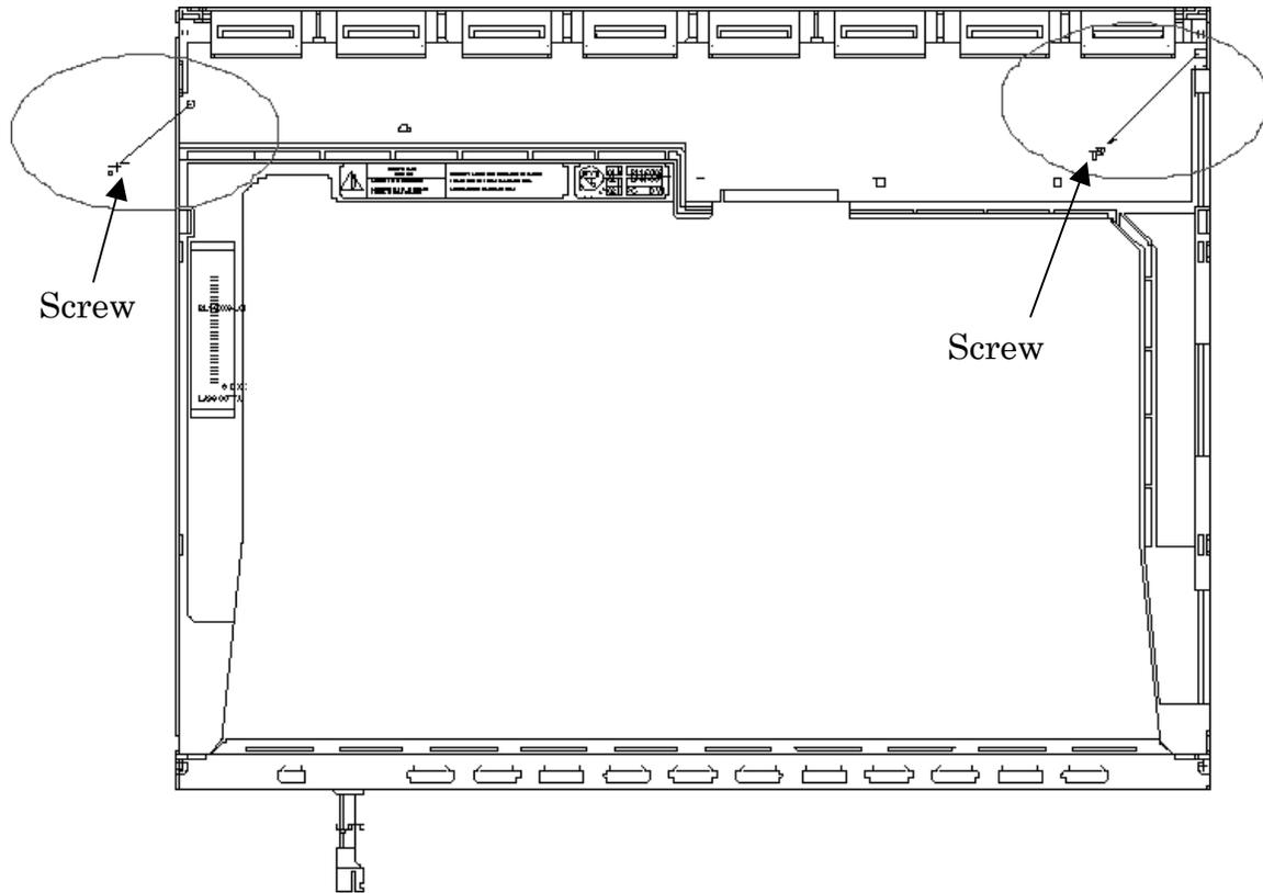
Figure 4-59 Replacing Samsung fluorescent lamp (XGA) (2)
