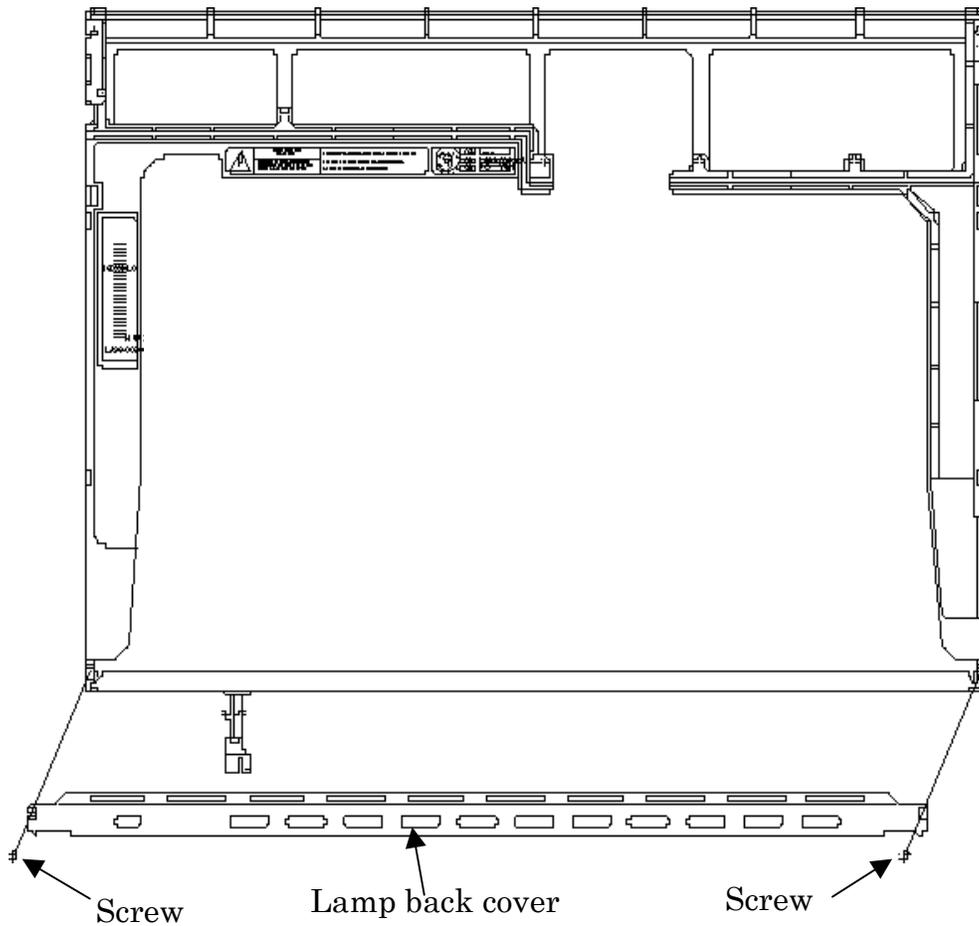
Figure 4-64 Replacing Samsung fluorescent lamp (XGA) (7)
