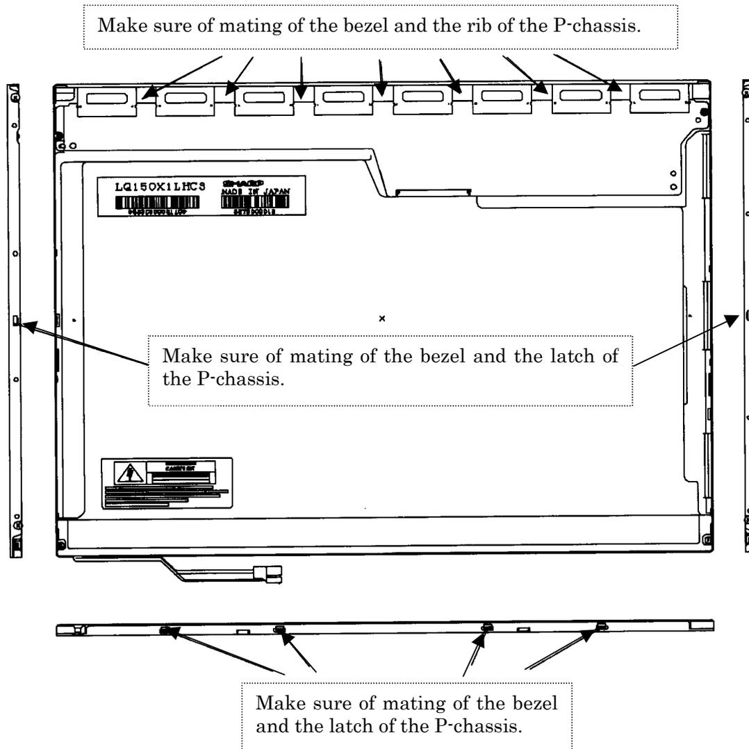
Figure 4-87 Replacing Sharp fluorescent lamp (XGA) (21)
