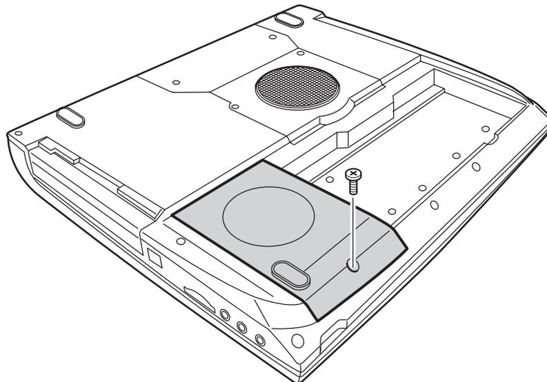
Figure 4-4 Removing the HDD cover
