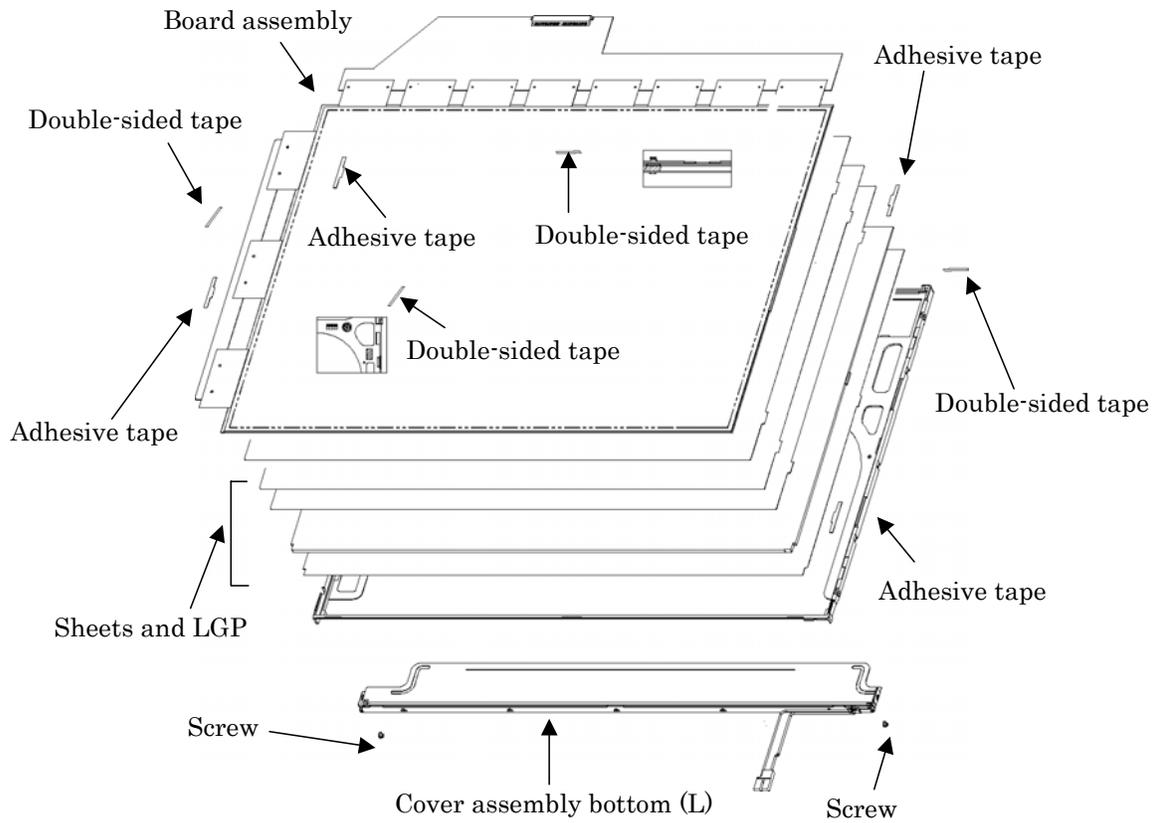
Figure 4-54 Replacing LG.Philips fluorescent lamp (XGA) (5)
