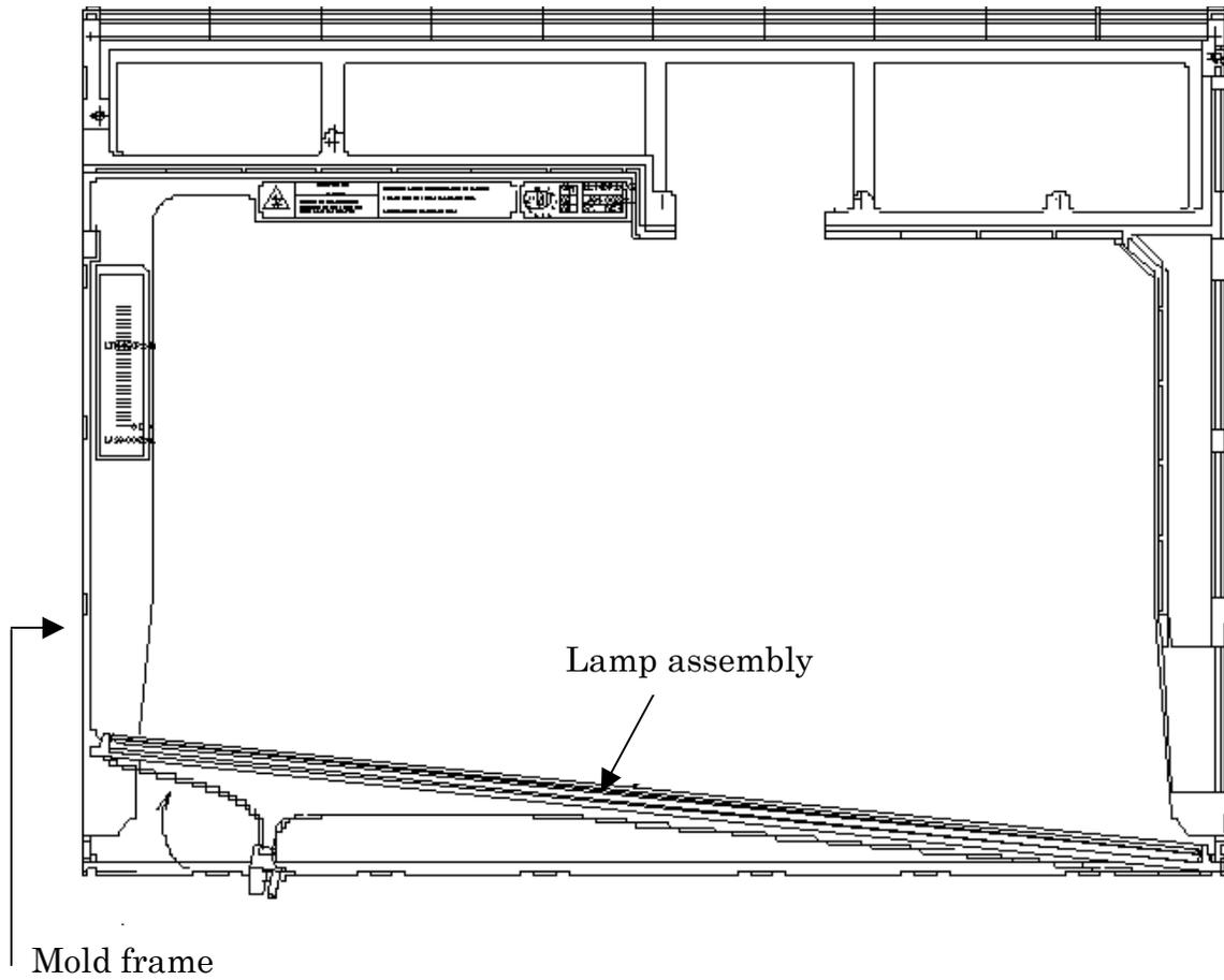
Figure 4-112 Replacing Samsung fluorescent lamp (SXGA+) (9)
