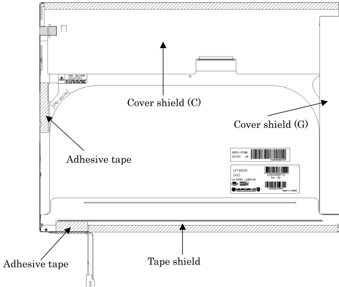
Figure 4-50 Replacing LG.Philips fluorescent lamp (XGA) (1)
