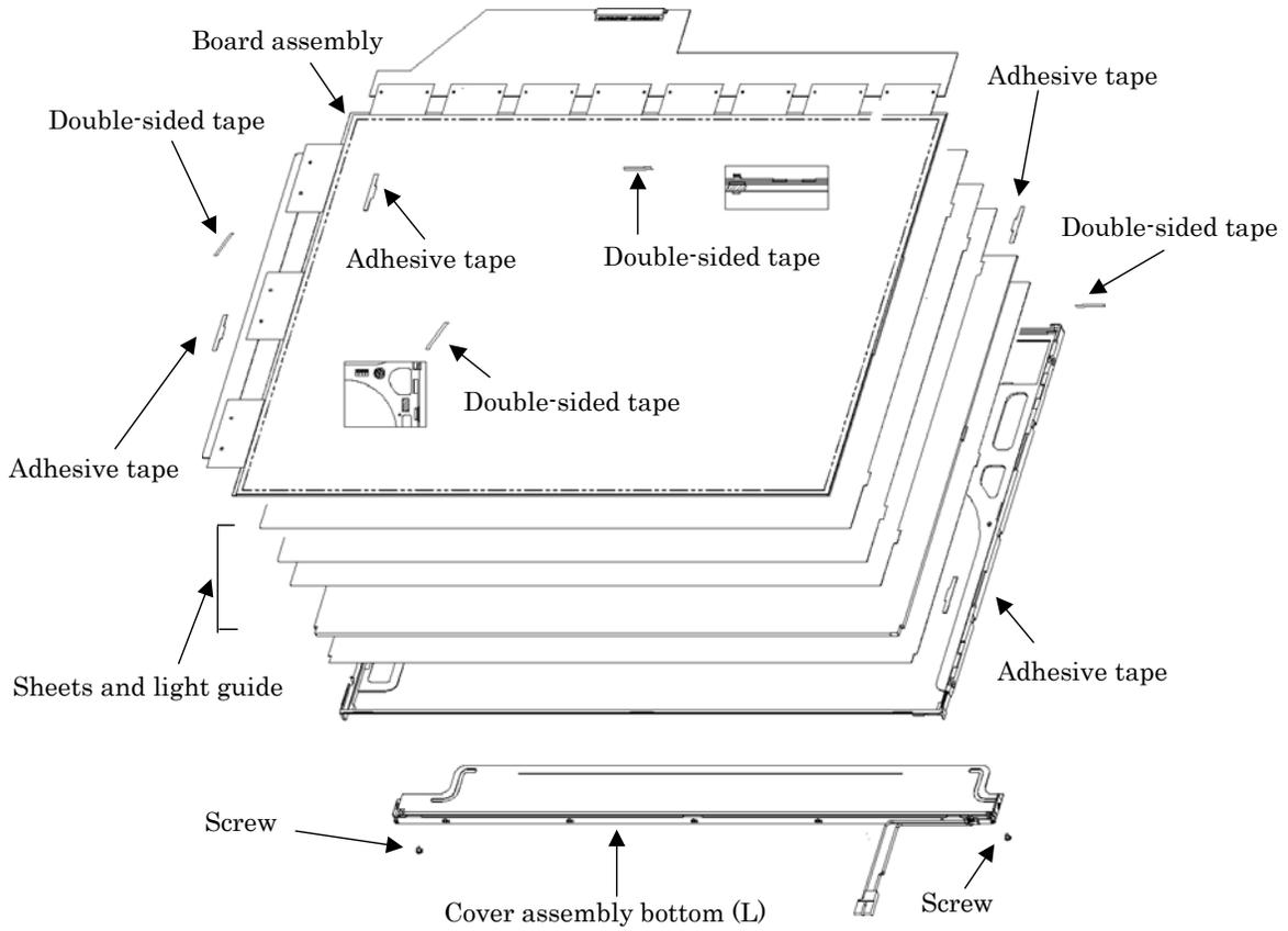
Figure 4-100 Replacing LG.Philips fluorescent lamp (SXGA+) (5)
