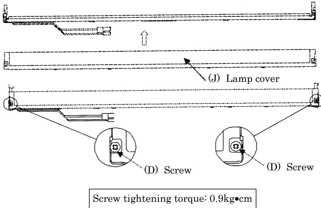
Figure 4-126 Replacing Sharp fluorescent lamp (SXGA+) (14)
