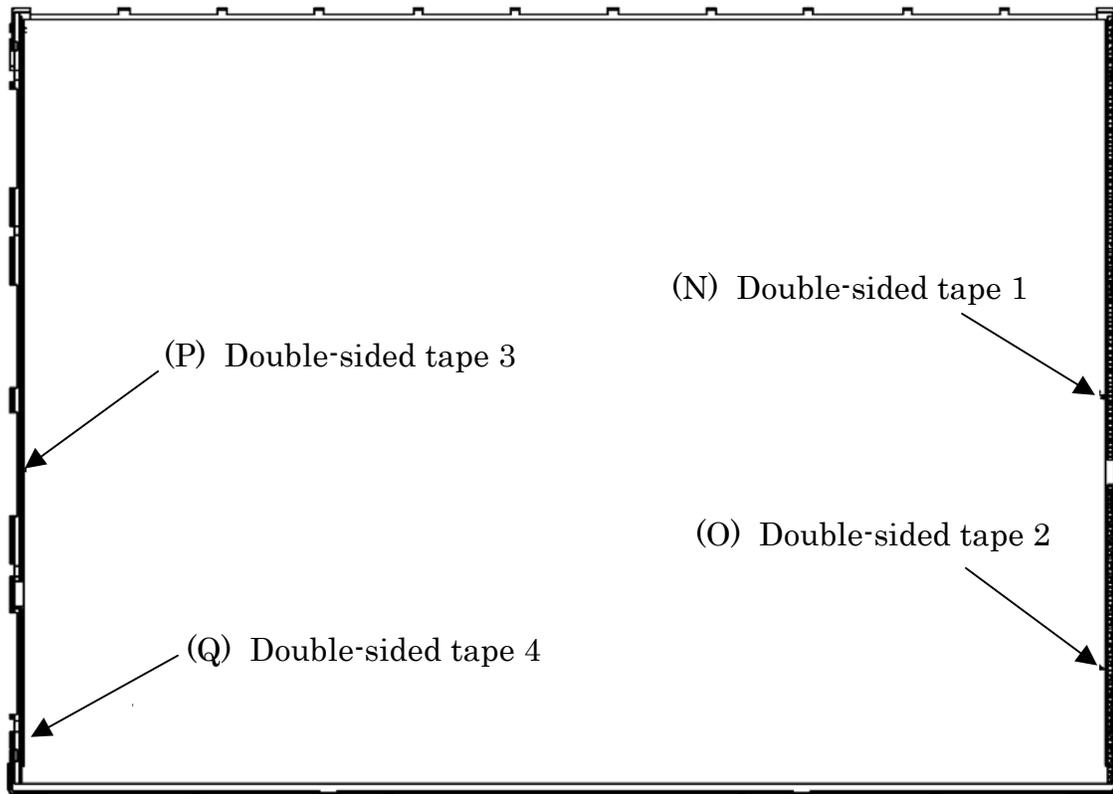
Figure 4-121 Replacing Sharp fluorescent lamp (SXGA+) (9)
