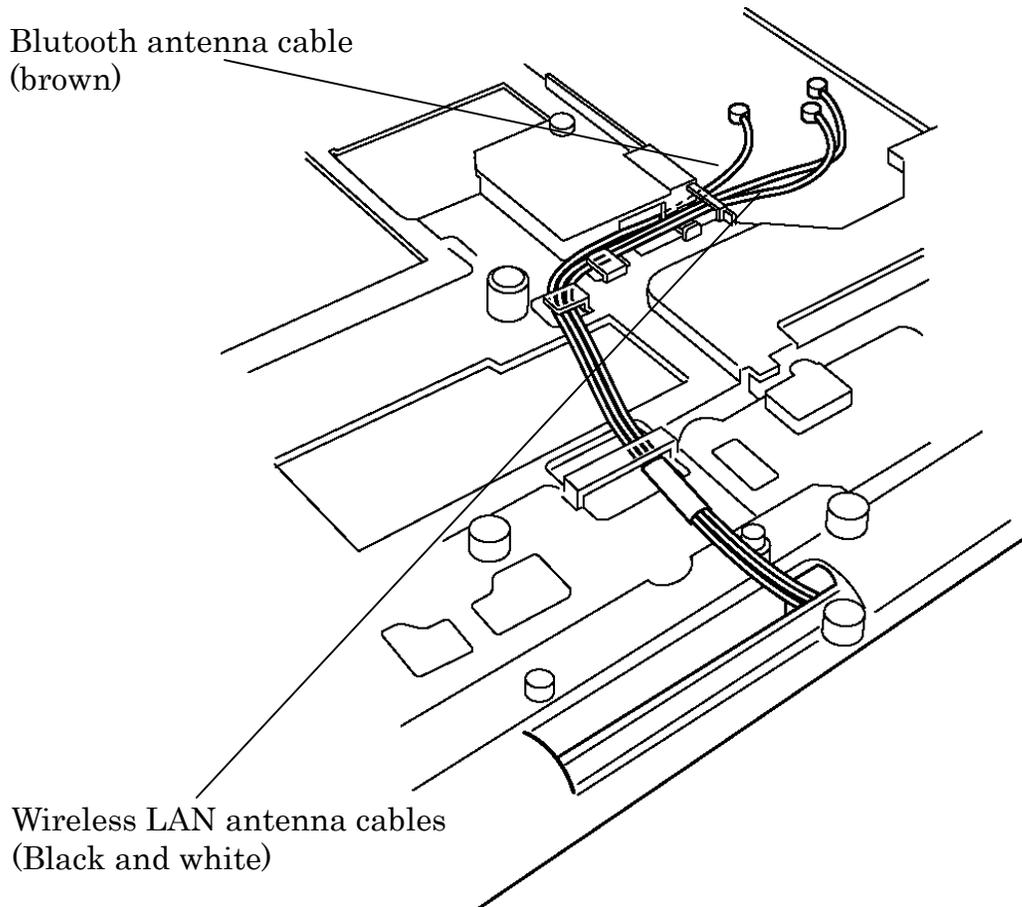
Figure 4-49 Installing the Wireless LAN/Bluetooth antenna cable
