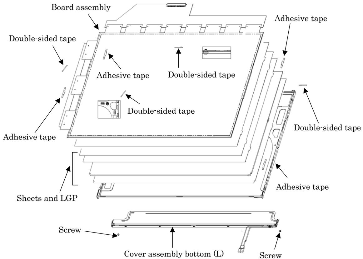
Figure 4-53 Replacing LG.Philips fluorescent lamp (XGA) (4)
