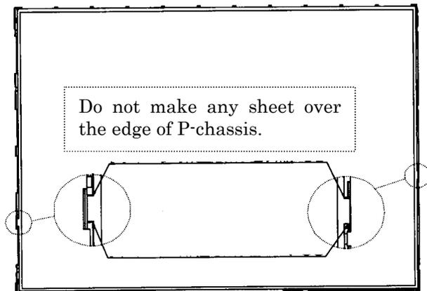
Figure 4-82 Replacing Sharp fluorescent lamp (XGA) (16)
