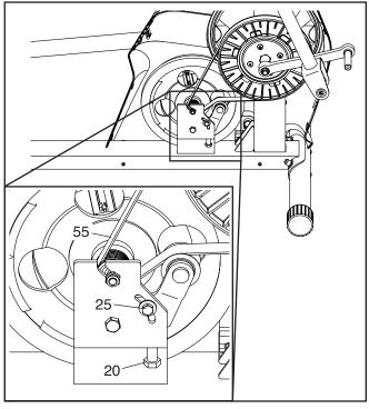
Reattach the right shield, the outer and inner crank covers, the right roller arm, the right pedal arm, and the accessory tray.
