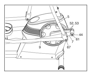
Next, remove the M8 x 20mm Screw (61), the Axle Cover (44), and the M8 Washer (not shown) from the Right Roller Arm (7) and the right Crank Arm (not shown). Gently move the Right Roller Arm out of the way. Then, use a flat screwdriver and gently remove the Outer and Inner Crank Covers (52, 53) from the right Crank Arm.
