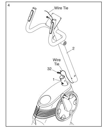
5. **Tip: Avoid pinching the Main Wire Harness** (32). Slide the Upright (2) onto the Frame (1).
