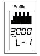
When you select a preset workout, a profile of the resistance levels of the workout will scroll across
