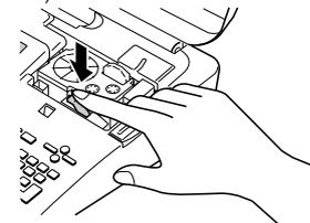
\* Use an object that is at least 30mm (1-3/16") long and no thicker than 1.5mm (1/16"). Do not use a toothpick or other object with an easily breakable tip. Doing so creates the risk of printer malfunction.
