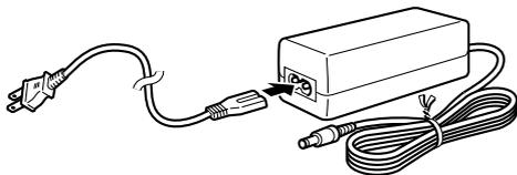
2. Connect the AC adaptor plug to the printer's AC adaptor terminal (①), and then plug the power cord into a household power outlet (②).
