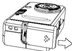
2. Insert the battery pack in the direction of the button marked on the battery pack.
