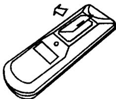
(2) Insert two size AAA batteries according to the polarity indication inside the remote controller.
