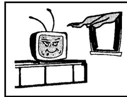
Do not cover the Ventilating holes in the cabinet. Keep a space of more than 5cm from the walls to the TV set, to guarantee the good ventilation.
