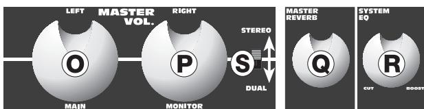
**O & P. MASTER VOLUME LEVEL CONTROLS** – The Left and Right Master Volume Controls adjust the output volume of the PD-250. The Master controls feature notched position indicators. For the majority of applications the Passport system has been balanced to operate with these controls at their notched 12 o'clock positions. In situations where more volume is required the master controls can provide an additional 6 dB of gain when turned to the right of the center position.
