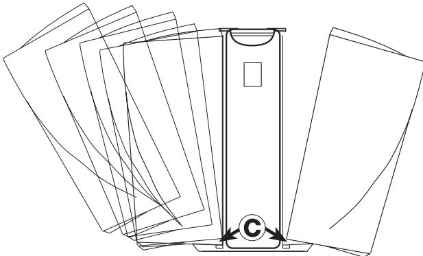
1. Place your finger tip under the safety latch and gently lift. When the safety latch has disengaged, lift the main latch to remove the speaker.
