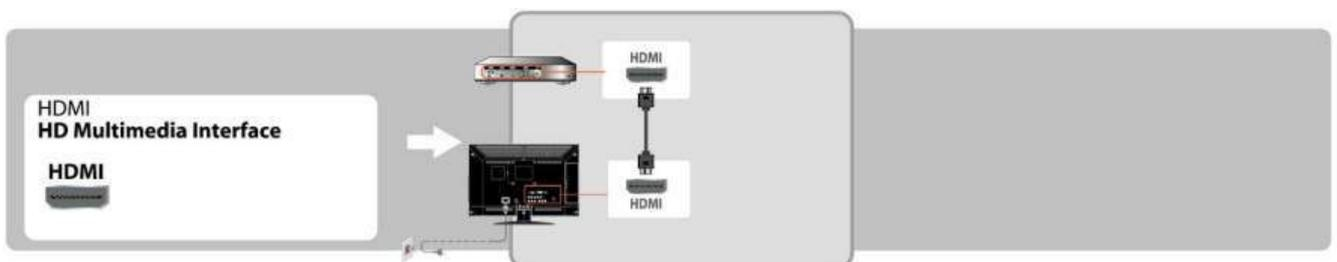
If the equipment has a DVI jack and not an HDMI jack, connect the DVI jack to the HDMI IN (with DVI-to-HDMI cable or adapter) jack and connect the audio jack to the PC AUDIO IN jacks.
