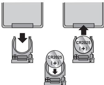
1. Remove the Battery Compartment by pressing in on the tab and then sliding the compartment out.
