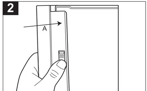
**TO INSERT:** Align tabs from the Battery Pack into the holes in the unit, then slide the Battery Pack in the direction of arrow A.
