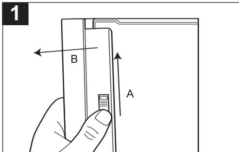
**TO REMOVE:** Slide the Battery Release switch in the direction of arrow A, then slide the Battery Pack in the direction of arrow B.
