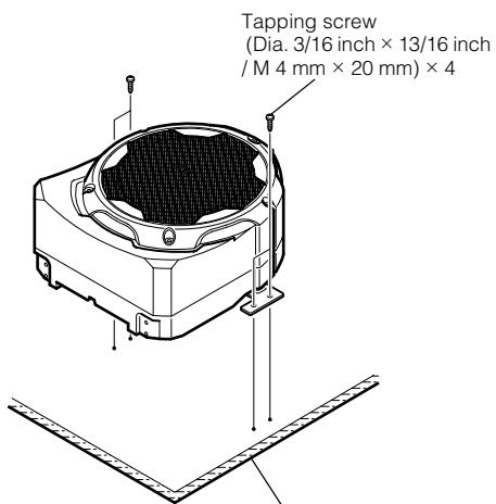
Board (Commercially available item: Thickness 23/32 inch / 18 mm and above)
