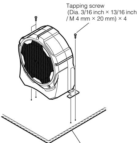
Board (Commercially available item: Thickness 23/32 inch / 18 mm and above)
