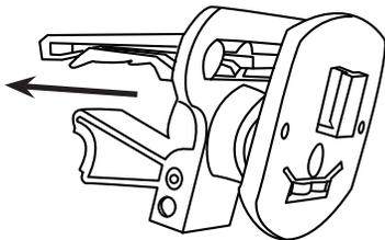
Step 3. Adjust the support leg vertically until it rests firmly along the bottom of the vent or dash surface below the vent. It will need to support the weight of the cradle and device.
