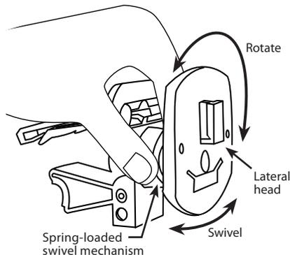
Step 5. While holding the pedestal's swivel mechanism, align the T-tab on the pedestal face to the T-slot on the back of the cradle and slide down.
