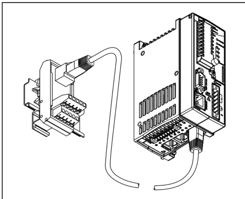
**Figure 3.** Compact FieldPoint DIN Rail-Mountable Terminal Block
