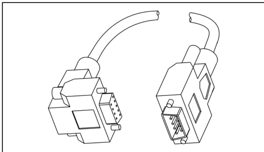
**Figure 1.** Compact FieldPoint DB-9 Cable Adapter for COM 1
