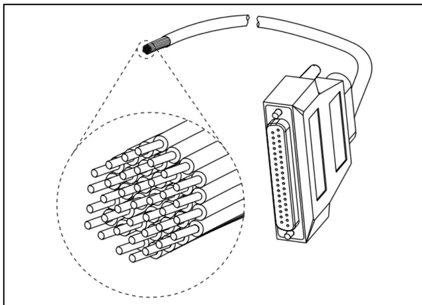
**Figure 6.** Compact FieldPoint 37-Pin I/O Connector Cable
