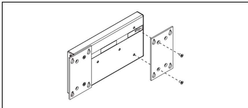
**Figure 9.** Compact FieldPoint Horizontal Panel-Mount Kit with cFP-BP-4
