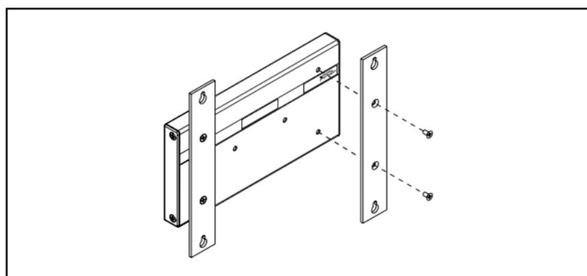
**Figure 12.** Compact FieldPoint Vertical Panel-Mount Kit with cFP-BP-4
