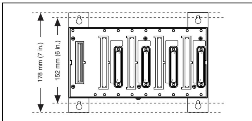
**Figure 13.** Dimensions of Compact FieldPoint Vertical Panel-Mount Kit
