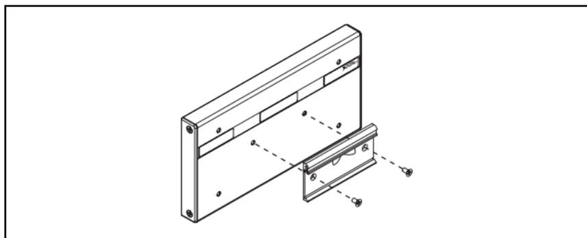
**Figure 8.** Compact FieldPoint DIN Rail Clip with cFP-BP-4
