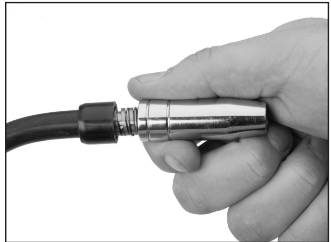
Figure 10. Removing the welding torch nozzle.
