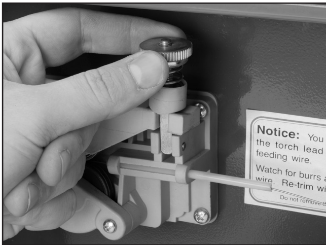
Figure 9. Adjusting the feed tension.
