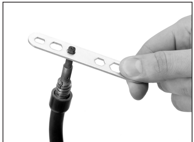
Figure 11. Attaching a new contact tip.
