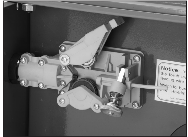
Figure 7. The open wire feed mechanism.
