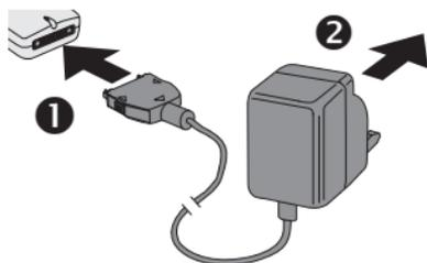
Connect the AC Adaptor to the mains power supply (2). Indicator will light and charging starts.
