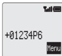
When the call is successful DTMF tones will be sent after 3 seconds or when **↶** is pressed.
