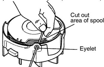
11. Remove line from notch and feed line through eyelet.
