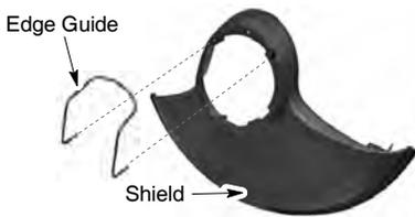
2. Insert the shield onto the motor housing. Ensure the cutting head remains free to rotate and the line is not caught between the shield and the motor housing (see following illustration).
