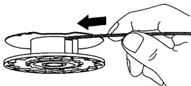
8. Wind the line evenly and tightly onto the spool. Wind in the direction of the arrow found on the spool.
