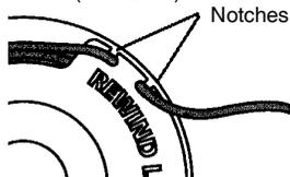
10. Place spool into hub with cut out area of spool in line with eyelet (see illustration).
