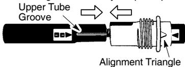
3. Try to pull tubes back apart. If the tubes do not come apart, they are properly snapped into place. If the tubes come apart, repeat step 1 and push until the tubes snap into place.
