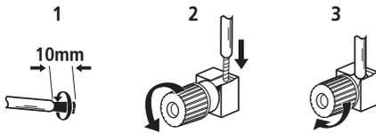
**1 Twist exposed wire strands together.****2 Loosen speaker terminal and insert exposed wire.**
