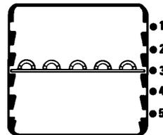
Most second oven cooking should be carried out using the shelf provided in shelf position 2. However, when cooking a small joint or a deep cake you can use the shelf on the base of the second oven to allow enough air to circulate around the food.
