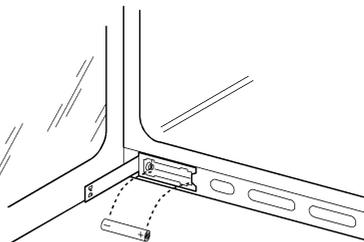
When you fit the new battery, make sure the positive end (marked with a + sign) is next to the (+) sign on the battery holder. Close the lid of the battery holder.
