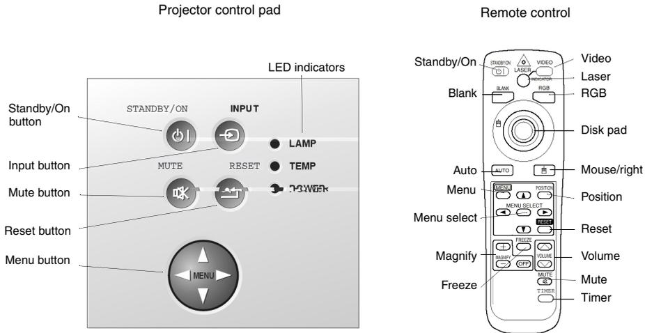
Figure 6: Projector and Remote Controls
