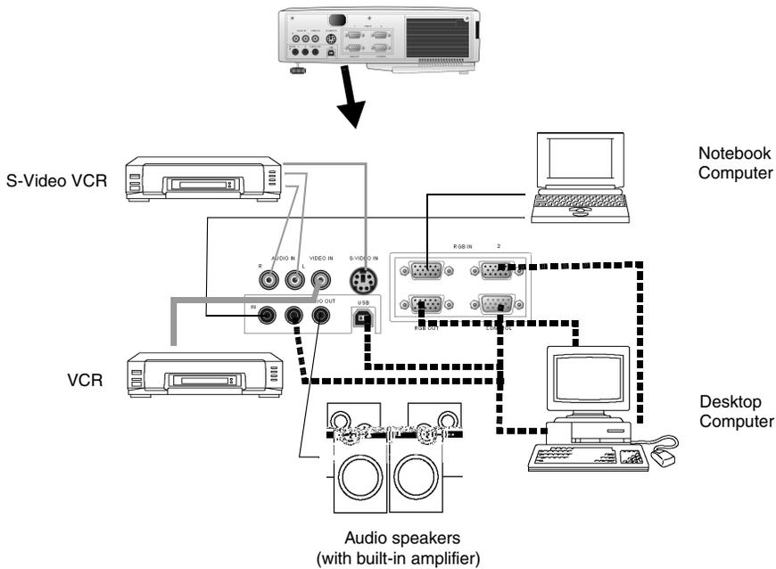
Figure 3: System Setup
