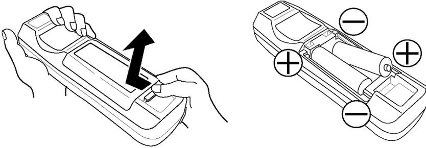
Figure 8: Installing the Batteries
