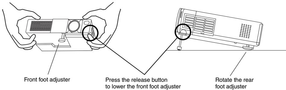
**Figure 5: Angle Adjustment**
