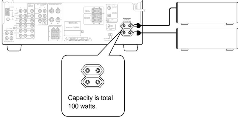
Capacity is total 100 watts.
