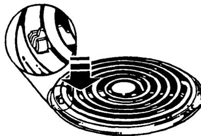
**NOTE:** Reflector bowls reflect heat back to the utensils on the surface units. They also help catch spills. When they are kept clean, they reflect heat better and look new longer.
