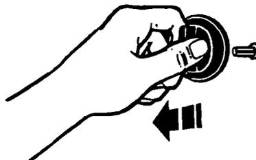
2. Loosen the locking screws inside the control knob. Note the position of the notches.
