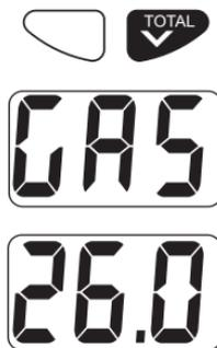
Press and hold both keys for three seconds and the displayed value will begin to flash.
