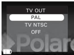
The TV screen performs as the LCD screen and the LCD screen is powered off after a proper connection between the picture viewer and a TV.
