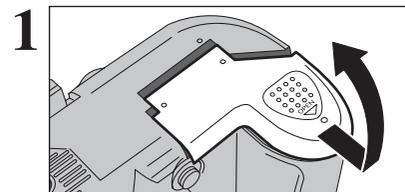
1 Check that the camera is turned off (set the Power switch to "OFF") before opening the battery cover.
