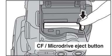
Open the slot cover, press the CF/Microdrive eject button and remove the CF/Microdrive.
