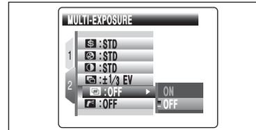
Multiple exposure provides a way of overlaying images on top of each other to give a final image that cannot be got through normal photography.
