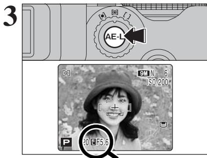
Position the subject in the center of the screen and press the "AE-L" button. "📷" appears on the screen and the exposure is locked while you hold down the "AE-L" button.
