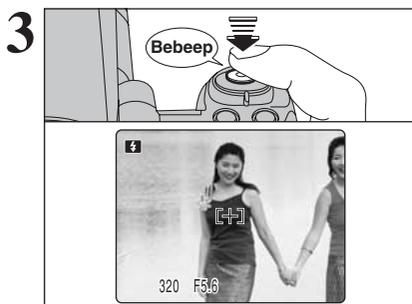
Press the shutter button down halfway (AF/AE lock). When a short double-beep is heard, the camera focuses on your subject. The AF frame on the screen becomes smaller and the camera sets the shutter speed and aperture. The indicator lamp (green) changes from blinking to lit.
