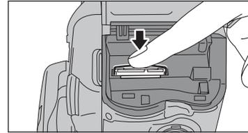
Push the **xD-Picture Card** into the slot and then slowly remove your finger. The lock is released and the **xD-Picture Card** is pushed out.
