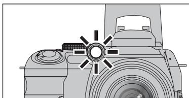
Press the shutter button down halfway in dimly lit conditions. The camera fires the AF-assist illuminator (green) to allow easier focusing. Note that the effective range decreases for telephoto shots.
