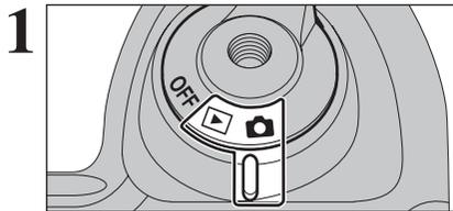
To turn the camera on, set the Power switch to “” or “”.
