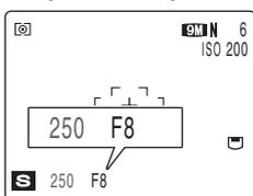
In scenes that are extremely overexposed, the aperture setting (F8) appears in red. When this occurs, select a faster shutter speed (up to 1/4000 sec.).
