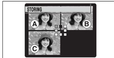
This mode shoots the same image with different exposure settings. Bracketing shoots 3 continuous frames, each with a different exposure setting.
