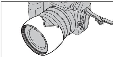
As in storing lens hood into the soft case, the lens hood can be attached upside down.
