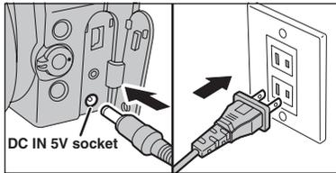
Check that the camera is off. Plug the AC power adapter connector into the "DC IN 5V" socket and then plug the AC power adapter into the power outlet.
