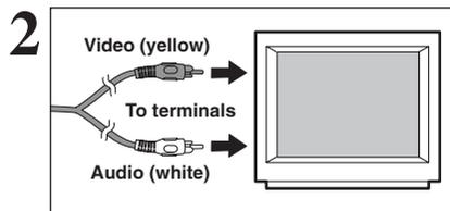
Plug the other end of the cable into the audio / video input socket on the TV. Then turn the camera and TV on and take pictures or play back images normally.
