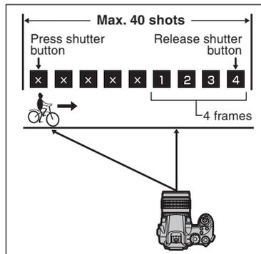
This mode allows you to release the shutter up to 40 times (max. 1.5 frames/sec.) and record the last 4 frames. If you take your finger off the shutter button before 40 shots have been taken, the camera records the final 4 frames shot before you released the shutter button.
