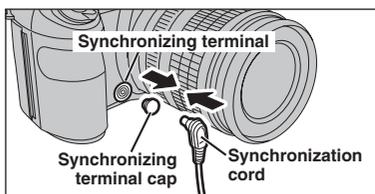
Attach the synchronization cord from the external flash to the Synchronizing terminal on the camera by pushing the cord into the terminal securely.
