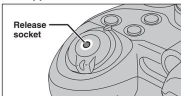
Use a mechanical cable release with this camera. To prevent camera shake, use a tripod (sold separately) and cable release (sold separately).
