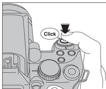
Hold a sheet of white paper so that it fills the entire screen. When pressing the shutter button, the flash fires and the white balance is set.
