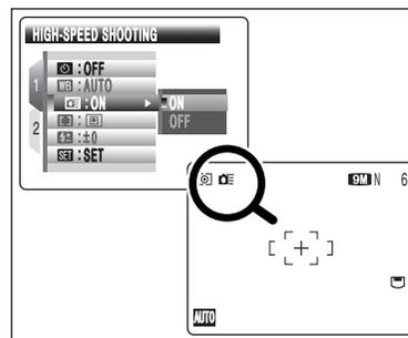
High-speed shooting mode reduces the time required for focusing when pressing the shutter button down halfway.
