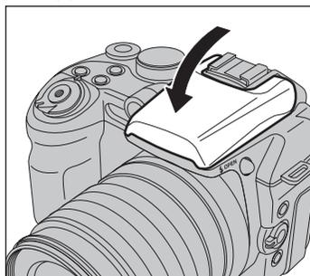
Pressing the flash down changes the camera to Suppressed flash mode.
