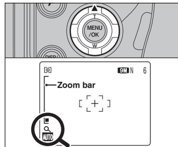
Press "▲" to change to Digital zoom mode (2×). When using digital zoom, "Q" appears in the bottom left corner of the screen and the zoom bar turns blue. Use the zoom ring to adjust digital zoom operation as well as optical zoom. Press the "▼" button to cancel the digital zoom.
