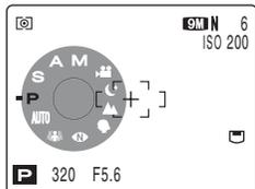
When turning the Mode dial, the Mode dial appears on the screen to check the selected mode. You can operate watching the screen. It is useful such as when taking pictures using viewfinder (EVF).
