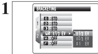
Use this setting to photograph the same image with different exposure settings. Bracketing shoots 3 continuous frames, one of which is correctly exposed while the remaining two are underexposed and overexposed respectively by a set amount.
