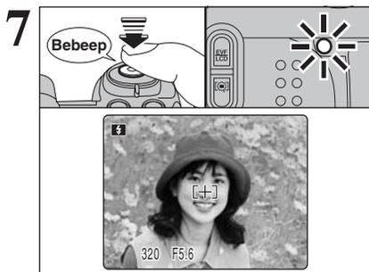
Press the shutter button down halfway. When a short double-beep is heard, the camera focuses on your subject. The AF frame on the screen becomes smaller and the camera sets the shutter speed and aperture. The indicator lamp (green) changes from blinking to lit.
