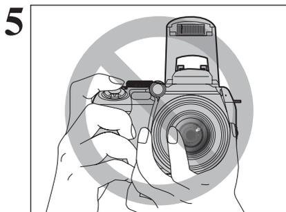
Hold the camera so that your fingers or the strap do not cover the lens, flash and AF-assist illuminator. If the lens, flash or AF-assist illuminator is obscured by your fingers or the strap, subjects may be out of focus or the brightness (exposure) of your shot may be incorrect.
