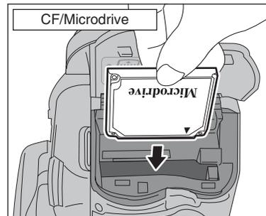
Push the CF/Microdrive firmly all the way into the CF/Microdrive slot. Compatibility is listed on Fujifilm website: <http://home.fujifilm.com/products/digital/>
