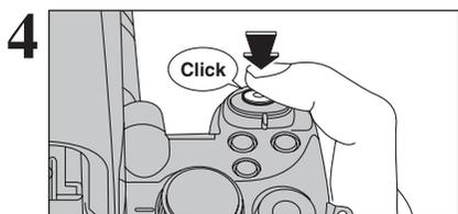
4 Press the shutter button down fully. When a clicking sound is heard, the camera records the image.
