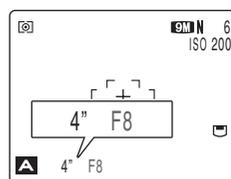
In scenes that are extremely underexposed, the shutter speed setting (4 sec.) appears in red. When this occurs, select a smaller number of aperture.
