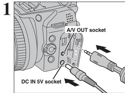
Turn off the camera and TV. Plug the A/V cable (included) into the "A/V OUT" (Audio/Visual output) socket.
