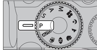
Set the Mode dial to "P". This is an automatic mode to specify the settings except for the shutter speed and aperture setting. This is a simple way to take pictures the same as the Shutter-priority Auto and Aperture-priority Auto modes (Program shift).
