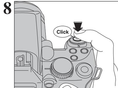
Press the shutter button down fully. When a clicking sound is heard, the camera records the image.
