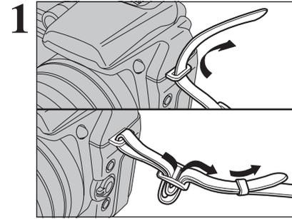
1 Attach the strap to the strap mounts on the camera. Once you have attached both ends of the strap, check carefully to make sure that the strap is firmly secured.
