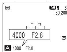
In scenes that are extremely overexposed, the shutter speed setting (1/2000 sec. or 1/4000 sec.) appears in red. When this occurs, select a larger number of aperture (up to F8).
