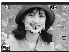
Normal shooting provides an aspect ratio of 4:3 and "3:2" shooting provides an aspect ratio of 3:2 (same aspect ratio as 35 mm film and post card).
