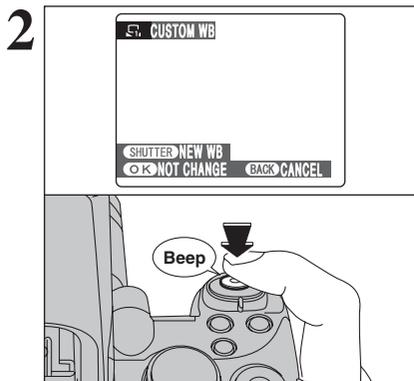
Hold a piece of white paper under the light source for setting the white balance, so that it fills the entire screen. Then press the shutter button to set the white balance.
