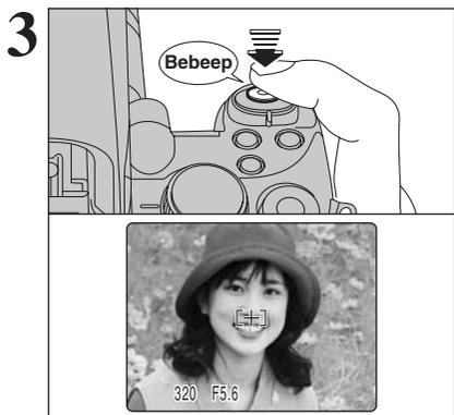
3 Press the shutter button down halfway. When a short double-beep is heard, the camera focuses on your subject. The AF frame on the screen becomes smaller and the camera sets the shutter speed and aperture. The indicator lamp (green) changes from blinking to lit.
