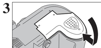
3 Press on the battery cover to push the batteries down. Slide the cover closed.
