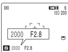
In scenes that are extremely underexposed, the aperture setting (F2.8) appears in red. When this occurs, select a slower shutter speed (down to 4 sec.).
