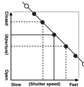
The graph at left shows the way the aperture and shutter speed settings can be changed while maintaining the same exposure level.
