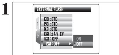
Select "ON" in this setting when using an external flash unit. Synchronized shutter speeds up to 1/1000 sec. can be used.
