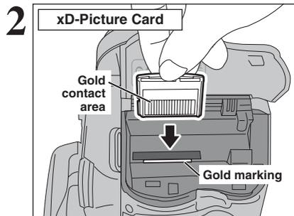
Align the gold marking on the xD-Picture Card slot with the gold contact area on the **xD-Picture Card** and push the card firmly all the way into the slot.
