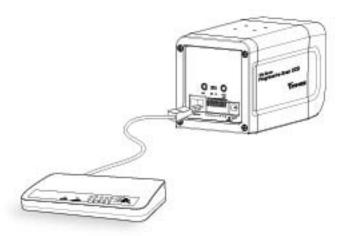
If your switch/router does not support PoE, use a PoE power injector (optional) to connect between the Network Camera and a non-PoE switch/router.
