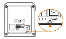
There is an indented reset button on the back panel of the Network Camera. It is used to reboot the Network Camera or restore the Network Camera to factory default. Sometimes rebooting the Network Camera sets the Network Camera back to normal state. If the problems remain after rebooting, restore the factory default and install again.
