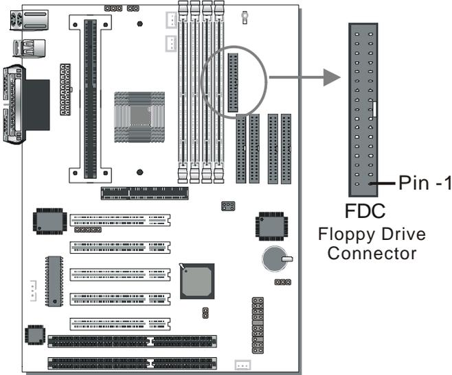
The system supports 5 possible floppy drive types: 720 KB, 1.2 MB, 1.44 MB, 2.88 MB, and LS-120. In addition, this Motherboard supports a 3-mode (720 KB/ 1.2 MB/ 1.44 MB) floppy commonly used in Japan. Connect one side of the 34-pin flat cable to the floppy drive and plug the other end to the floppy drive connector on the Motherboard. This Motherboard can support up to 2 floppy drives.
