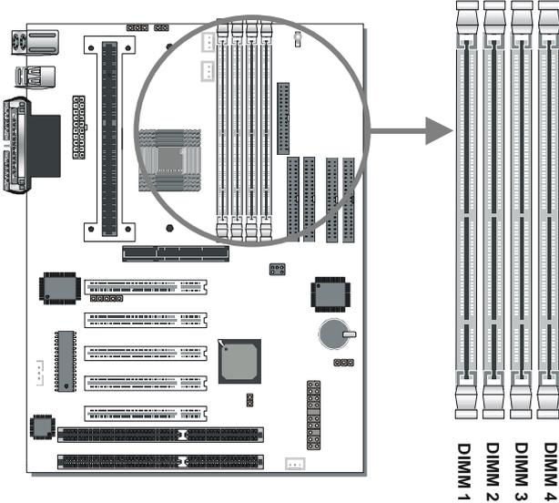
Your board comes with four DIMM sockets, providing support for up to 512 Mbytes or 1 GB (with registered DIMMs). For 66MHz front side bus CPUs use 12ns or faster memory; for 100MHz front side bus CPUs use 8ns (100MHz, PC100 compliant) memory.
