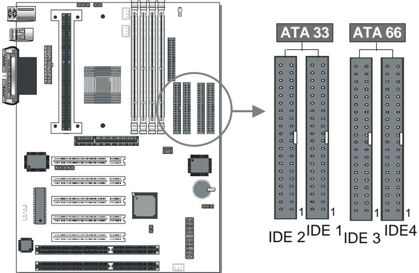
Connect one side of the ATA 33 or ATA 66 flat cable to the IDE device (HDD or CD ROM) and plug the other end to the IDE1~IDE4 directionally keyed IDE connector on the Motherboard. ATA66 cable can be used backward compatible with ATA33 HDD.
