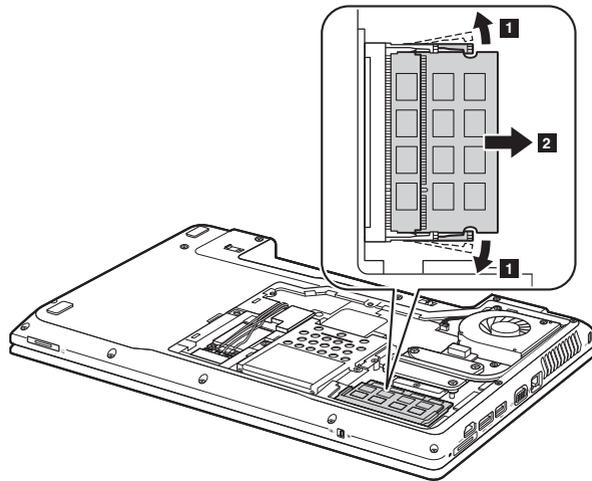
**Note:** If only one DIMM is used on the computer you are servicing, the card must be installed in SLOT-0 ( **a** : lower slot), but not in SLOT-1 ( **b** : upper slot).
