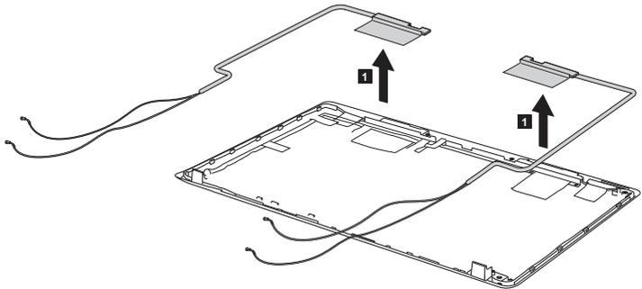
**When installing:** Route the antenna cables along the cable guides and secure the antenna boards with adhesive tapes. As you route the cables, make sure that they are not subjected to any tension. Tension could cause the cables to be damaged by the cable guides, or a wire to be broken.
