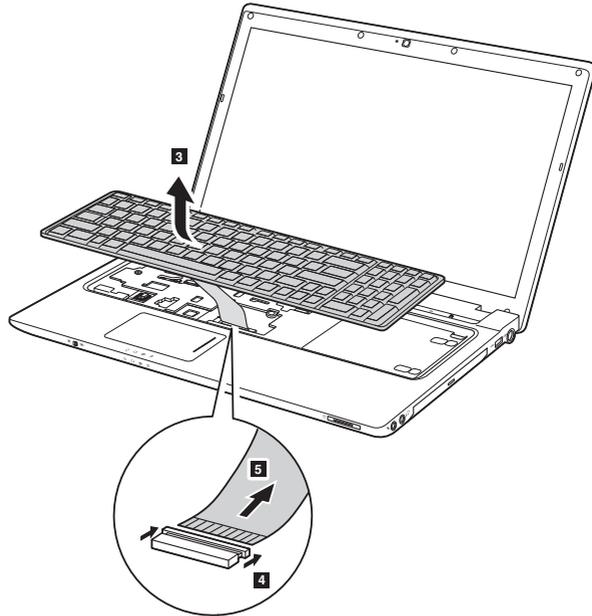
**When installing:** Make sure that the FPC connector is attached firmly and then lock the FPC connector.
