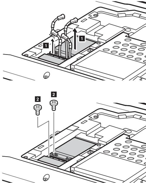
Disconnect the two wireless LAN cables (black, white) and the two wireless WAN cables (red, blue) in the direction shown by arrows **1**, and then remove the screws **2**.
