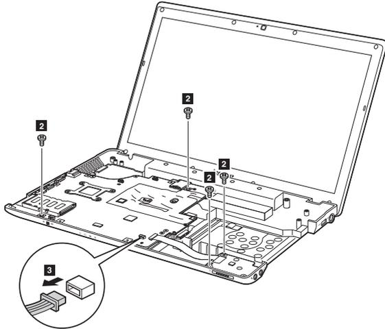
**When installing:** Make sure that the connector is attached firmly.
