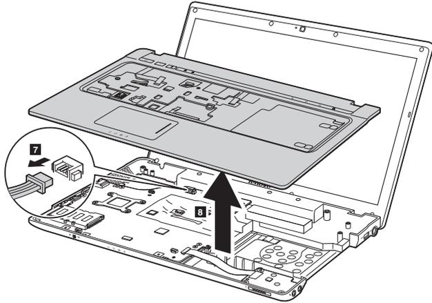
**When installing:** Make sure that the speaker connector is attached firmly.
