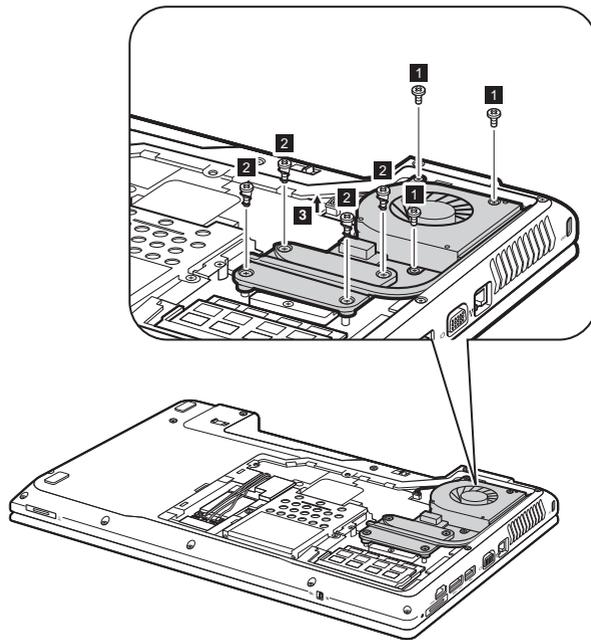
**When installing:** Make sure that the fan connector is attached firmly to the system board.
