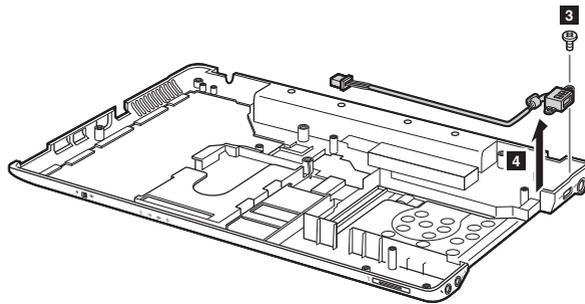
**When installing:** Make sure that the USB connector is attached firmly.
