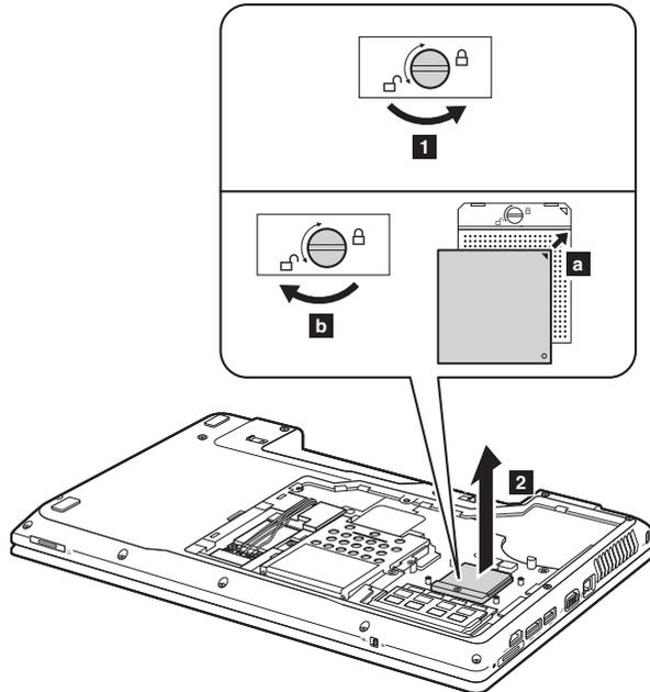
**When installing:** Place the CPU on the CPU socket in the direction shown by arrow **a**, and then rotate the head of the screw in the direction shown by arrow **b** to secure the CPU.
