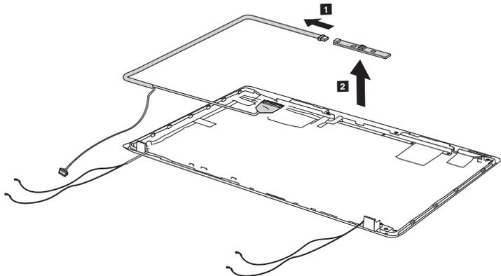
**When installing:** Stick the integrated camera to the top center of the LCD cover and adjust the placement of it to make sure the connector is attached firmly. When replacing the integrated camera, route the connector cable as shown in the figure above.
