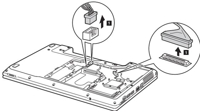
**When installing:** Make sure that the connectors are attached firmly.
