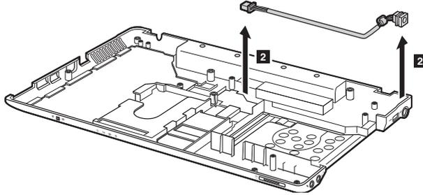
**When installing:** Make sure that the power connector is attached firmly.
