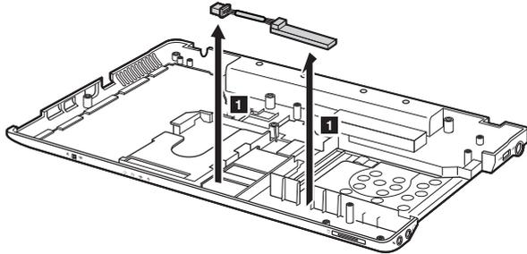
**When installing:** Make sure that the connector is attached firmly.
