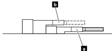
**When installing:** Insert the notched end of the DIMM into the socket. Push the DIMM firmly, and pivot it until it snaps into the place. Make sure that it is firmly fixed in the slot and difficult to be moved.
