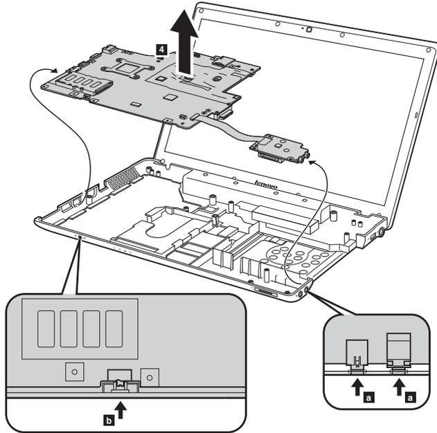
**When installing:** When attaching the system board to the base cover, adjust the placement of the wireless radio switch as shown in **b**, and make sure that both of the audio jack and the microphone jack are attached to the holes on the base cover as shown in **a**. Improper placement of the switch or those jacks might cause a damage.
