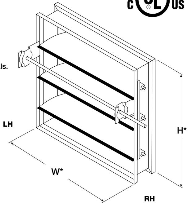
\*W&H dimensions furnished approximately ¼ in. (6mm) undersize. (Add sleeve thickness for overall sleeved damper dimension)
