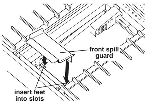
**C.** Insert the front spill guard feet into the slots in the rear spill guard as shown. The rear flange will rest on the burner box.
