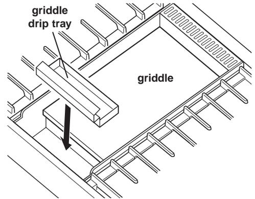
**A.** Place drip tray in the well at the front of the griddle. Slide tray forward until it stops.
