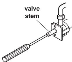
**B.** **Adjusting the surface burner or grille flame:** Note: there is no adjustment for the griddle flame. Gas flow is at 100%, temperature is controlled by thermostat.
