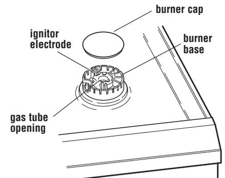
**13.** Put burner caps on each burner base. Place burner grates over burner bases and caps.
