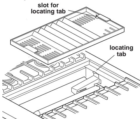
**G.** Install the wave tray into the grille/griddle bay. The tab in the left rear corner of the bay **must** fit through the slot in the left rear corner of the wave tray.
