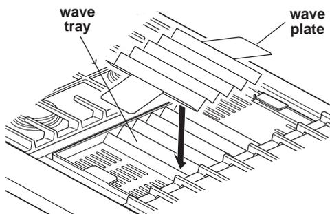
**H.** Place the wave plate on the wave tray as shown. The wave plate **must** be centered on the wave tray.
