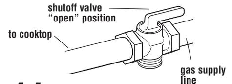
**11.** Open shutoff valve in the gas supply line. Wait a few minutes for gas to move through the gas line.
