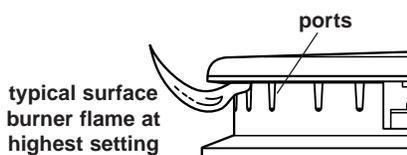
**C.** Check flame on “HI” for a blue color. It should be clean and soft in character. No yellow tip, blowing or lifting of flame should occur. Occasional orange flashes are normal and reflect different elements in the air or gas.
