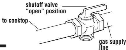
**F.** The supply line shall be equipped with an approved shutoff valve. This valve should be located in the same room as the cooktop and should be in a location that allows ease of opening and closing. Do Not block access to the shutoff valve. The valve is for turning on or shutting off gas to the appliance.
