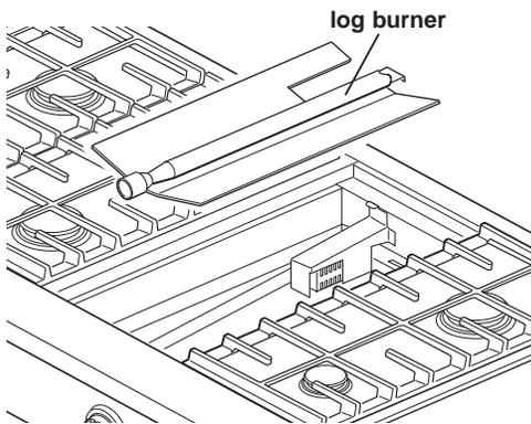
**A.** Lift the log burner up out of the bay and set aside.
