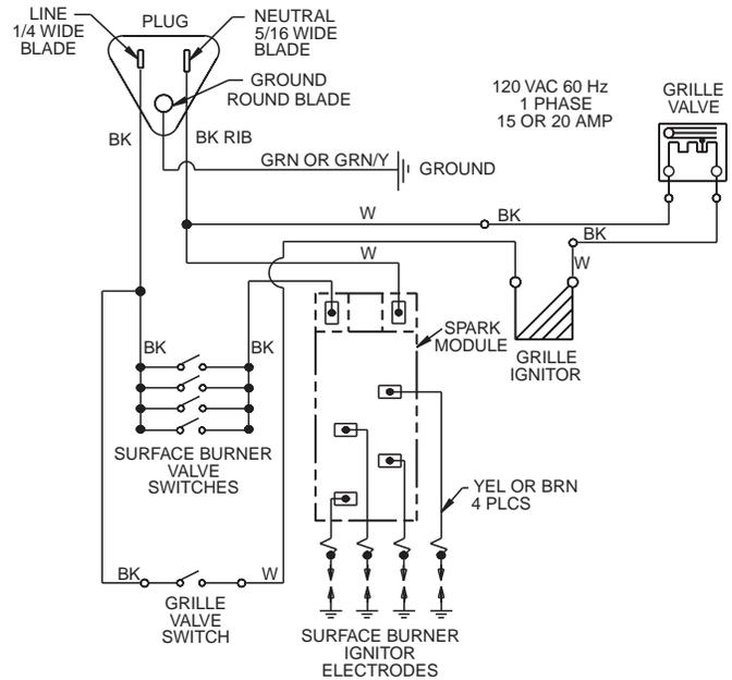
SWITCHES ON SURFACE BURNER VALVES:
