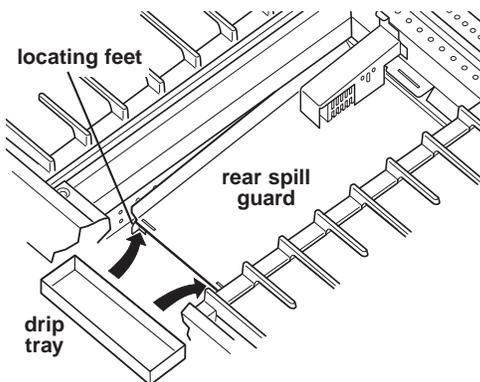
**B.** Place drip tray on bottom of grille bay and slide the tray forward so that it is located side-to-side and against the locating feet of the rear spill guard.
