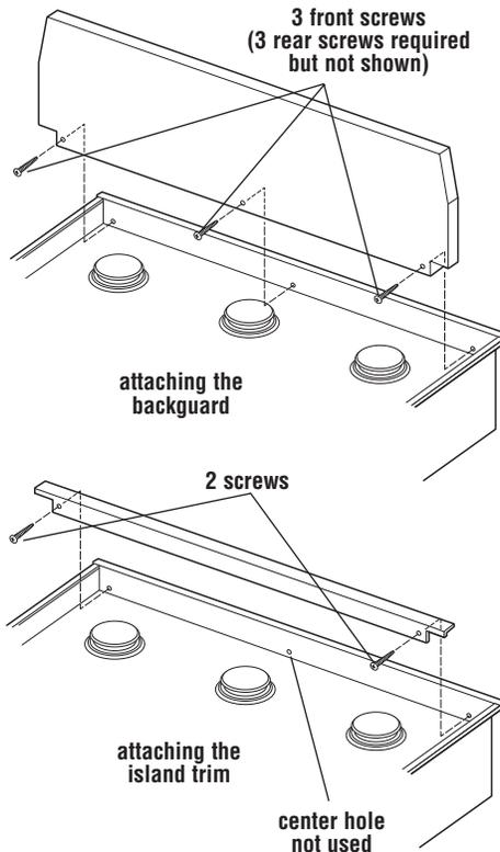
**6.** Attach the backguard or island trim as required for your installation. Attachment screws are in the literature package.
