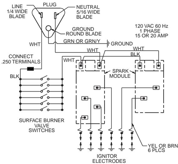
SWITCHES ON SURFACE BURNER VALVES:
