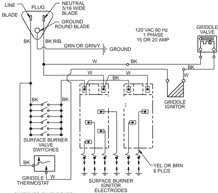
SWITCHES ON SURFACE BURNER VALVES:
