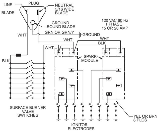
SWITCHES ON SURFACE BURNER VALVES:
