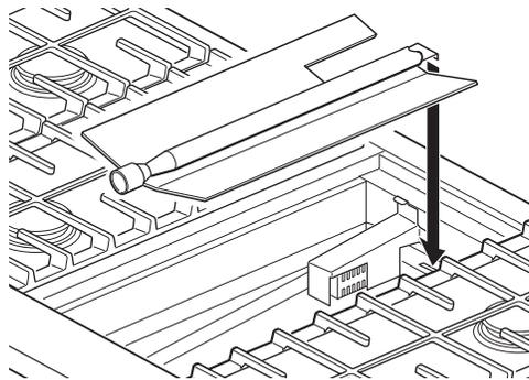
**D.** Reinstall the log burner. Make sure burner's rear flange is seated in slot.
