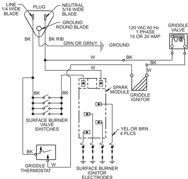
SWITCHES ON SURFACE BURNER VALVES:
