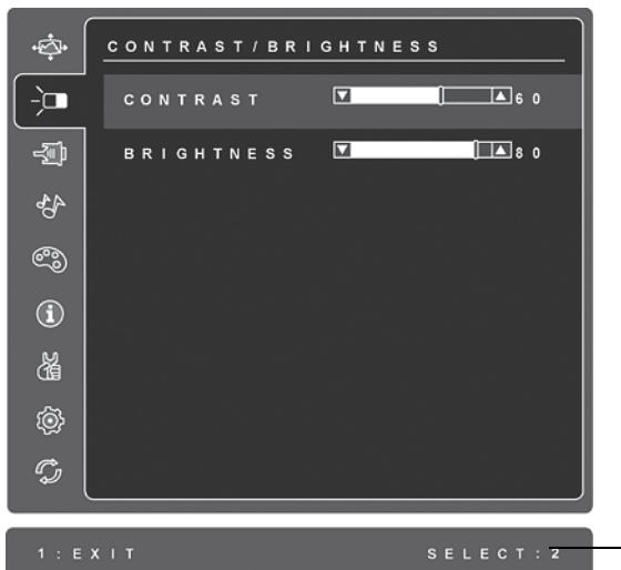
The line at the bottom of the screen shows the current functions of buttons 1 and 2: Exit or select the control.
