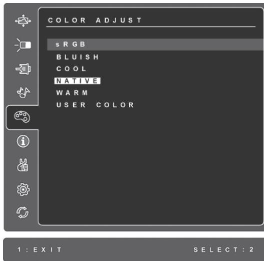
**sRGB**-This is quickly becoming the industry standard for color management, with support being included in many of the latest applications. Enabling this setting allows the LCD display to more accurately display colors the way they were originally intended. Enabling the sRGB setting will cause the Contrast and Brightness adjustments to be disabled.
