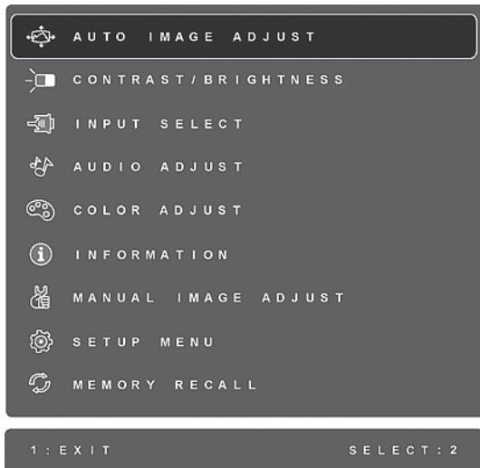
**NOTE:** All OSD menus and adjustment screens disappear automatically after about 15 seconds. This is adjustable through the OSD timeout setting in the setup menu.
