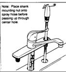
1 Pass spray hose down through hole in escutcheon and extreme right sink deck hole and up through center sink deck hole. Attach spray
