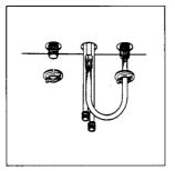
3 Thread mounting nuts onto shanks. FINGER tighten securely.
