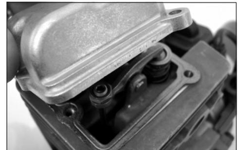
6. Turn engine over several times, and return to TDC-compression. Recheck with proper feeler gauge to make sure clearance adjustment did not change as a result of tightening locknut. Readjust as necessary.
