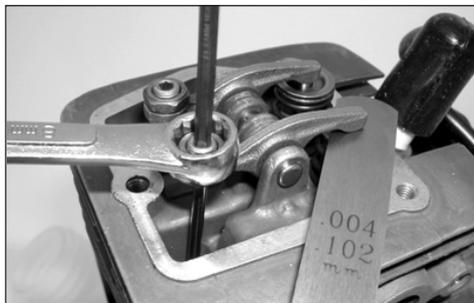
3. Insert feeler gauge (.004" for both intake and exhaust) between valve stem tip and rocker arm.
