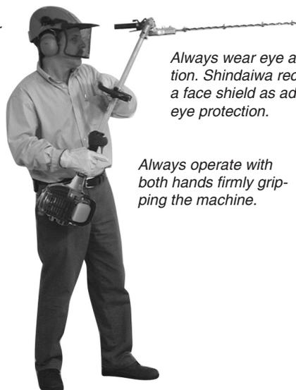
*Always wear eye and hearing protection. Shindaiwa recommends wearing a face shield as additional face and eye protection.*
