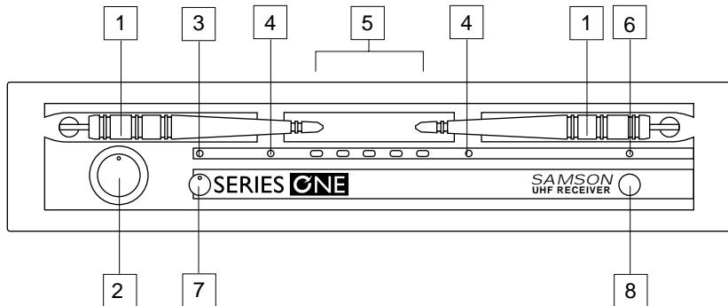
**1: Antennas (A and B)** - The antenna mountings allow full rotation for optimum placement. In normal operation, both Antenna A (the antenna on the left) and Antenna B (the antenna on the right) should be placed in a vertical position. Both antennas can be folded inward for convenience when transporting the UR1. See the “Setting Up and Using the Series One System” section on page 8 in this manual for more information about antenna installation and positioning.
