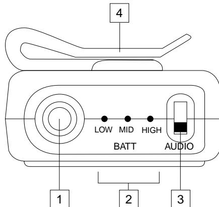
**1: Input connector** - The input device is connected here. The UT1L is supplied with either a lavalier or headset microphone (connected via a Switchcraft mini-XLR jack), while the UT1G is supplied with a permanently connected 1/4" jack cable.
