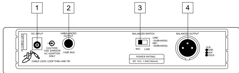
**1: DC input** - Connect the supplied 12 volt 160 mA power adapter here, using the strain relief as shown in the illustration below. **WARNING:** Do not substitute any other kind of power adapter; doing so can cause severe damage to the UR1 and will void your warranty.
