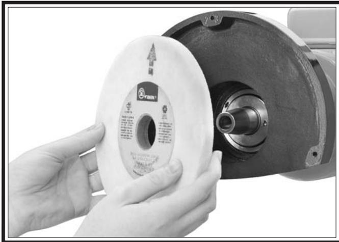
**Figure 17. Removing wheel.**
