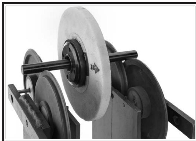
**Figure 33. Wheel on balancing fixture.**
