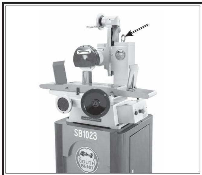
**Figure 5. Lifting location.**
