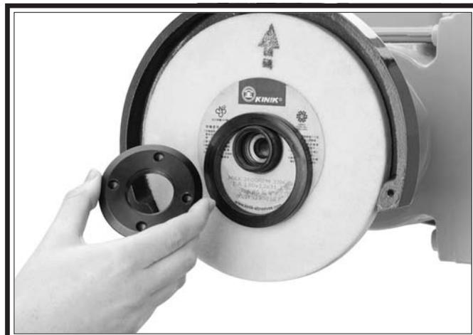
Figure 16. Exposing wheel spacer washer.
