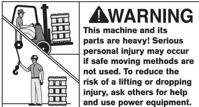
Unbolt the machine from the pallet and make sure that the table is locked in place. Connect a chain or lifting strap to the lifting hook on the machine (**Figure 5**), use a hoist or forklift to lift the machine off the pallet, and move it to the suitable location. All hoisting equipment and straps must be rated to lift at least 1500 lbs.
