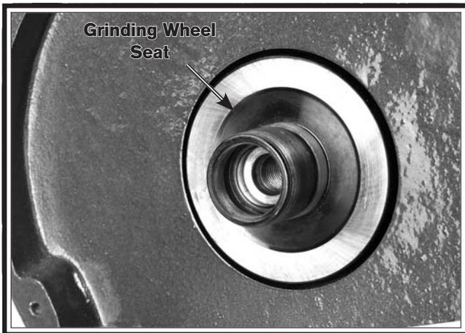
**Figure 18. Wheel mounting hub.**
